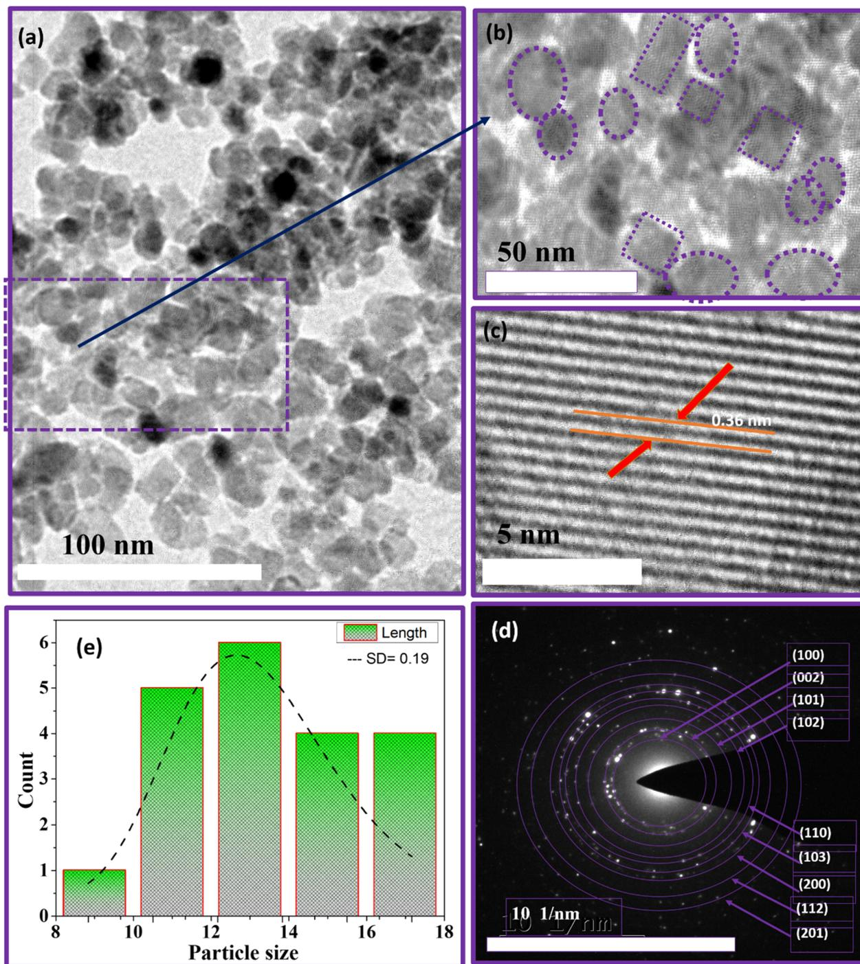
Fig. 6 TEM and HRTEM analysis of *J. adhatoda*-mediated ZnO NPs: (a) low-magnification TEM image showing particle morphology, (b) high-magnification TEM highlighting particle shapes, (c) HRTEM displaying lattice fringes with 0.36 nm spacing, (d) SAED pattern showing indexed diffraction rings, and (e) particle size distribution histogram.
