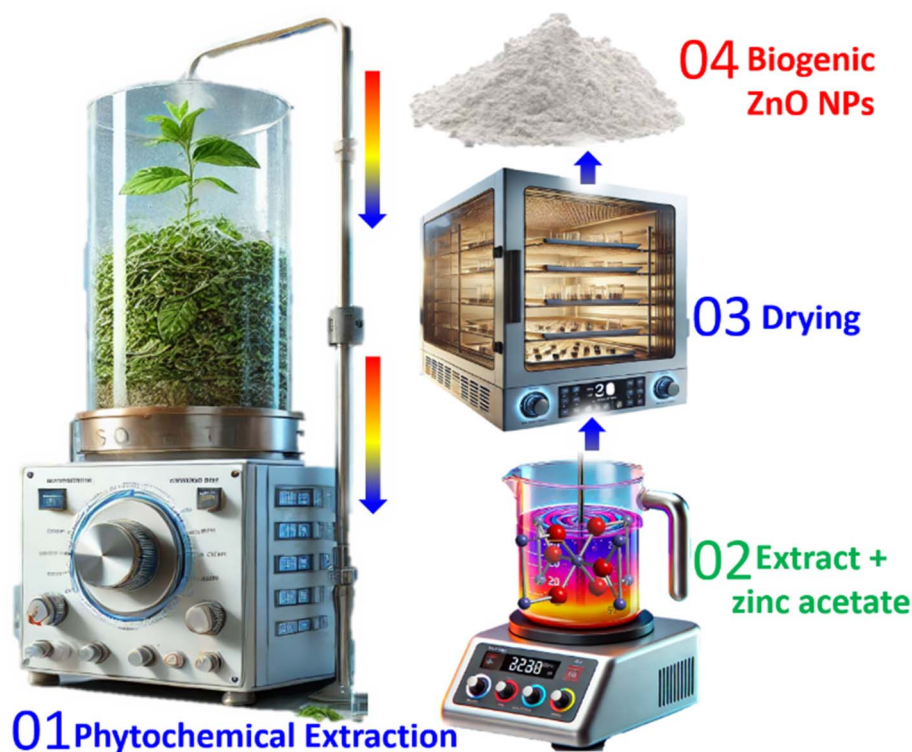
Fig. 1 Stepwise process of green synthesis of ZnO NPs mediated by J. adhatoda extract.
