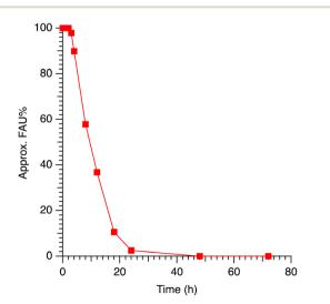
Fig. 2 Mass percent of FAU present as a function of reaction time estimated by powder X-ray diffraction for syntheses performed with a *trans* isomer content of 14%.
