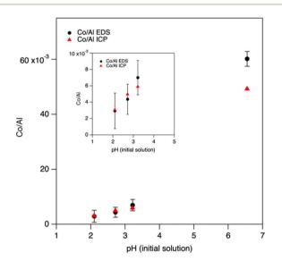
Fig. 13 (Top) Co/Al ratio of a SSZ-39 material made with 20% trans isomer as a function of the initial pH of the cobalt nitrate exchange solution. (Inset) magnification of the plot over pH range of one to five.
