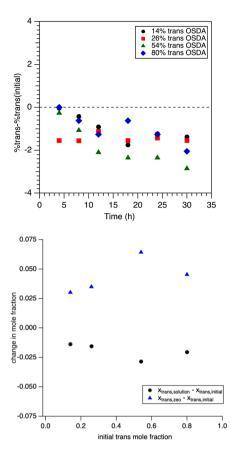
Fig. 7 (Top) change of the *trans* mole percent of OSDA in solution for various *trans* content of OSDA as a function of time. (Bottom) plot of the change in *trans* mole fraction for the OSDA in solution (black circle) and occluded in the final product after synthesis (blue diamond).
