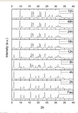
Fig. 1 PXRD results as a function of the heating time (14% trans content of OSDA).
