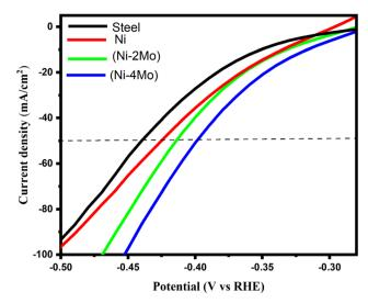
Fig. 4 Polarization curves of the hydrogen evolution reaction on the deposited electrocatalytic materials in mol  $\rm L^{-1}$   $\rm H_2SO_4$  at 298 K. The potential scan rate is 50 mV s<sup>-1</sup>.
