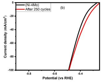
Fig. 7 LSV for (a) Ni–2Mo fresh and after 250 cycles; (b) Ni–4Mo fresh and after 250 cycles. The curves are collected in 0.5 mol  $L^{-1}$  H<sub>2</sub>SO<sub>4</sub> at 25 °C with a scan rate of 50 mV s<sup>-1</sup>.
