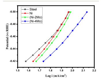
Fig. 5 Tafel plots of hydrogen evolution reaction on the deposited electrocatalytic materials in mol L<sup>-1</sup> M H<sub>2</sub>SO<sub>4</sub> at 298 K.
