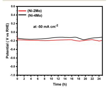
Fig. 6 The chronopotentiometric curves for HER on the surface of Ni-2Mo and Ni-4Mo catalysts at a current density of -50 mA cm<sup>-2</sup>.
