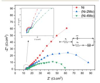
Fig. 8 Measured (dots) and fitted (solid lines) Nyquist plots for Ni, (Ni–2Mo), and (Ni–4 Mo) coatings in 0.5 mol L $^{-1}$  H $_2$ SO $_4$ . Insets: The equivalent circuit for EIS fitting; the locally enlarged plots for showing semicircles.
