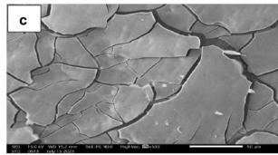
Fig. 1 SEM micrographs of electrodeposited Ni (a), Ni-2Mo (b), and Ni-4Mo (c) alloys
