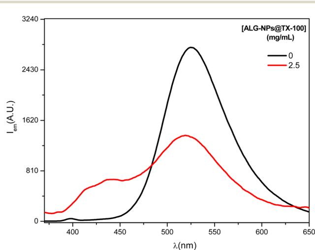
Fig. 3 The emission spectra of PRODAN in pure water and, in ALG-NPs prepared in TX-100 RMs at  $W_0 = 5$ . [ALG-NPs] =  $2.5 \text{ mg mL}^{-1}$ , [PRODAN] =  $3 \times 10^{-6}$  M,  $\lambda_{\text{exc}} = 351$  nm.
