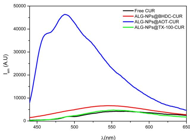
Fig. 4 The emission spectra of curcumin using ALG-NPs synthesized in AOT, BHDC, and TX-100 RMs at  $W_0 = 5$ . [ALG-NPs] =  $1.6 \text{ mg mL}^{-1}$ , [curcumin] =  $3.5 \times 10^{-5}$  M,  $\lambda_{\text{exc}} = 423$  nm.
