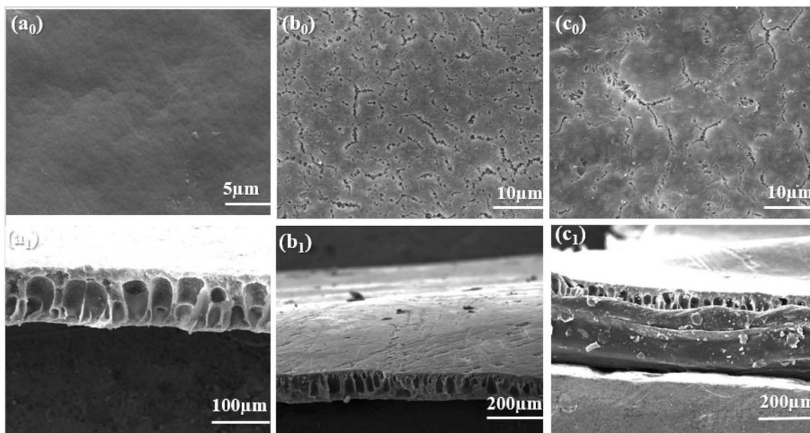
Fig. 6 SEM images of the upper surface and cross-section of membranes: ( $a_0$  and  $a_1$ ) PVDF membrane; ( $b_0$  and  $b_1$ )  $\text{Al}_2\text{O}_3/\text{PVDF}$  (powder)-1.0; ( $c_0$  and  $c_1$ )  $\text{Al}_2\text{O}_3/\text{PVDF}$  (sol)-20%.
