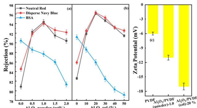
Fig. 11 Effect of the content on filtration performance of Al<sub>2</sub>O<sub>3</sub>/PVDF membranes ((a): Al<sub>2</sub>O<sub>3</sub> powder; (b): Al<sub>2</sub>O<sub>3</sub> sol) and zeta potential (c).
