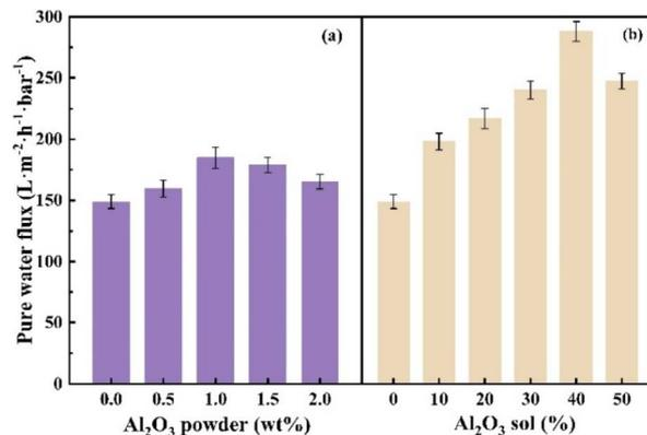
Fig. 10 Effect of content on pure water flux of Al<sub>2</sub>O<sub>3</sub>/PVDF membranes ((a): Al<sub>2</sub>O<sub>3</sub> powder; (b): Al<sub>2</sub>O<sub>3</sub> sol).
