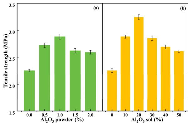
Fig. 8 Effect of Al<sub>2</sub>O<sub>3</sub> content on the mechanical strength of Al<sub>2</sub>O<sub>3</sub>/PVDF membranes ((a): Al<sub>2</sub>O<sub>3</sub> powder; (b): Al<sub>2</sub>O<sub>3</sub> sol).
