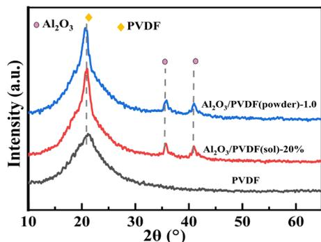
Fig. 5 XRD patterns of PVDF pristine membrane and modified membranes by sol and powder.
