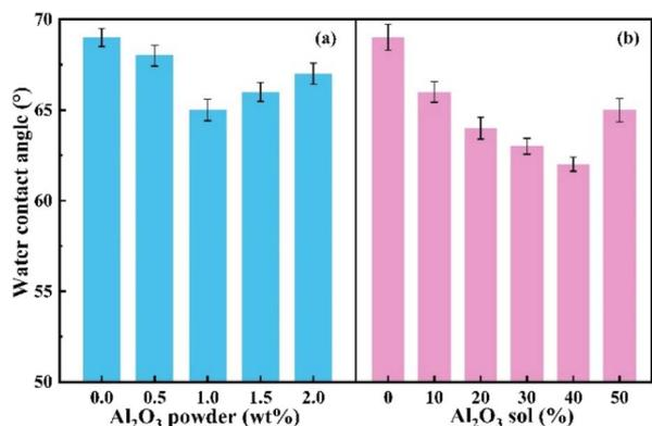
Fig. 9 Effect of Al<sub>2</sub>O<sub>3</sub> content on the contact angle of Al<sub>2</sub>O<sub>3</sub>/PVDF membranes ((a): Al<sub>2</sub>O<sub>3</sub> powder; (b): Al<sub>2</sub>O<sub>3</sub> sol).
