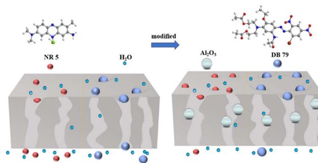
Fig. 12 Schematic of membrane filtration of dyes.
