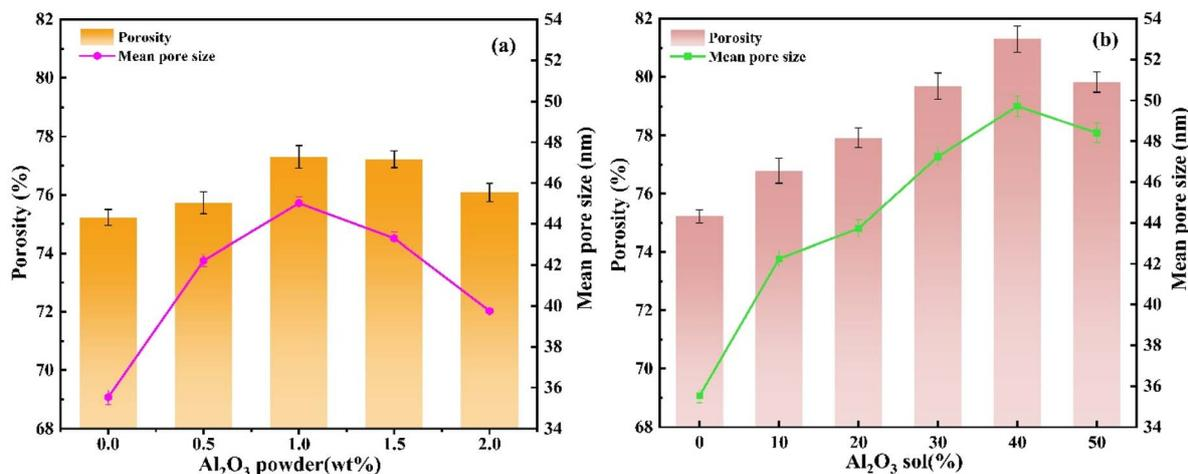
Fig. 7 Effect of the  $\text{Al}_2\text{O}_3$  content on porosity and average pore size of  $\text{Al}_2\text{O}_3$ /PVDF membranes ((a):  $\text{Al}_2\text{O}_3$  powder; (b):  $\text{Al}_2\text{O}_3$  sol).
