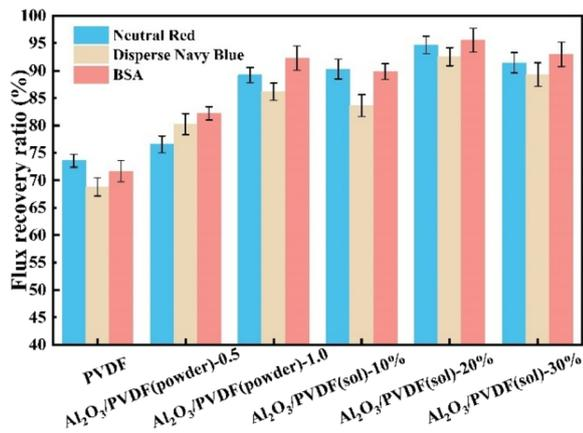
Fig. 13 Effectiveness of different types of Al<sub>2</sub>O<sub>3</sub>/PVDF membrane flux recovery testing.
