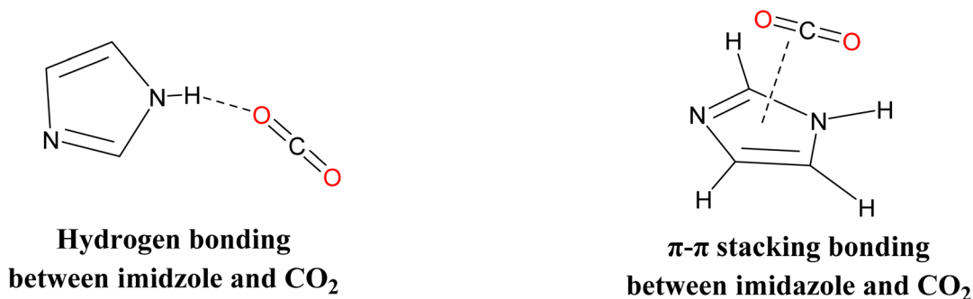
Fig. 2 Different types of interaction for CO 2 adsorption by imidazole.
