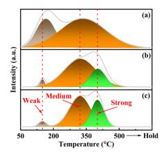
Fig. 8  $\rm NH_3\text{-}TPD$  profiles of the catalysts, (a) VPO, (b) VPOC<sub>6</sub>, (c) VPOC<sub>5</sub>.
