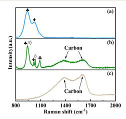
Fig. 2 Raman spectra of the catalysts, (a) VPO, (b) VPOC<sub>6</sub>, (c) VPOC<sub>5</sub>.  $\spadesuit$ - $\delta$ -VOPO<sub>4</sub>,  $\spadesuit$ -(VO)<sub>2</sub>P<sub>2</sub>O<sub>7</sub>,  $\diamondsuit$ - $\gamma$ -VOPO<sub>4</sub>.
