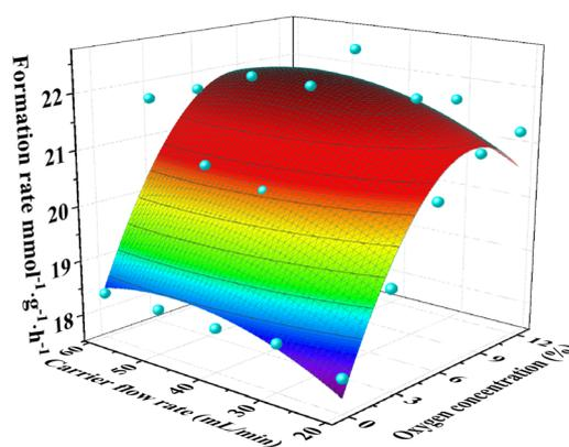
Fig. 11 Catalyst performance of the catalyst VPOC<sub>6</sub>, the reaction temperature was 300 °C. The liquid feed was a glycerol aqueous solution (20 wt%), with a LHSV of 6 mL h<sup>-1</sup>.
