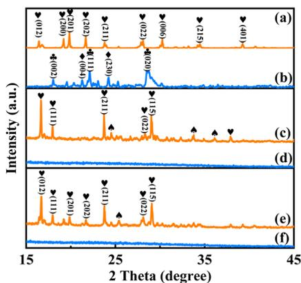
Fig. 1 XRD patterns of the catalysts, (a) pre-VPO, (b) VPO, (c) pre-VPNC<sub>6</sub>, (d) VPNC<sub>6</sub>, (e) pre-VPNC<sub>5</sub>, and (f) VPNC<sub>5</sub>. ♣- $\delta$ -VOPO<sub>4</sub> PDF # 47-0951, ◆- $\gamma$ -VOPO<sub>4</sub> PDF # 47-0950, ♥-(NH<sub>4</sub>)(VO<sub>2</sub>)HPO<sub>4</sub> PDF # 33-0062, ♣-V-P-N-C coordination compound.
