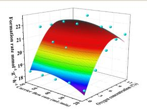
Fig. 11 Catalyst performance of the catalyst VPOC<sub>6</sub>, the reaction temperature was 300 °C. The liquid feed was a glycerol aqueous solution (20 wt%), with a LHSV of 6 mL  $h^{-1}$ .
