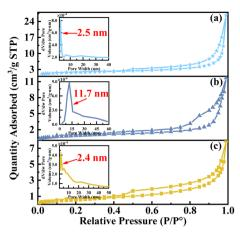
Fig. 4  $N_2$  adsorption-desorption isotherms of the catalysts, (a) VPO, (b) VPOC<sub>6</sub>, (c) VPOC<sub>5</sub>.
