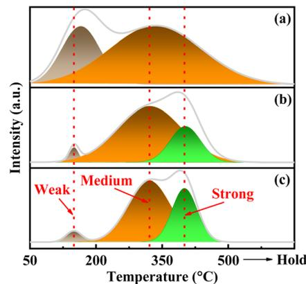
Fig. 8  $NH_3$ -TPD profiles of the catalysts, (a) VPO, (b) VPOC<sub>6</sub>, (c) VPOC<sub>5</sub>.
