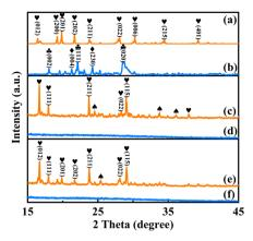
Fig. 1 XRD patters of the catalysts, (a) pre-VPO, (b) VPO, (c) pre-VPNC<sub>6</sub>, (d) VPNC<sub>6</sub>, (e) pre-VPNC<sub>5</sub>, and (f) VPNC<sub>5</sub>.  $\spadesuit$ - $\delta$ -VOPO<sub>4</sub> PDF # 47-0951,  $\spadesuit$ - $\gamma$ -VOPO<sub>4</sub> PDF # 47-0950,  $\Psi$ -(NH<sub>4</sub>)(VO<sub>2</sub>)HPO<sub>4</sub> PDF # 33-0062,  $\spadesuit$ -V-P-N-C coordination compound.
