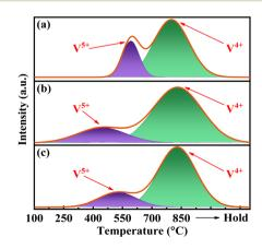
Fig. 5  $H_2$ -TPR profiles of the catalysts, (a) VPO, (b) VPOC<sub>6</sub>, (c) VPOC<sub>5</sub>.
