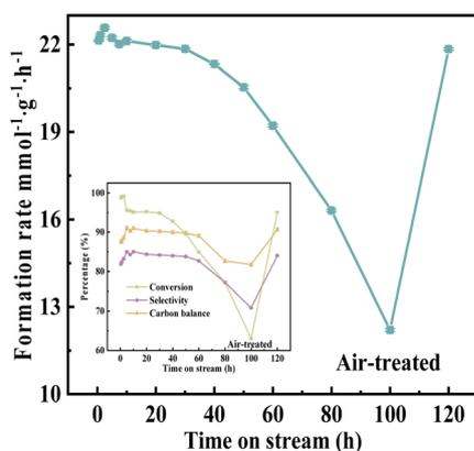
Fig. 12 Durability test over catalyst VPOC<sub>6</sub>, the reaction temperature and carrier flow rate were 320 °C and 40 mL min<sup>-1</sup> (9%-O<sub>2</sub>/N<sub>2</sub>), respectively. The liquid feed was a glycerol aqueous solution (20 wt%), with a LHSV of 6 mL h<sup>-1</sup>.
