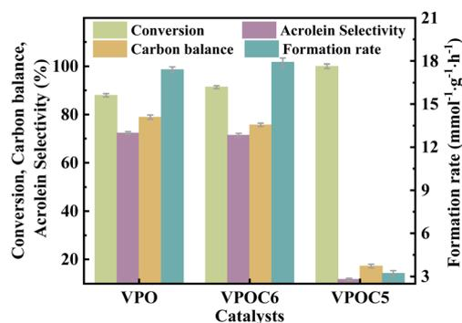
Fig. 9 Catalytic performance of the catalysts, the reaction temperature and carrier flow rate was 320 °C and 30 mL per min ( $N_2$ ), respectively. The liquid feed was a glycerol aqueous solution (20 wt%), with a LHSV of 6 mL h<sup>-1</sup>.
