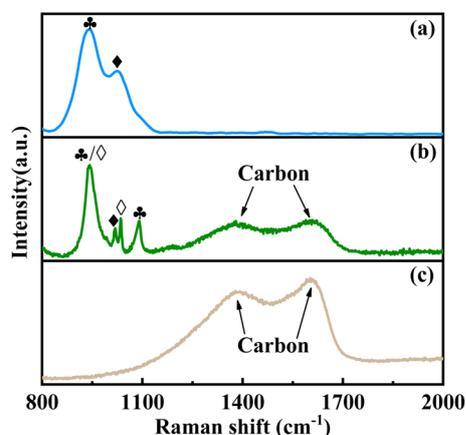
Fig. 2 Raman spectra of the catalysts, (a) VPO, (b) VPOC<sub>6</sub>, (c) VPOC<sub>5</sub>. ♣- $\delta$ -VOPO<sub>4</sub>, ◆-(VO)<sub>2</sub>P<sub>2</sub>O<sub>7</sub>, ◇- $\gamma$ -VOPO<sub>4</sub>.
