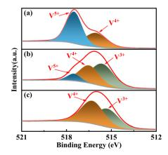
Fig. 7  $\,$  XPS spectra of V  $2p_{3/2}$  for the catalysts, (a) VPO, (b) VPOC6, (c) VPOC5.
