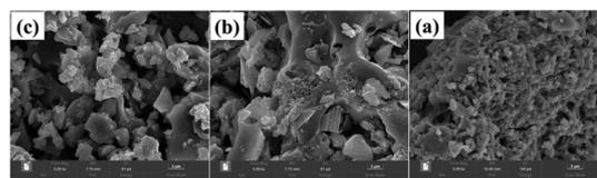
Fig. 3 SEM images of the catalysts, (a) VPO, (b) VPOC<sub>6</sub>, (c) VPOC<sub>5</sub>.
