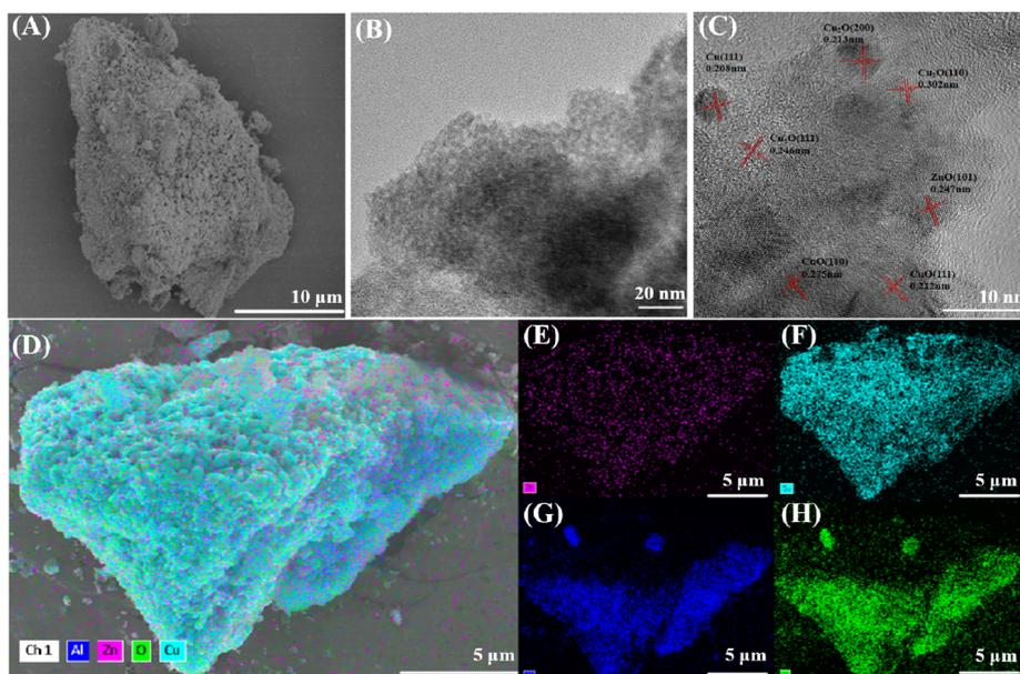
Fig. 2 (A) SEM image; (B) TEM image; (C) HRTEM image; (D–H) EDS elemental mappings of the CAZ<sub>1.5/2.0</sub>-200 catalyst.
