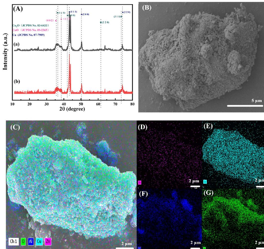
Fig. 9 (A) XRD patterns of catalysts: the fresh catalyst CAZ<sub>1.5/2.0</sub>-200 (a) and the recovered catalyst CAZ<sub>1.5/2.0</sub>-200 (R) (b); (B) SEM image of the recovered catalyst CAZ<sub>1.5/2.0</sub>-200 (R); (C–G) EDS elemental mappings of the recovered catalyst CAZ<sub>1.5/2.0</sub>-200 (R).
