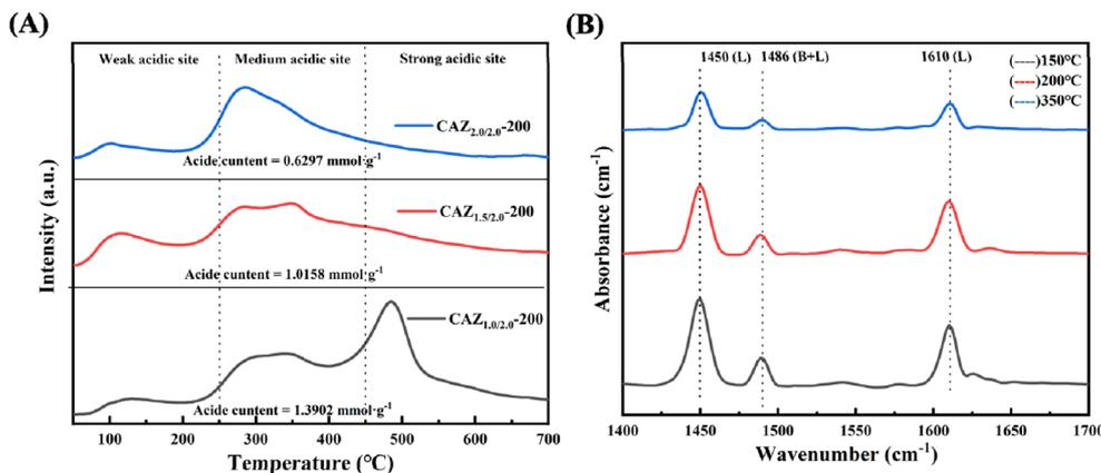
Fig. 4 (A)  $\text{NH}_3$ -TPD of the catalyst  $\text{CAZ}_{1.0/2.0}$ -200,  $\text{CAZ}_{1.5/2.0}$ -200 and  $\text{CAZ}_{2.0/2.0}$ -200. (B) Py-IR of the catalyst  $\text{CAZ}_{1.5/2.0}$ -200 at different test temperatures.
