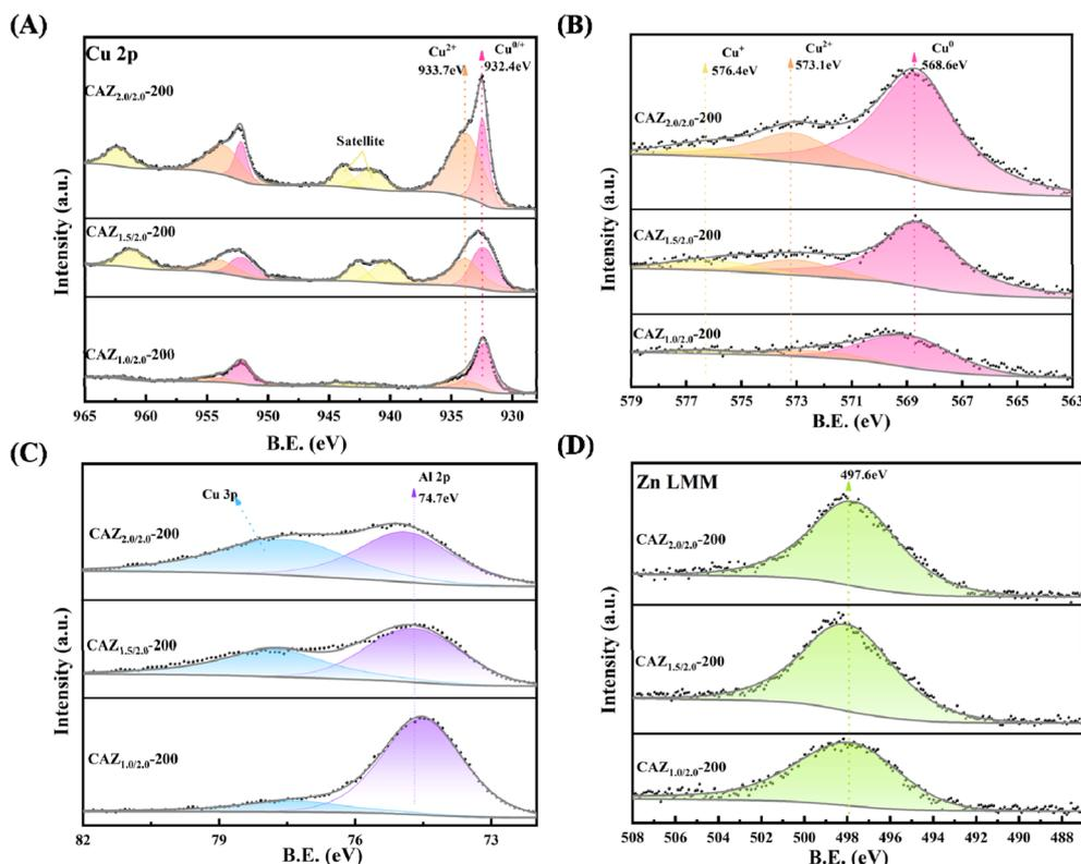
Fig. 3 XPS of these prepared catalysts in (A) Cu 2p spectra, (B) corresponding XAES spectra of Cu LMM, (C) Al 2p spectra, and (D) corresponding XAES spectra of Zn LMM for CAZ<sub>1.0/2.0-200</sub>, CAZ<sub>1.5/2.0-200</sub> and CAZ<sub>2.0/2.0-200</sub>.
