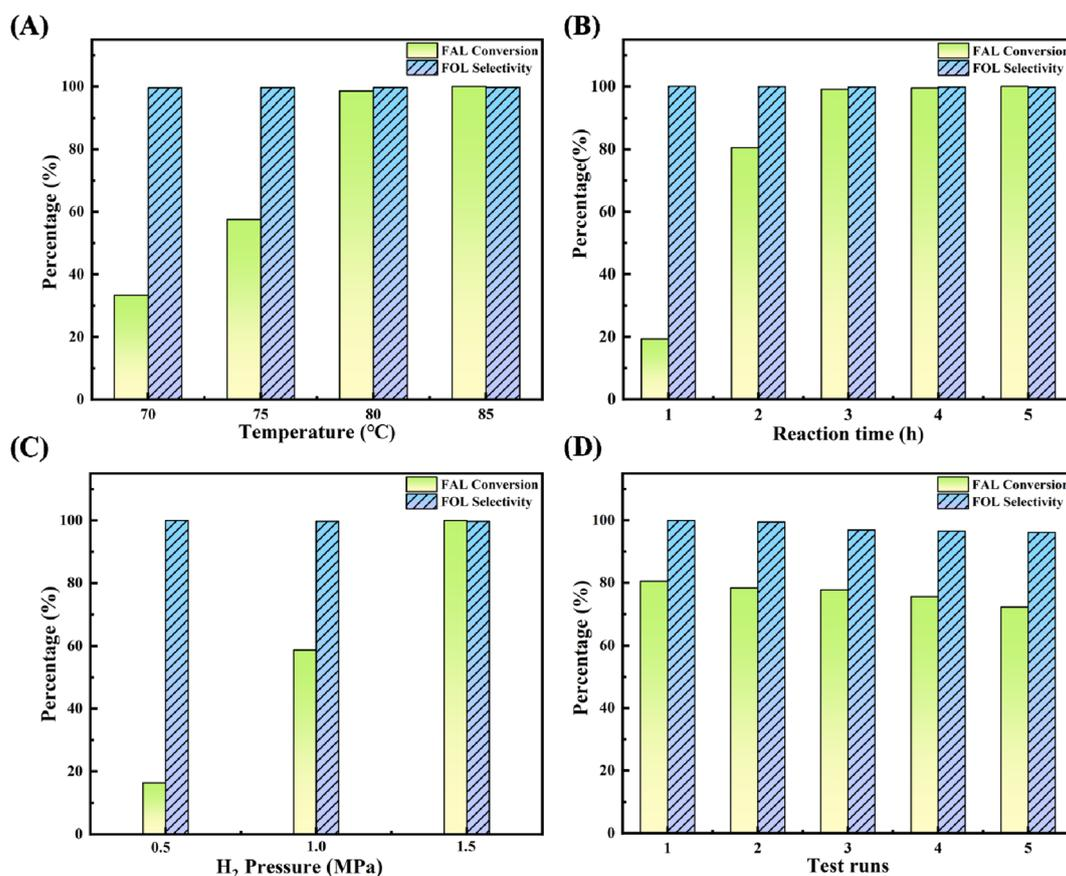
Fig. 8 The effect of reaction conditions on activity and reusability of the CAZ<sub>1.5/2.0</sub>-200 catalyst (reaction conditions: FAL (1.20 g), catalyst (0.24 g), ethanol (60.0 g), (A) 1.5 MPa H<sub>2</sub>, 5 h; (B) 85 °C, 1.5 MPa H<sub>2</sub>; (C) 85 °C, 4 h; (D) 85 °C, 1.5 MPa H<sub>2</sub>, 2 h).
