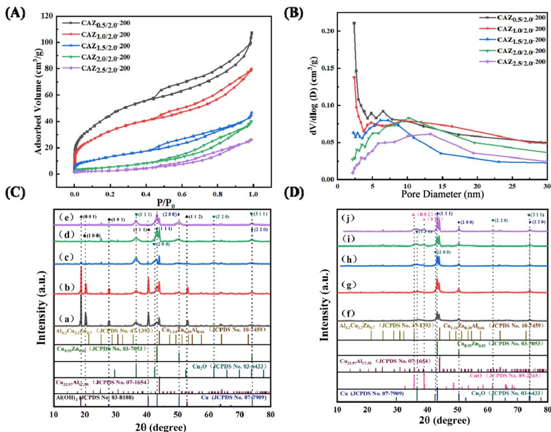
Fig. 1 (A)  $N_2$  adsorption–desorption isotherms; (B) pore size distribution obtained with the  $CAZ_{x/2.0-200}$  catalysts. XRD patterns of the catalysts; (C) etched precursor of (a)  $CAZ_{0.5/2.0}$ , (b)  $CAZ_{1.0/2.0}$ , (c)  $CAZ_{1.5/2.0}$ , (d)  $CAZ_{2.5/2.0}$  and (e)  $CAZ_{2.5/2.0}$ ; (D) after calcination and reduction of (f)  $CAZ_{0.5/2.0-200}$ , (g)  $CAZ_{1.0/2.0-200}$ , (h)  $CAZ_{1.5/2.0-200}$ , (i)  $CAZ_{2.0/2.0-200}$  and (j)  $CAZ_{2.5/2.0-200}$ .
