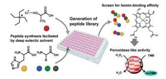
Fig. 1 The proposed approach to generate and screen catalytic peptides from DES-mediated ester-amide exchange reaction.
