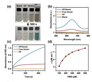
Fig. 4 (a) Color changes of TMB oxidation test. (b) UV-Vis spectra of different samples after 500 s of TMB oxidation. (c) Kinetics of TMB oxidation in different samples. (d) Michaelis–Menten kinetic fitting results of HF/hemin at different TMB concentrations. 500  $\mu$ M TMB, 500  $\mu$ M H<sub>2</sub>O<sub>2</sub>, and 16.67  $\mu$ M hemin were used. The molar ratio of amino acids to hemin was 80:1. HF peptides were prepared from a mixture of TEACl/a/H/F (100:100:100:100) at 120 °C for 3 days.
