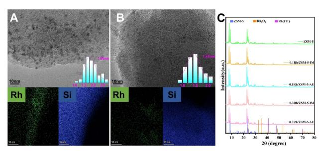
Fig. 1 (A) TEM and EDS mapping images of 0.3 Rh/ZSM-5-IM and (B) 0.3 Rh/ZSM-5-AE. (C) XRD results of ZSM-5, 0.1 Rh/ZSM-5-IM, 0.1 Rh/ZSM-5-AE, 0.3 Rh/ZSM-5-IM, and 0.3 Rh/ZSM-5-AE. (After experimental testing, the catalysts prepared by both methods showed the highest activity at a loading level of 0.3 wt%. Therefore, 0.3 Rh/ZSM-5 was selected for characterization and analysis in this study.) (The scale bar in TEM images is
