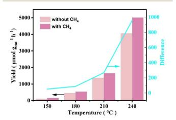
Fig. 4 0.3 Rh/ZSM-5-AE temperature-dependent CO $_2$  yield in CH $_4$ , O $_2$ , CO and N $_2$ , O $_2$ , CO gas atmospheres, respectively. The blue line corresponded to the right axis, indicating the difference in CO $_2$  produced under two different reaction conditions.
