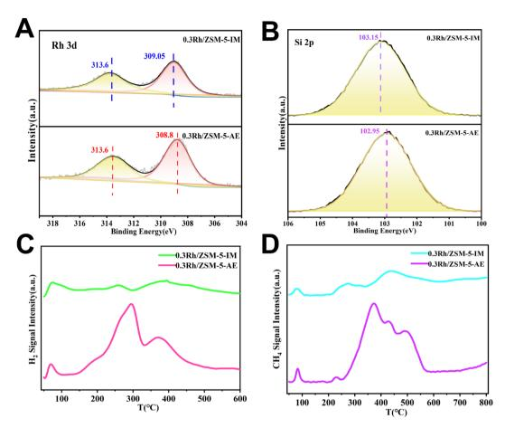
Fig. 2 (A) Rh 3d XPS spectra of 0.3 Rh/ZSM-5-IM and 0.3 Rh/ZSM-5-AE. (B) Si 2p XPS spectra of 0.3 Rh/ZSM-5-IM and 0.3 Rh/ZSM-5-AE. (C)  $H_2$ -TPR curves of 0.3 Rh/ZSM-5-IM and 0.3 Rh/ZSM-5-AE. (D)  $CH_4$ -TPD curves of 0.3 Rh/ZSM-5-IM and 0.3 Rh/ZSM-5-AE.
