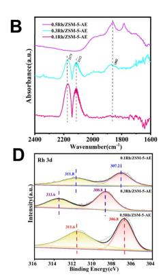
Fig. 5 (A) In situ DRIFTS spectra of 0.3 Rh/ZSM-5-AE at 240 °C in  $CH_4 + O_2$  atmosphere (20 : 3) and  $CH_4 + O_2 + CO$  (20 : 8 : 3) atmosphere, respectively. (B) In situ DRIFTS spectra of CO adsorption at 240 °C for AE samples with different loadings. (C)  $CH_4$ -TPD curves of AE samples with different loadings. (D) Rh 3d XPS spectra of AE samples with different loadings.
