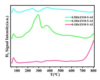
Fig. 6 H<sub>2</sub>-TPR curves of AE samples with different loadings.
