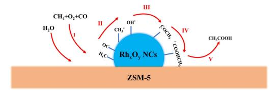
Fig. 7 Schematic of one possible reaction pathway.
