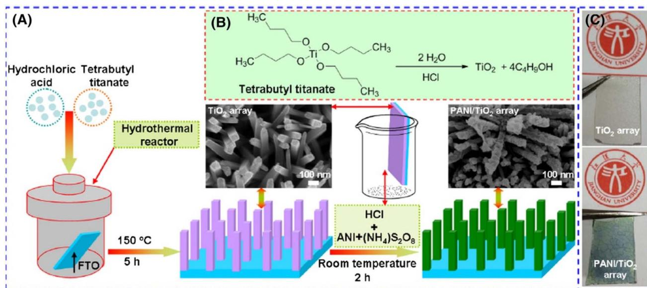
Fig. 6 (A) Synthesis of tetragonal prism array of TiO<sub>2</sub> deposited on fluorine-doped tin oxide (FTO) and followed by PANI coating, (B) synthesis of TiO<sub>2</sub> array *via* hydrolysis process, and (C) optical images of TiO<sub>2</sub>/FTO and PANI/TiO<sub>2</sub>/FTO.<sup>138</sup>
