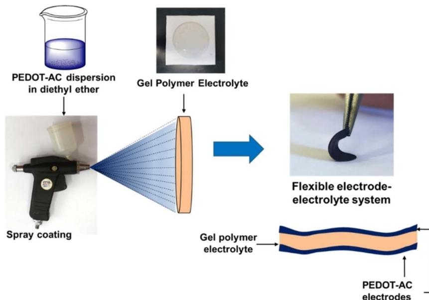
Fig. 19 Preparation of flexible electrode–electrolyte system.<sup>174</sup>
