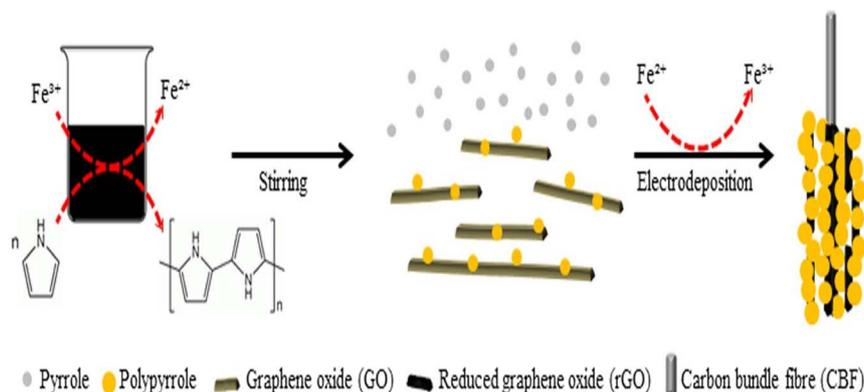
Fig. 15 Schematic diagram of the synthesis process of CBF/PPy-rGO-2.<sup>58</sup>
