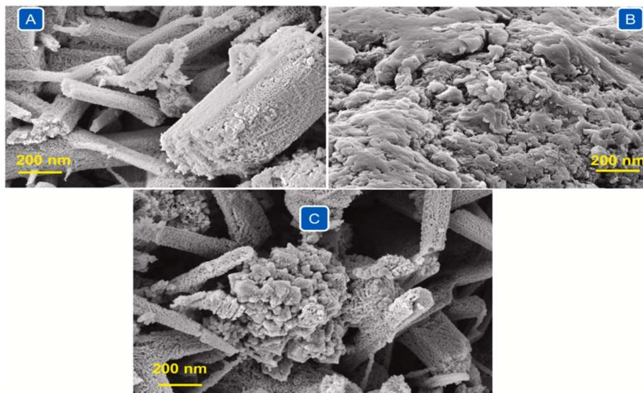
Fig. 5 FESEM image of (A) FeCO<sub>2</sub>O<sub>4</sub> (B) PANI and (C) FeCO<sub>2</sub>O<sub>4</sub>/PANI.<sup>132</sup>
