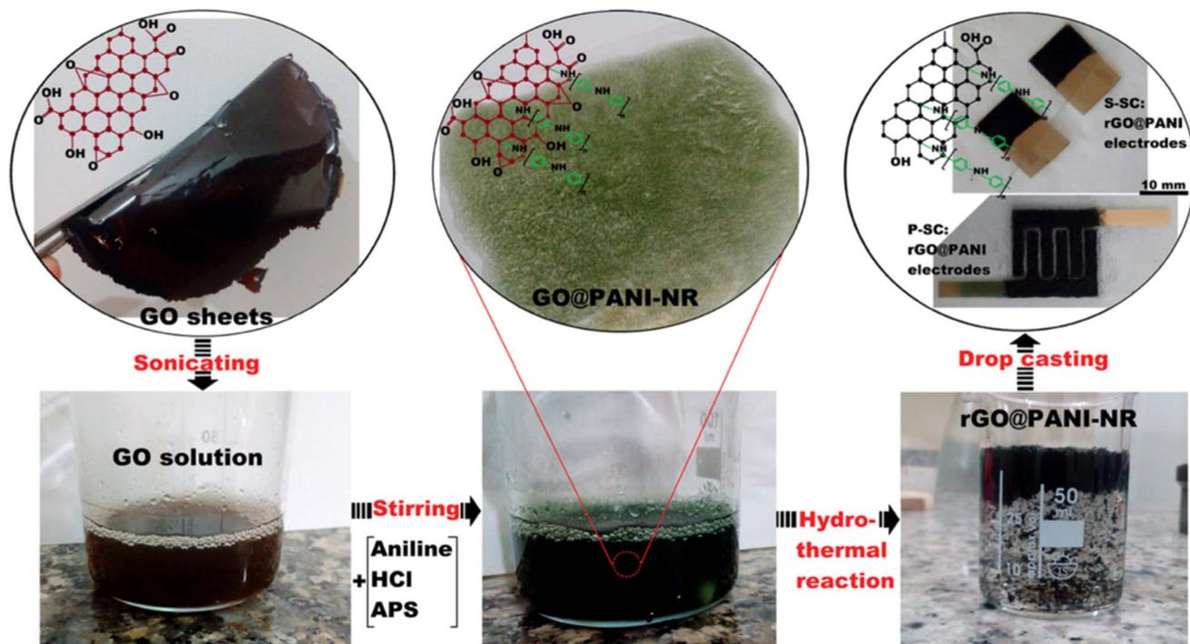
Fig. 10 Image showing the simple and ecofriendly synthesis and development procedures for rGO/PANI nanocomposites as active materials and supercapacitor electrodes.<sup>142</sup>
