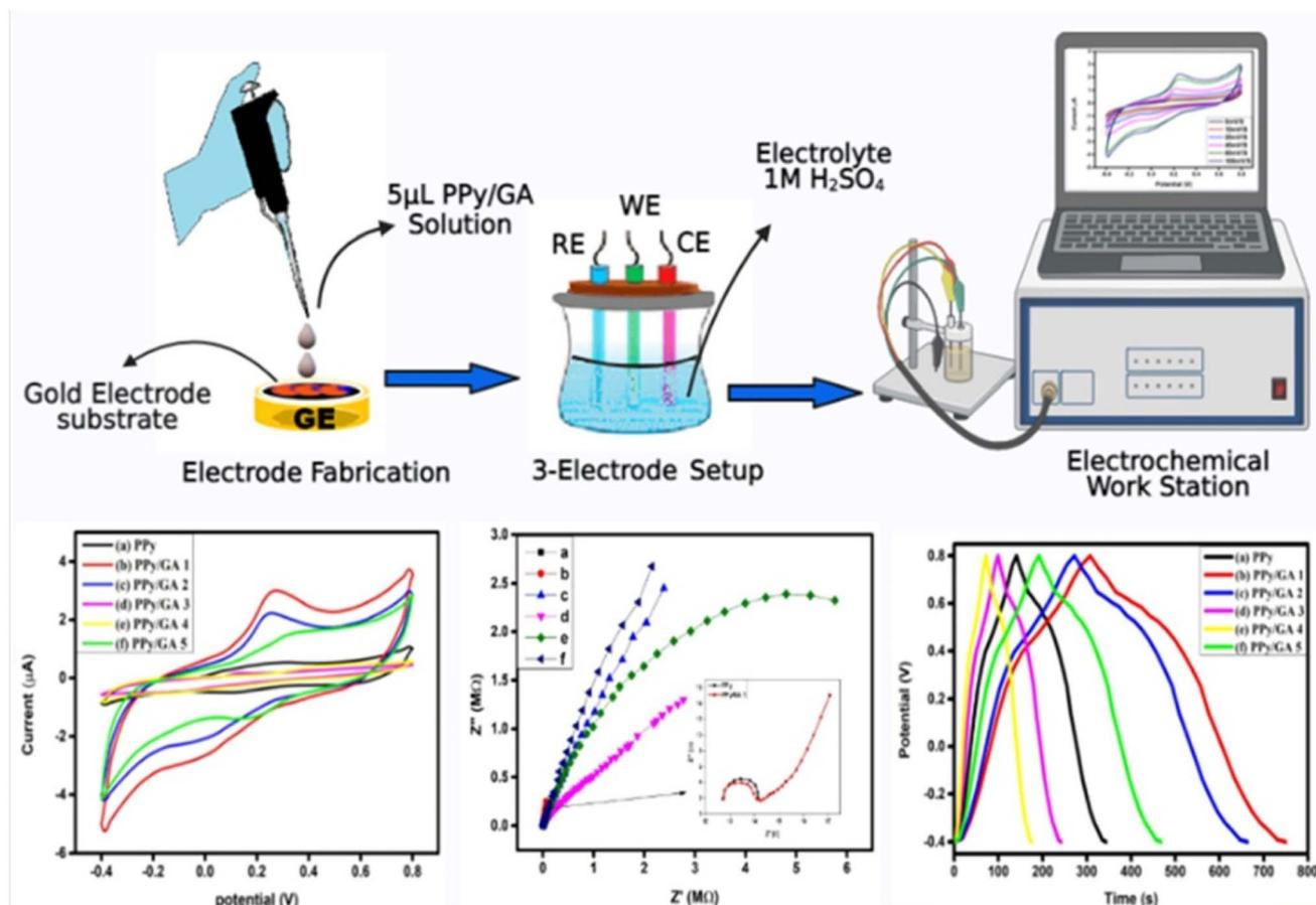
Fig. 16 Electrode fabrication towards electrochemical properties.<sup>157</sup>
