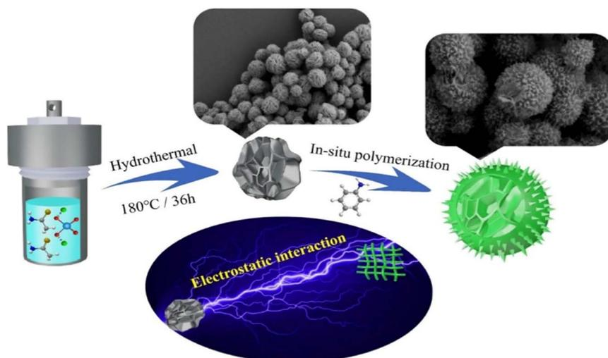
Fig. 8 An illustration of the synthesis process of MoS<sub>2</sub>/PANI hybrids through *in situ* oxidative polymerization.<sup>141</sup>
