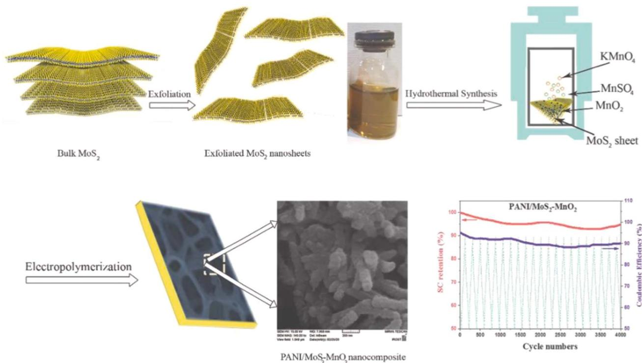
Fig. 11 Synthesis route for ternary PANI/MoS<sub>2</sub>-MnO<sub>2</sub> hybrid nanocomposite.<sup>147</sup>
