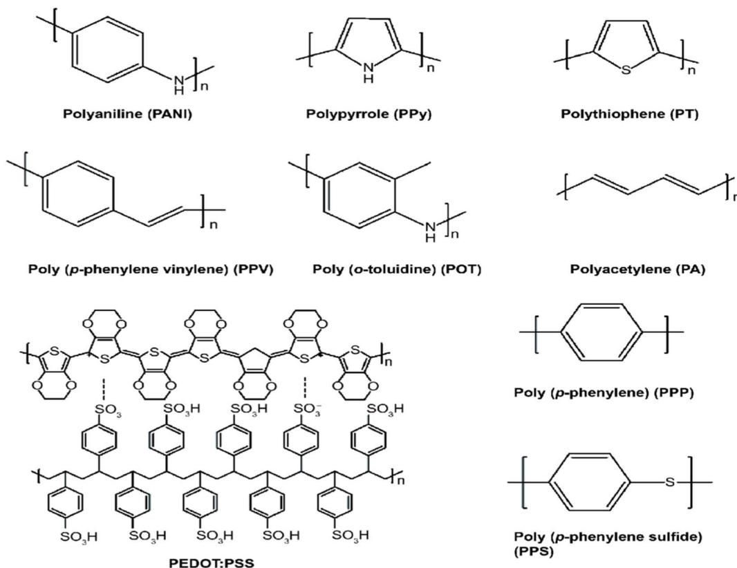
Fig. 3 Chemical structures of selected conducting polymers.<sup>101</sup>
