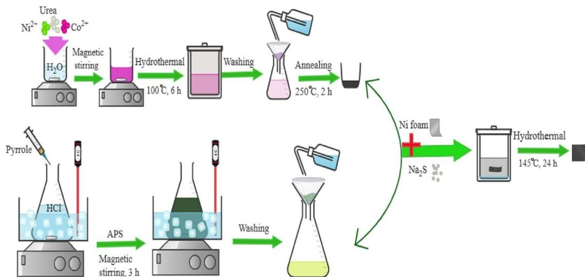
Fig. 14 Schematic representation of  $\text{NiCo}_2\text{S}_4@\text{PPy}$  nanomaterial fabrication.<sup>160</sup>
