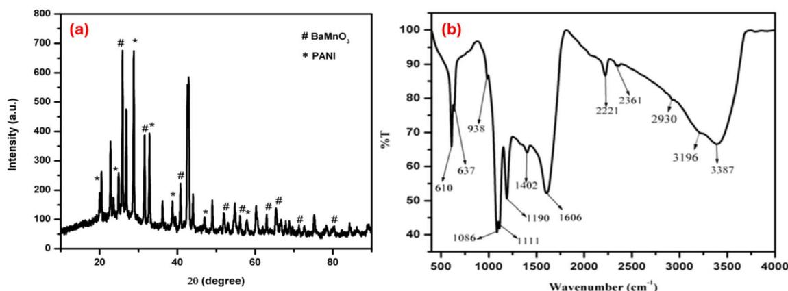
Fig. 4 (a) XRD patterns of PANI- $\text{BaMnO}_3$  nanocomposite and (b) FT-IR spectrum of PANI- $\text{BaMnO}_3$  nanocomposite.<sup>128</sup>
