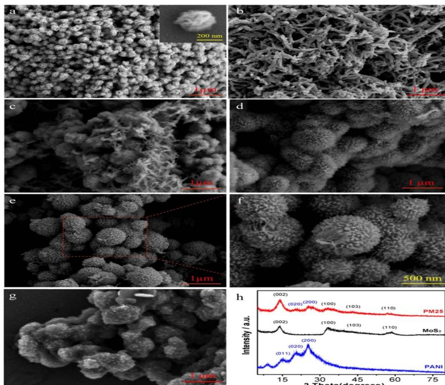
Fig. 9 SEM images of (a) pure MoS<sub>2</sub>, (b) pure PANI; (c) PM<sub>15</sub>; (d) PM<sub>20</sub>; (e) and (f) PM<sub>25</sub>; (g) PM<sub>33</sub>; and (h) XRD patterns of PANI, MoS<sub>2</sub>, and PM<sub>25</sub>.<sup>141</sup>
