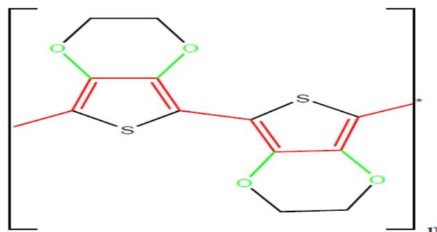
Fig. 17 Chemical structure of conjugated conductive polymer poly(3,4-ethylene dioxythiophene).<sup>163</sup>
