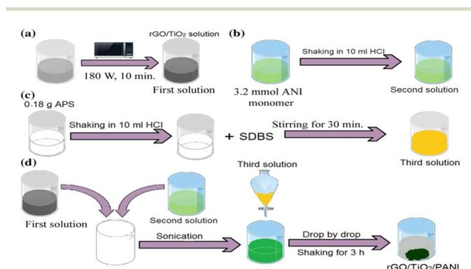
Fig. 7 Schematic showing the synthesis of rGO/TiO<sub>2</sub>/PANI nanocomposite via *in situ* emulsion polymerization: (a) preparation of rGO/TiO<sub>2</sub> suspension, (b) addition of 3.2 mmol ANI monomer, (c) addition of 0.18 g APS and SDBS with stirring and (d) sonication drop-by-drop addition of APS solution with shaking for 3 hours.<sup>139</sup>
