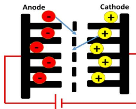
Fig. 1 Major components of a supercapacitor.<sup>74</sup>
