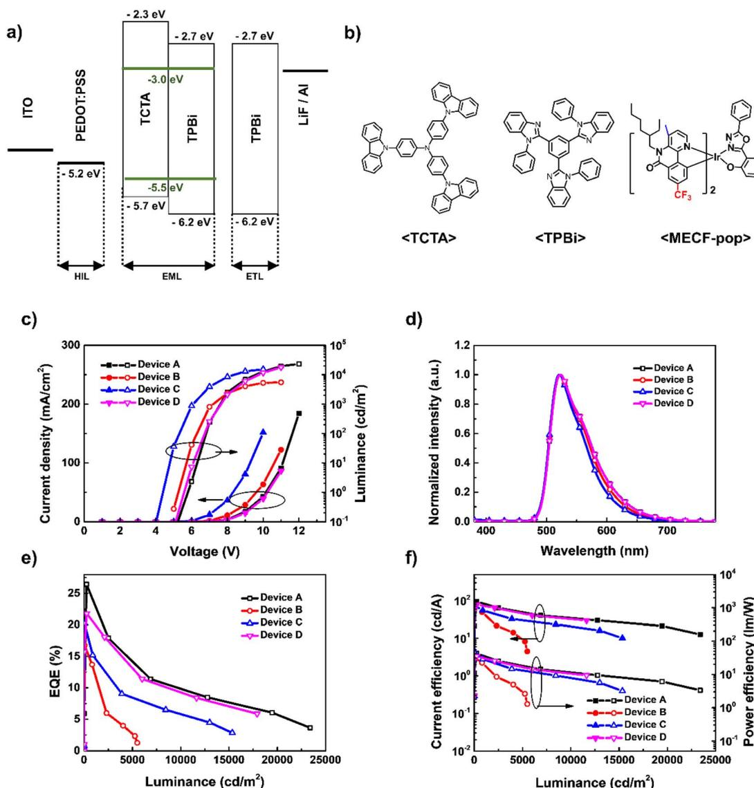
Fig. 2 (a) Energy level diagram of solution-processed PHOLEDs. (b) Molecular structure of TCTA, TPBi, and MECF-pop, (c)  $J$ - $V$ - $L$  curve, (d) EL spectra, (e) EQE- $L$  curve, and (f) CE- $L$ -PE curve of Devices A-D.
