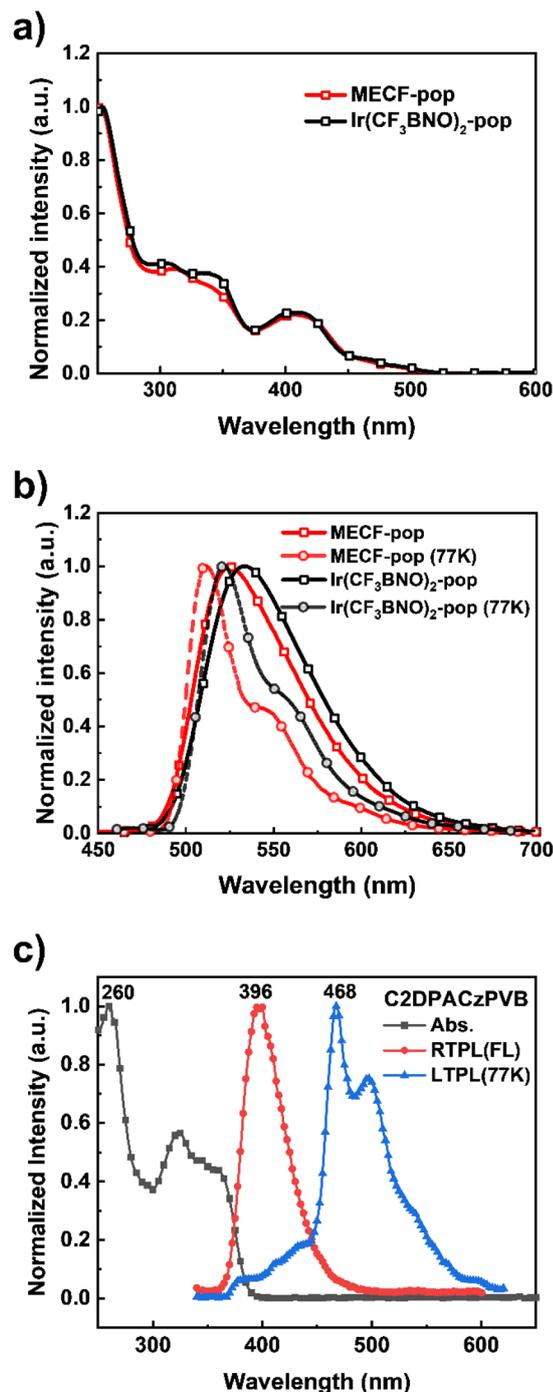
Fig. 1 (a) UV-vis absorption, (b) PL spectra of MECF-pop and Ir(CF<sub>3</sub>-BNO)<sub>2</sub>-pop. (c) UV-vis absorption, RTPL (FL) and LTPL (Ph) spectra of C2DPACzPVB.
