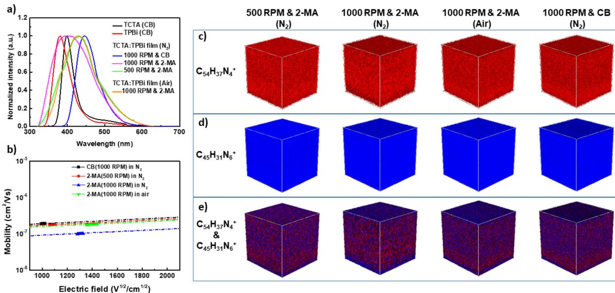
Fig. 3 (a) PL properties of TCTA, TPBi, and mixed films (TCTA and TPBi). (b) Hole mobility of mixed films depending on film forming conditions using CB and 2-MA. ToF-SIMS 3D analysis of (c) TCTA (C<sub>54</sub>H<sub>37</sub>N<sub>4</sub><sup>+</sup>), (d) TPBi (C<sub>45</sub>H<sub>31</sub>N<sub>6</sub><sup>+</sup>), and (e) mixed TCTA and TPBi distribution according to film forming conditions.
