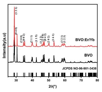
Fig. 1 XRD patterns of pure BVO and BVO: Er/Yb samples. The corresponding standard JCPDS card data of BVO (JCPDS##96-901-3438) is given as a reference.
