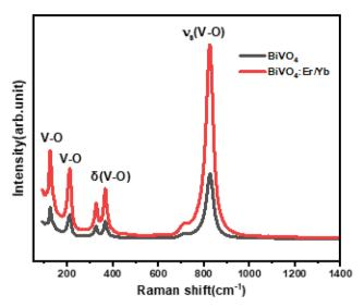
Fig. 3 Raman spectra of pure BVO and BVO: Er/Yb samples.
