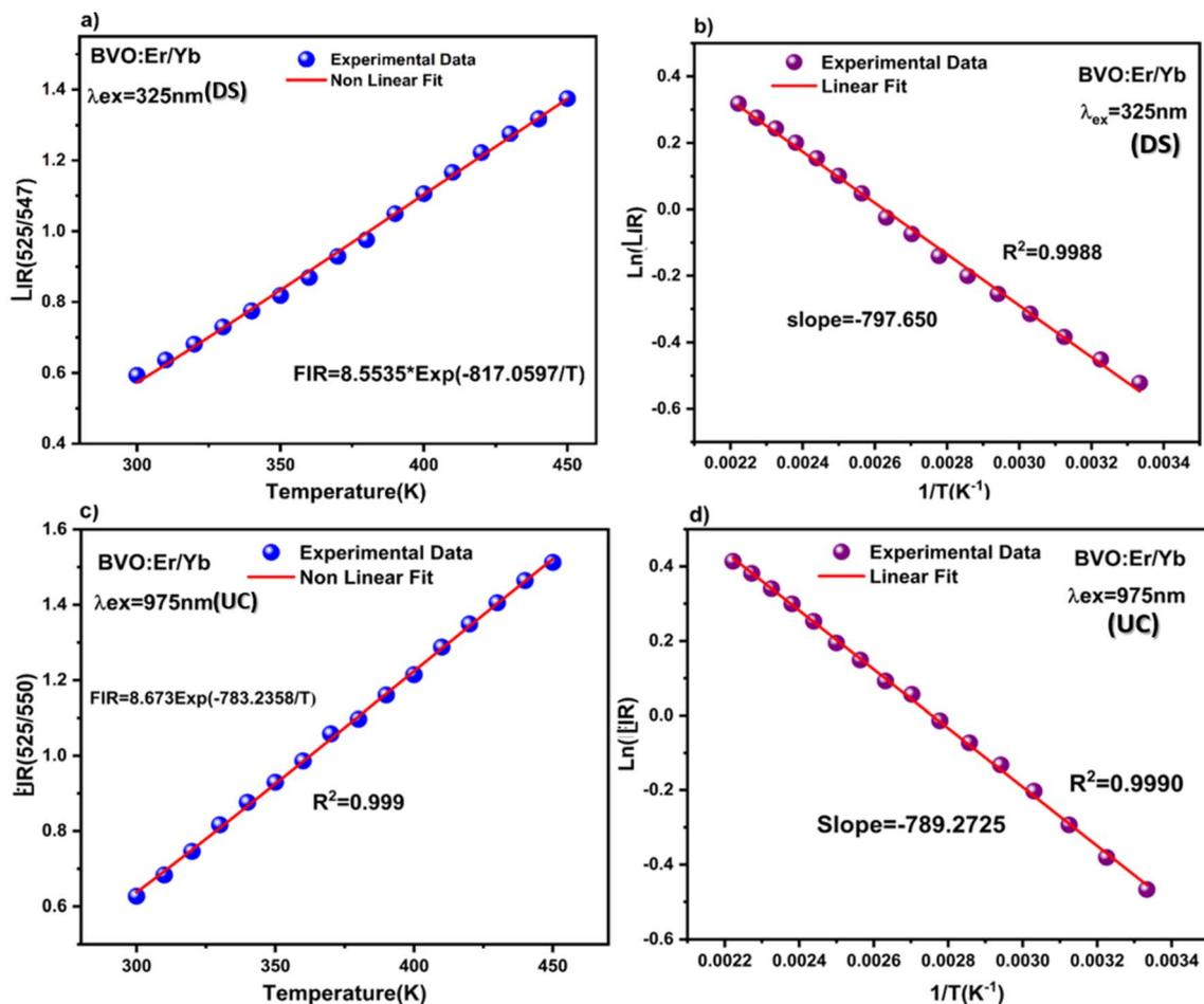
Fig. 9 Luminescence intensity ratio LIR as a function of temperature. (a) under 325 nm (DS); (c) under 975 nm (UC). Monolog plot of the LIR as a function of the inverse temperature ( $1/T$ ). (b) under 325 nm (DS); (d) under 975 nm (UC).
