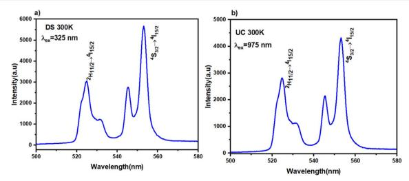
Fig. 5 Emission spectra of BVO: Er/Yb at room temperature (a) under 325 nm excitation (DS), (b) under 975 nm excitation (UC), respectively.
