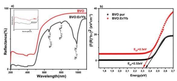
Fig. 4 (a) UV-vis-NIR diffuse reflectance spectra (inset spectra from 200–500 nm region), (b) the plot of gap energy of pure BVO and BVO: Er/Yb samples.
