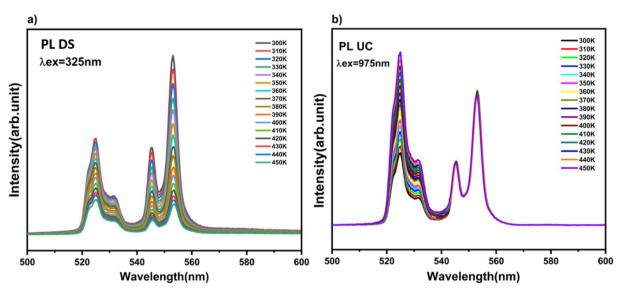
Fig. 8 Emission spectra of the BVO: Yb/Er phosphor for different temperatures in the visible range (a) under 325 nm excitation (DS), (b) under 975 nm (UC) excitation.
