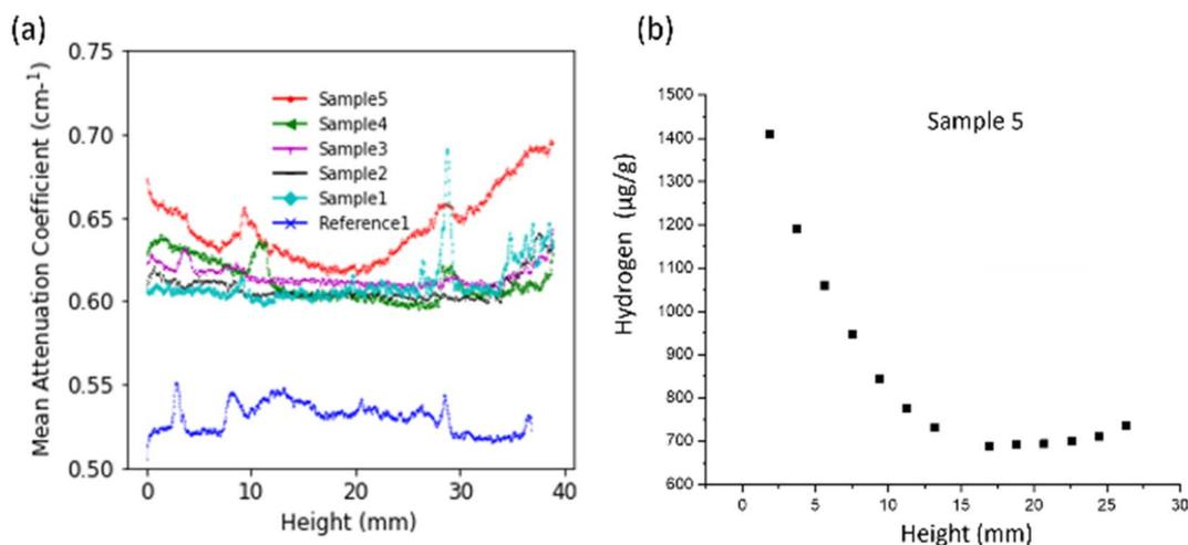
Fig. 5 Plot showing mean neutron attenuation obtained from neutron tomography of all samples (a) along height. (b) Concentration sample 5 from chemical analysis.
