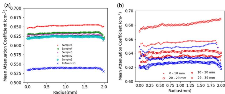
Fig. 6 Plot showing mean neutron attenuation obtained from neutron tomography of all samples (a) radially (b) along height (sample 5 in red and reference 1 sample in blue, different markers for different heights are indicated in legend).
