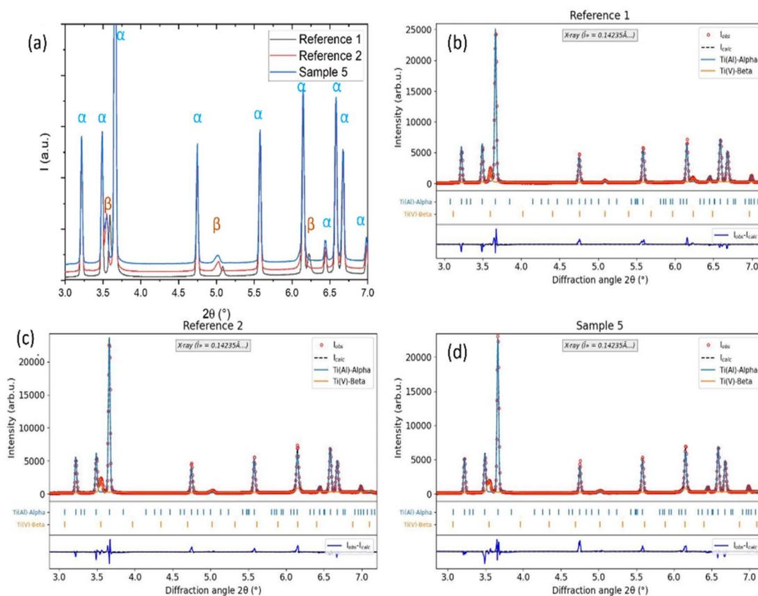
Fig. 7 XRD pattern of samples: reference 1, reference 2 and sample 5 (a) and corresponding Rietveld refinements (b–d) by taking into account  $\alpha$  and  $\beta$  phases. The observed data (red circles), calculated data (blue line for  $\alpha$  phase, orange for  $\beta$  phase and black line total fit), and difference plots (blue line), together with the positions of the Bragg reflections, are depicted for all the samples.
