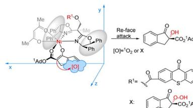
Fig. 17 Stereinduction model of asymmetric  $\alpha$ -hydroxylation catalyzed by complexation of ketone **C17** with Ni ( $\text{acac}$ )<sub>2</sub>.
