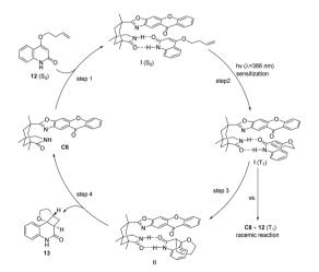
Fig. 6 Mechanism of asymmetric [2 + 2] photocycloaddition of quinolones catalyzed by ketone C8.
