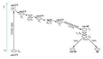
Fig. 13 Photosensitive deracemization mechanism of racemates.
