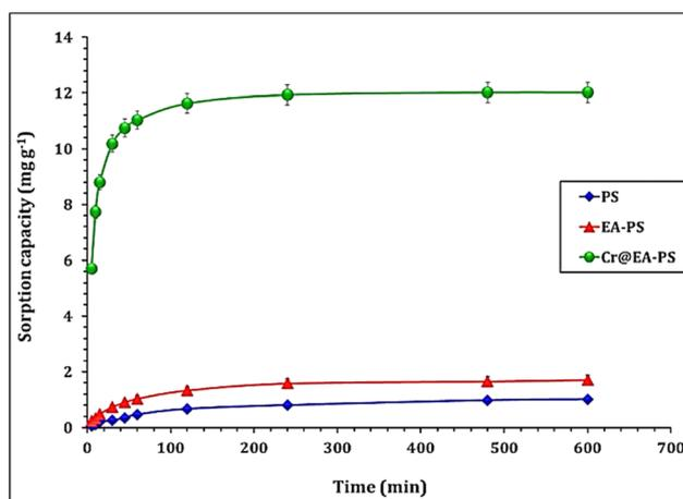
Fig. 6 Influence of the contact time on the Cd(II) adsorption capacity (pH 6.9; temperature of 25 ± 1 °C; initial concentration of 50 mg L<sup>-1</sup>; sorbent dosage of 3.0 g L<sup>-1</sup>).
