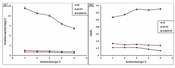
Fig. 8 The dependence of sorption capacity (I) and the distribution coefficient ( $\log K_d$ ) (II) on the sorbent dose (room temperature; initial concentration of 50 mg L<sup>-1</sup>; time of 240 min; solution pH 6.9).
