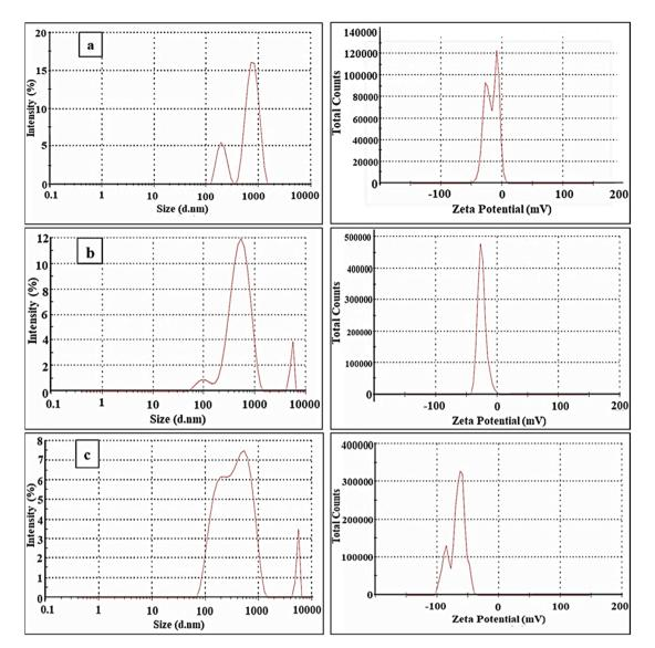
Fig. 4 DLS measurements and zeta potential curves of (a) polystyrene, (b) ethanolamine-blended polystyrene, (c) Cr(OH)<sub>3</sub>-impregnated polystyrene/ethanolamine.
