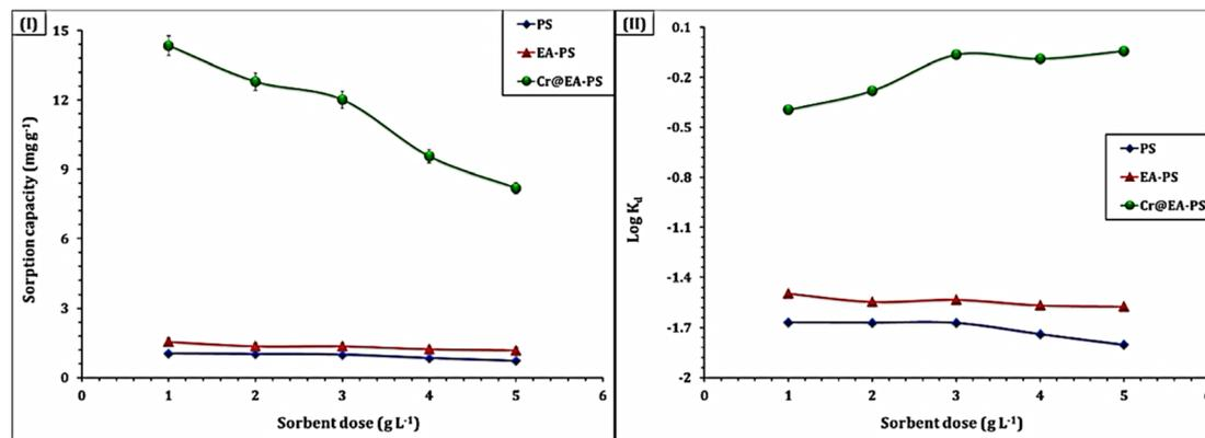
Fig. 8 The dependence of sorption capacity (I) and the distribution coefficient ( $\log K_d$ ) (II) on the sorbent dose (room temperature; initial concentration of 50 mg L<sup>-1</sup>; time of 240 min; solution pH 6.9).
