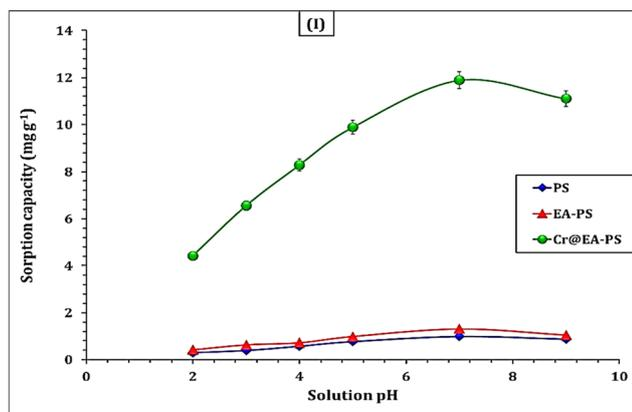
Fig. 5 The variation of Cd(II) sorption capacity as a function of pH (time: 240 min; room temperature; initial concentration: 50 mg L<sup>-1</sup>; and sorbent dose: 3.0 g L<sup>-1</sup>).
