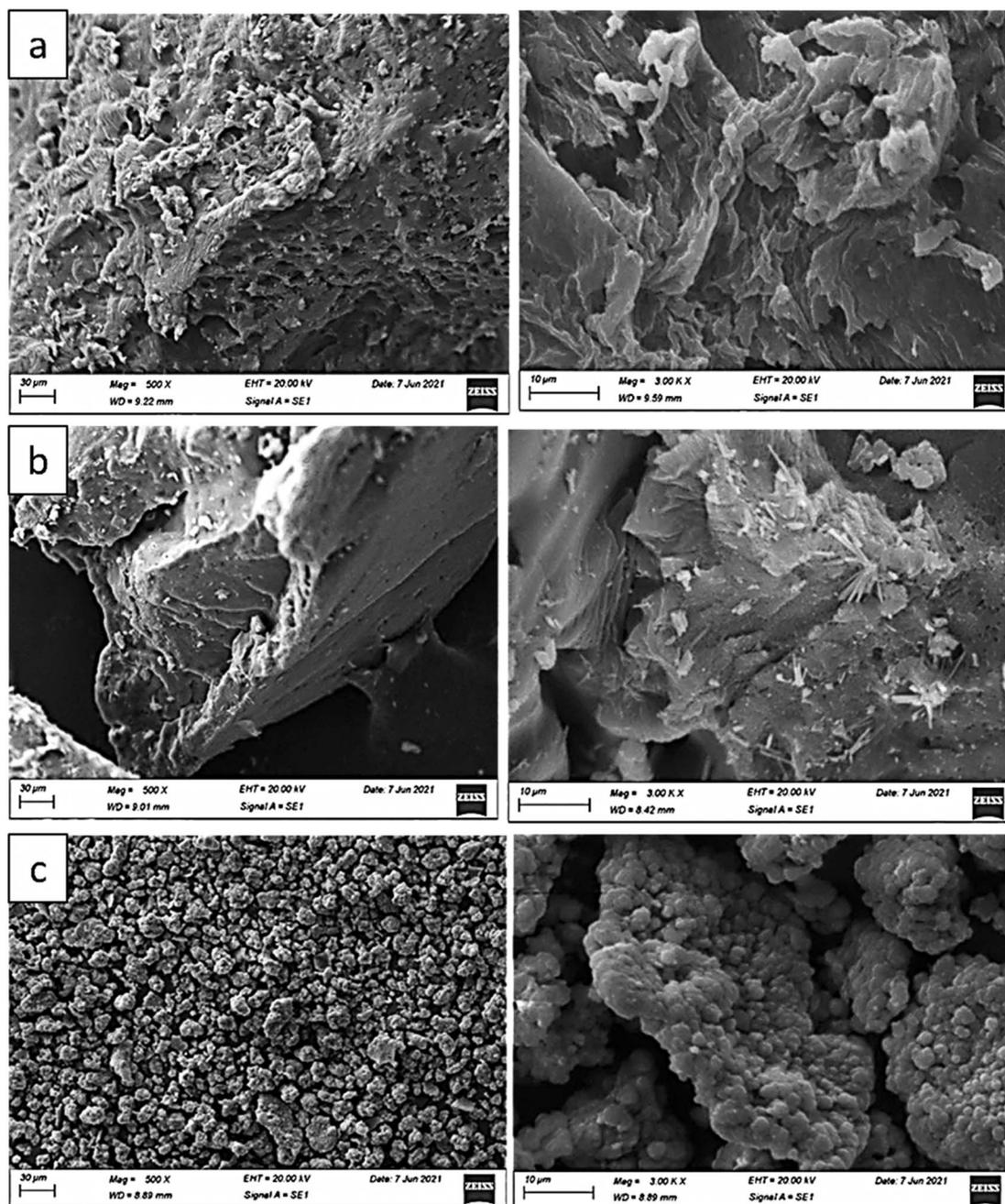
Fig. 3 SEM image of (a) polystyrene, (b) ethanolamine-blended polystyrene, (c) Cr(OH)<sub>3</sub>-impregnated polystyrene/ethanolamine.
