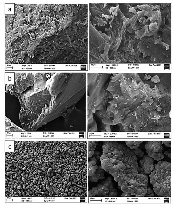
Fig. 3 SEM image of (a) polystyrene, (b) ethanolamine-blended polystyrene, (c) Cr(OH)<sub>3</sub>-impregnated polystyrene/ethanolamine.
