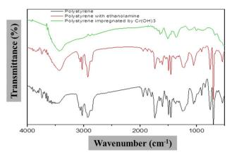
Fig. 1 FTIR of polystyrene, ethanolamine-blended polystyrene, and Cr(OH)<sub>3</sub>-impregnated polystyrene/ethanolamine.
