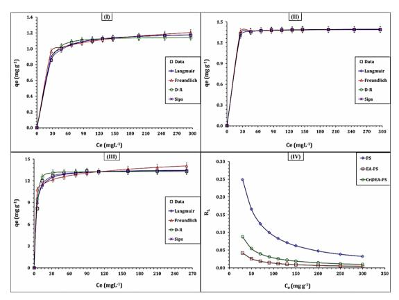
Fig. 10 The isotherm profile of PS(I), EA-PS(II), and Cr@EA-PS(III) materials. The dimensionless  $R_1$  values for the three sorbents (IV).
