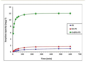
Fig. 6 Influence of the contact time on the Cd( $\shortparallel$ ) adsorption capacity (pH 6.9; temperature of 25  $\pm$  1 °C; initial concentration of 50 mg L $^{-1}$ ; sorbent dosage of 3.0 g L $^{-1}$ ).
