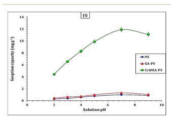
Fig. 5 The variation of Cd( $_{\rm II}$ ) sorption capacity as a function of pH (time: 240 min; room temperature; initial concentration: 50 mg L $^{-1}$ ; and sorbent dose: 3.0 g L $^{-1}$ ).
