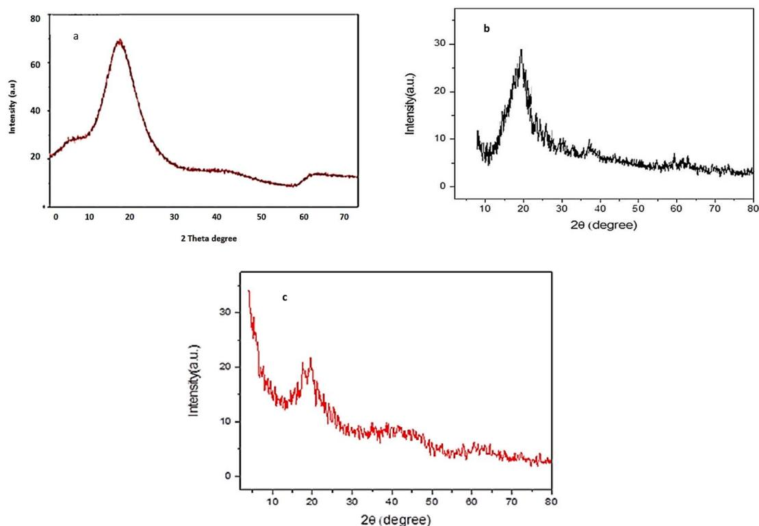
Fig. 2 XRD patterns of (a) PS, (b) EA-PS and (c) the Cr(OH)<sub>3</sub>-impregnated polystyrene/ethanolamine composite.
