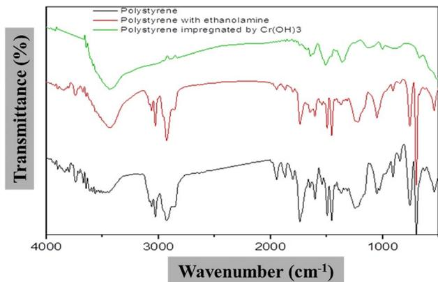
Fig. 1 FTIR of polystyrene, ethanolamine-blended polystyrene, and Cr(OH)<sub>3</sub>-impregnated polystyrene/ethanolamine.
