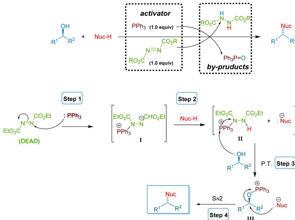
Fig. 3 The recognized mechanism of the Mitsunobu reaction.
