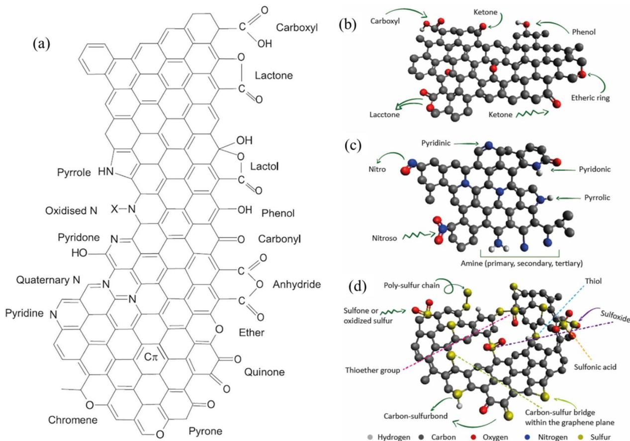
Fig. 1 (a) Nitrogen and oxygen surface functional groups on carbons.<sup>62</sup> Different surface functional groups on the surface biomass: (b) oxygenated functional groups (c) nitrogen functional groups (d) sulfur functional groups.
