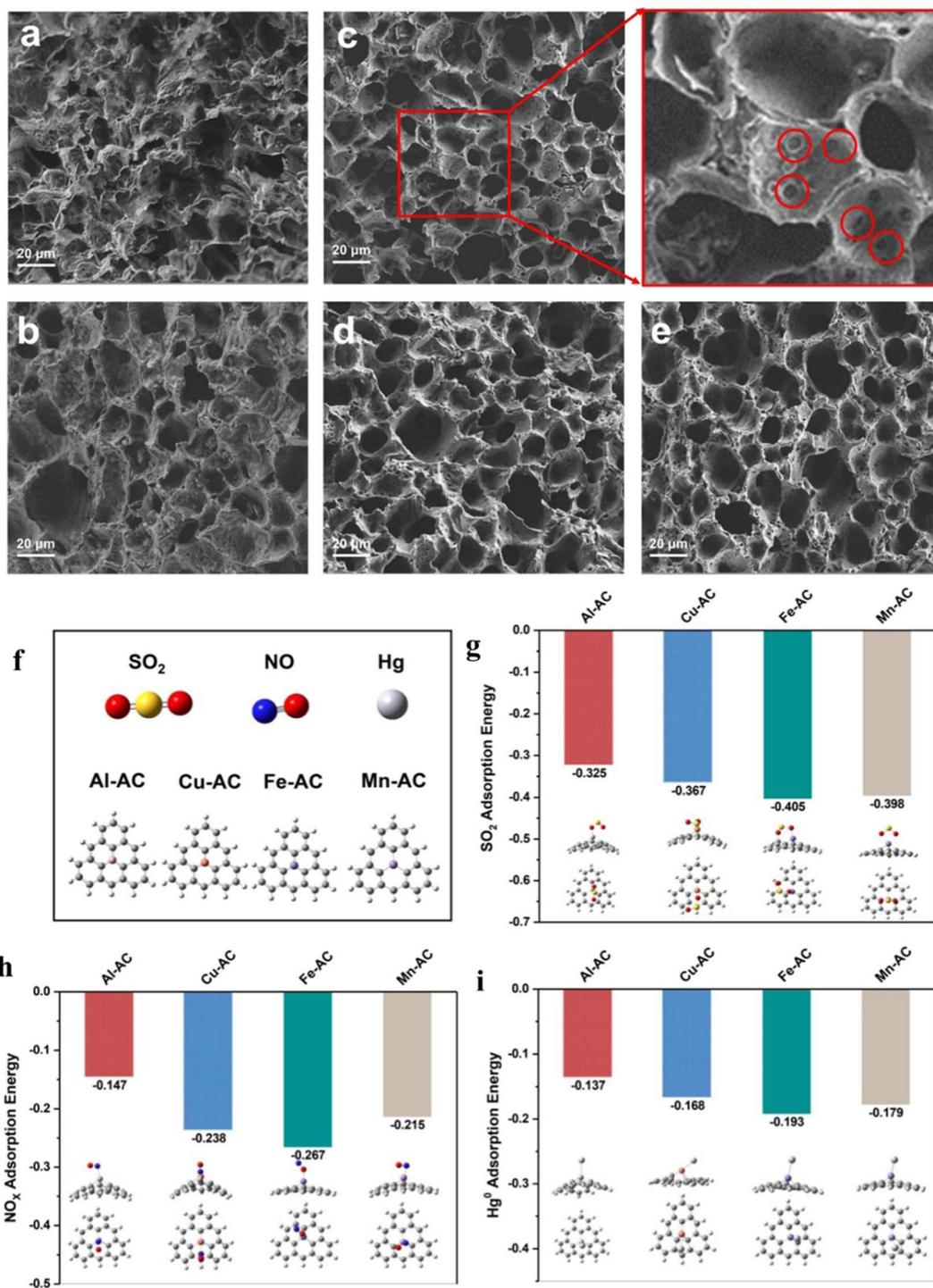
Fig. 8 SEM images at (a) 500 °C (b) 600 °C (c) 700 °C (d) 800 °C (e) 900 °C. (f–i) Molecular structures and energy states of  $\text{SO}_2$ ,  $\text{NO}_x$  and  $\text{Hg}^0$  adsorbed on walnut shell-based carbon.<sup>290</sup>
