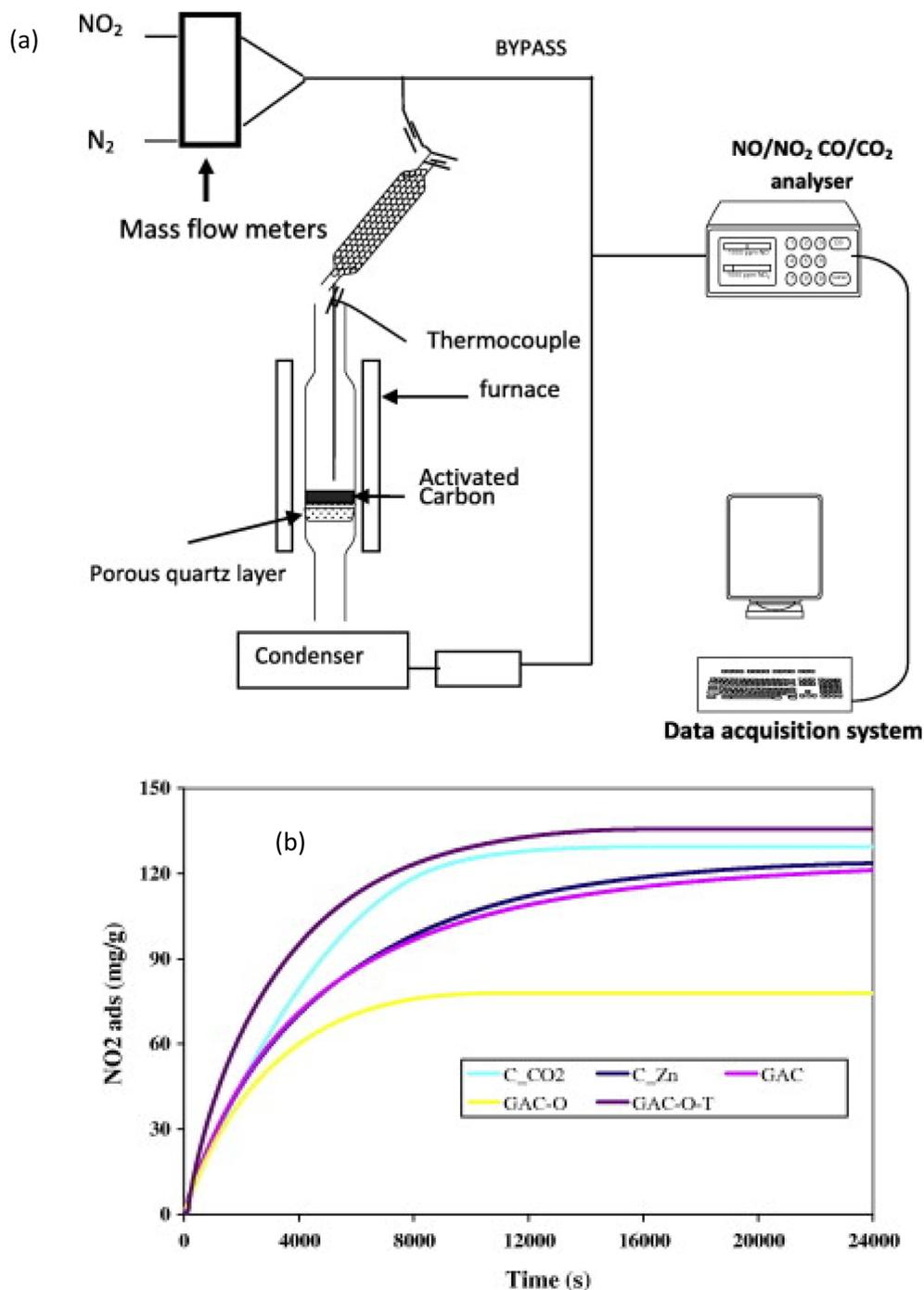
Fig. 5 (a) Scheme of the set-up for the NO<sub>2</sub> adsorption experiments. (b) NO<sub>2</sub> adsorption capacities at 25 °C for the different activated carbons.<sup>245</sup>
