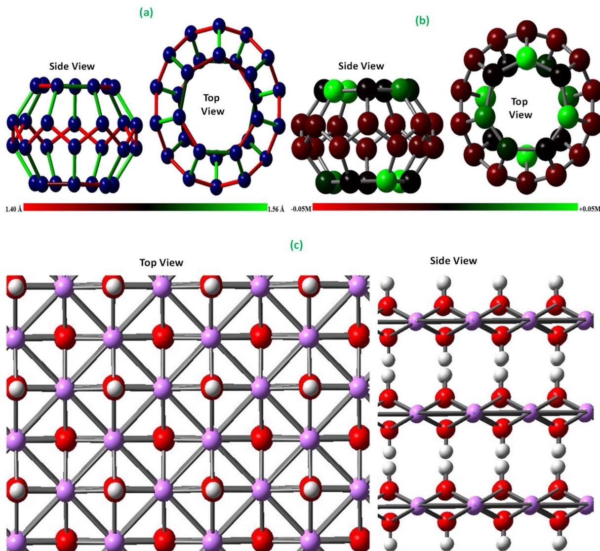
Fig. 9 (a): Modeled structure of AC with chemical formula C<sub>28</sub>, which fullerene includes pentagonal and heptagonal rings; (b): the electric charge distribution of the C<sub>28</sub> structure on the Mulliken scale; (c): LiOH crystal structure showing the top and side view.<sup>318</sup>
