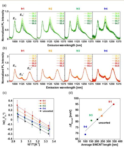
Fig. 7 Temperature-dependent PL spectra (excitation: 570 nm) of the length-sorted (a) gel-coated If-SWCNTs- $pNO_2$  solution and (b) gel-coated If-SWCNTs- $pPNO_2$  solution in H<sub>2</sub>O, (c) the van't Hoff plot of the length-sorted and unsorted gel-coated If-SWCNTs- $pNO_2$  solution, and (d) plot of  $\Delta E_{\text{thermal}}$  as a function of the average SWCNT length. Error bars mean the error estimated during peak deconvolution.
