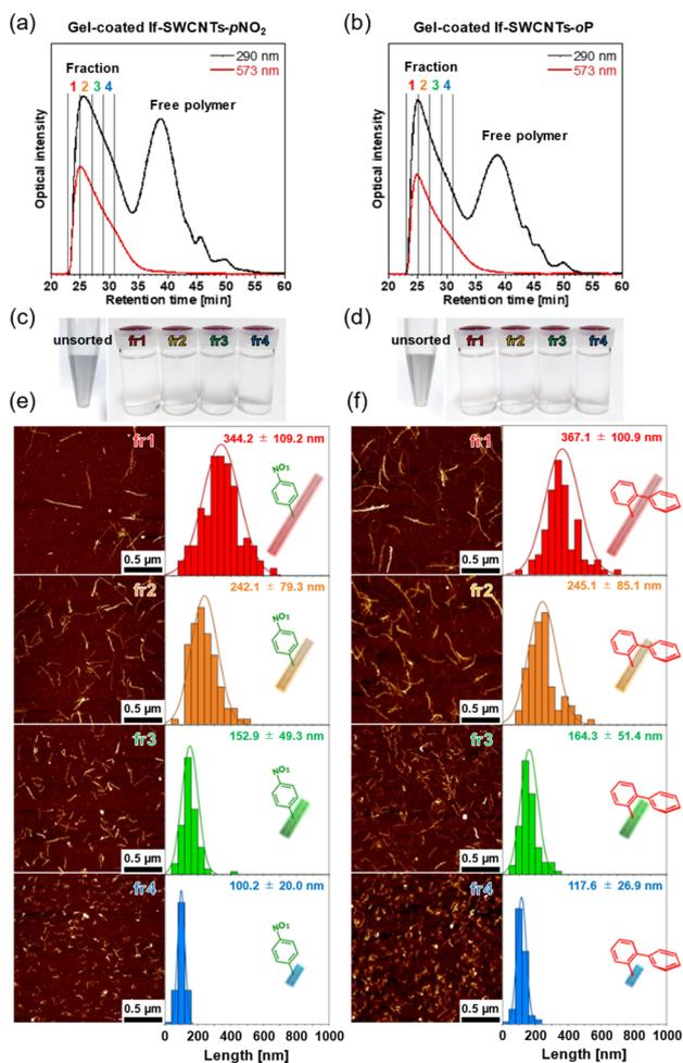
**Fig. 5** (a and b) Size exclusion chromatograms, (c and d) photographs of fractionated solutions, and (e and f) AFM images and length distribution histogram of the (a–c) gel-coated lf-SWCNTs-*p*NO<sub>2</sub> and (d–f) gel-coated lf-SWCNTs-*o*P. Displayed values are the mean length  $\pm$  standard deviation for  $N = 100$ .
