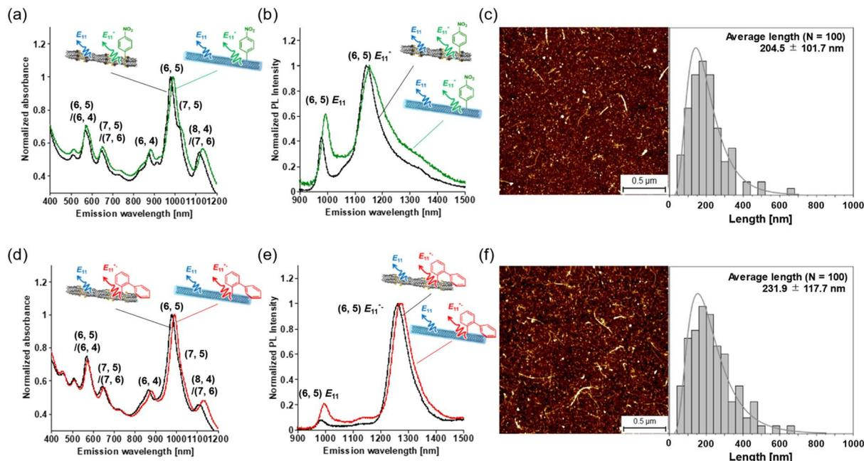
Fig. 2 (a) Absorption and (b) PL spectra (excitation: 570 nm) of SDBS-dispersed lF-SWCNTs-*p*NO<sub>2</sub> (black) and gel-coated lF-SWCNTs-*p*NO<sub>2</sub> (green) in D<sub>2</sub>O. (c) AFM image and length distribution of gel-coated lF-SWCNTs-*p*NO<sub>2</sub>. (d) Absorption and (e) PL spectra (excitation: 570 nm) of SDS-dispersed lF-SWCNTs-*o*P (black) and gel-coated lF-SWCNTs-*o*P (red) in D<sub>2</sub>O, and (f) AFM image and length distribution of gel-coated lF-SWCNTs-*o*P.
