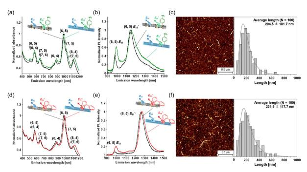
Fig. 2 (a) Absorption and (b) PL spectra (excitation: 570 nm) of SDBS-dispersed If-SWCNTs-pNO<sub>2</sub> (black) and gel-coated If-SWCNTs-pNO<sub>2</sub> (green) in D<sub>2</sub>O, (c) AFM image and length distribution of gel-coated If-SWCNTs-pNO<sub>2</sub>. (d) Absorption and (e) PL spectra (excitation: 570 nm) of SDS-dispersed If-SWCNTs-oP (black) and gel-coated If-SWCNTs-oP (red) in D<sub>2</sub>O, and (f) AFM image and length distribution of gel-coated If-SWCNTs-oP.
