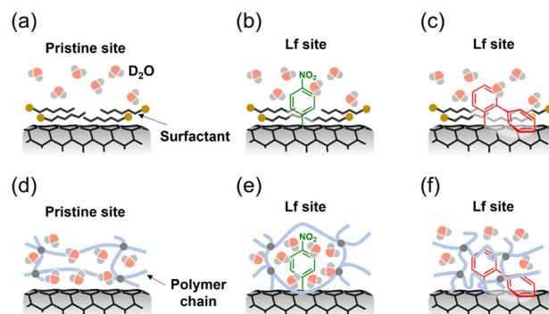
Fig. 3 Schematic diagram around the pristine site and lF site of (a and b) SDBS-dispersed lF-SWCNTs-*p*NO<sub>2</sub>, (a and c) SDS-dispersed lF-SWCNTs-*o*P, (d and e) gel-coated lF-SWCNTs-*p*NO<sub>2</sub> and (d and f) gel-coated lF-SWCNTs-*o*P.
