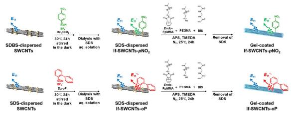
Fig. 1 Synthetic scheme of the gel-coated If-SWCNTs-pNO<sub>2</sub> (upper) and gel-coated If-SWCNTs-oP (lower).
