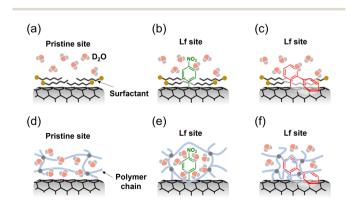
Fig. 3 Schematic diagram around the pristine site and If site of (a and b) SDBS-dispersed If-SWCNTs-pNO<sub>2</sub>, (a and c) SDS-dispersed If-SWCNTs-oP, (d and e) gel-coated lf-SWCNTs-pNO2 and (d and f) gelcoated If-SWCNTs-oP.
