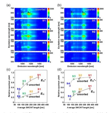
Fig. 6 (a and b) PL mapping and (c and d) relative quantum yield of length-sorted gel-coated lf-SWCNTs-pNO2 and gel-coated lf-SWCNTs-oP, respectively, in H<sub>2</sub>O. Curves are displayed as a guide to the eye. Error bars mean the error estimated during peak deconvolution.
