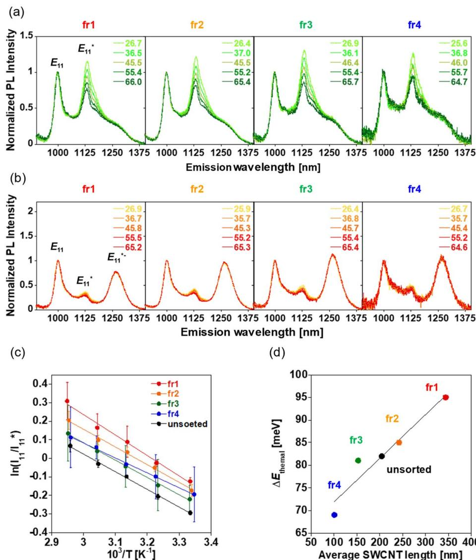
Fig. 7 Temperature-dependent PL spectra (excitation: 570 nm) of the length-sorted (a) gel-coated lf-SWCNTs-*pNO*<sub>2</sub> solution and (b) gel-coated lf-SWCNTs-*oP* solution in H<sub>2</sub>O, (c) the van't Hoff plot of the length-sorted and unsorted gel-coated lf-SWCNTs-*pNO*<sub>2</sub> solution, and (d) plot of  $\Delta E_{\text{thermal}}$  as a function of the average SWCNT length. Error bars mean the error estimated during peak deconvolution.
