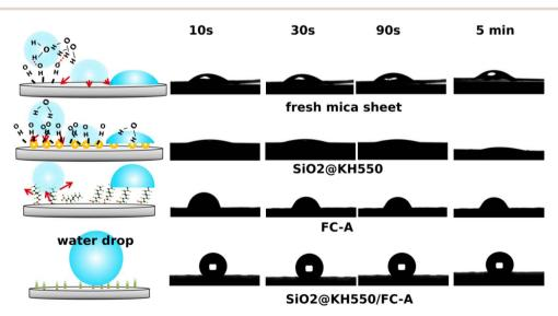
Fig. 8 The stability of water contact angles of mica treated with various fluids.
