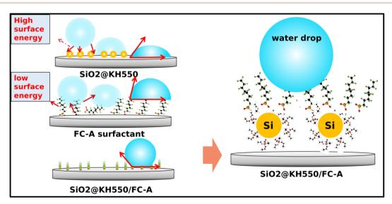
Fig. 15 Schematic illustration of the wettability modification by various fluids.
