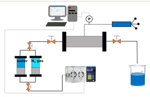
Fig. 3 A diagram of the gas displacement device
