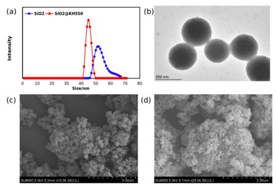
Fig. 6 (a) The particle size distribution for  $SiO_2$  and  $SiO_2$ @KH550. (b) The surface morphology of dispersed  $SiO_2$ @KH550. (c) The surface morphology of  $SiO_2$ . (d) The surface morphology of  $SiO_2$ . (d) The surface morphology of  $SiO_2$ .
