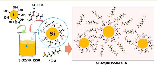
Fig. 2 Schematic diagram of the reaction process of modification of SiO<sub>2</sub>@KH550 and the SiO<sub>2</sub>@KH550/FC-A system.
