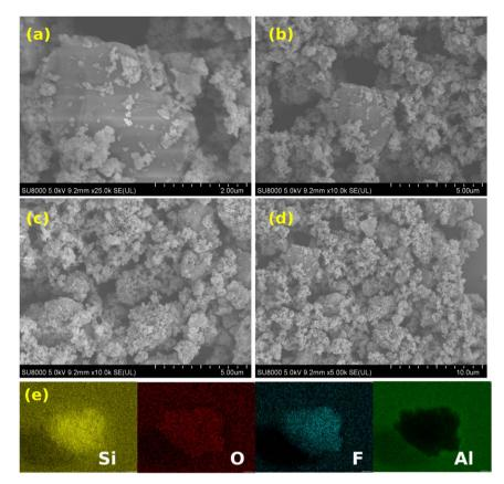
Fig. 9 The surface morphology of a hydrophilic solid treated with (a)  $SiO_2$  (b)  $SiO_2$  (kH550, and (c and d)  $SiO_2$  (kH550/FC-A. (e) SEM mapping images.
