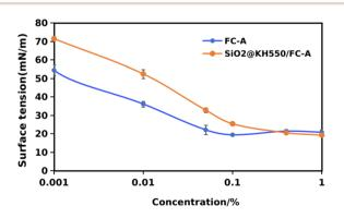
Fig. 10 Surface tensions with different concentrations of FC-A and the  $SiO_2@KH550/FC-A$  composite system.
