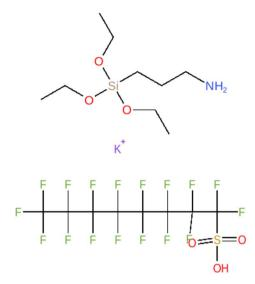
Fig. 1 The chemical structures of KH550 and FC-A
