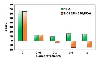
Fig. 11 Variation of  $\sigma\cos\theta$  with different concentrations of FC-A and the SiO<sub>2</sub>@KH550/FC-A composite system.
