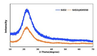
Fig. 5 The XRD patterns of SiO<sub>2</sub> and SiO<sub>2</sub>@KH550.
