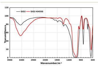
Fig. 4 Fourier-transform infrared (FT-IR) spectra of  $SiO_2$  and  $SiO_2$ @KH550.
