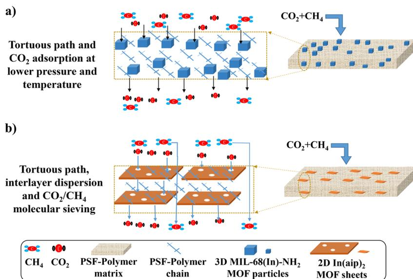
Fig. 1 Illustration of gas separation mechanisms for MMMs in this study, (a) MMM with MIL-68(In)-NH<sub>2</sub> filler and (b) MMM with In(aip)<sub>2</sub> filler.
