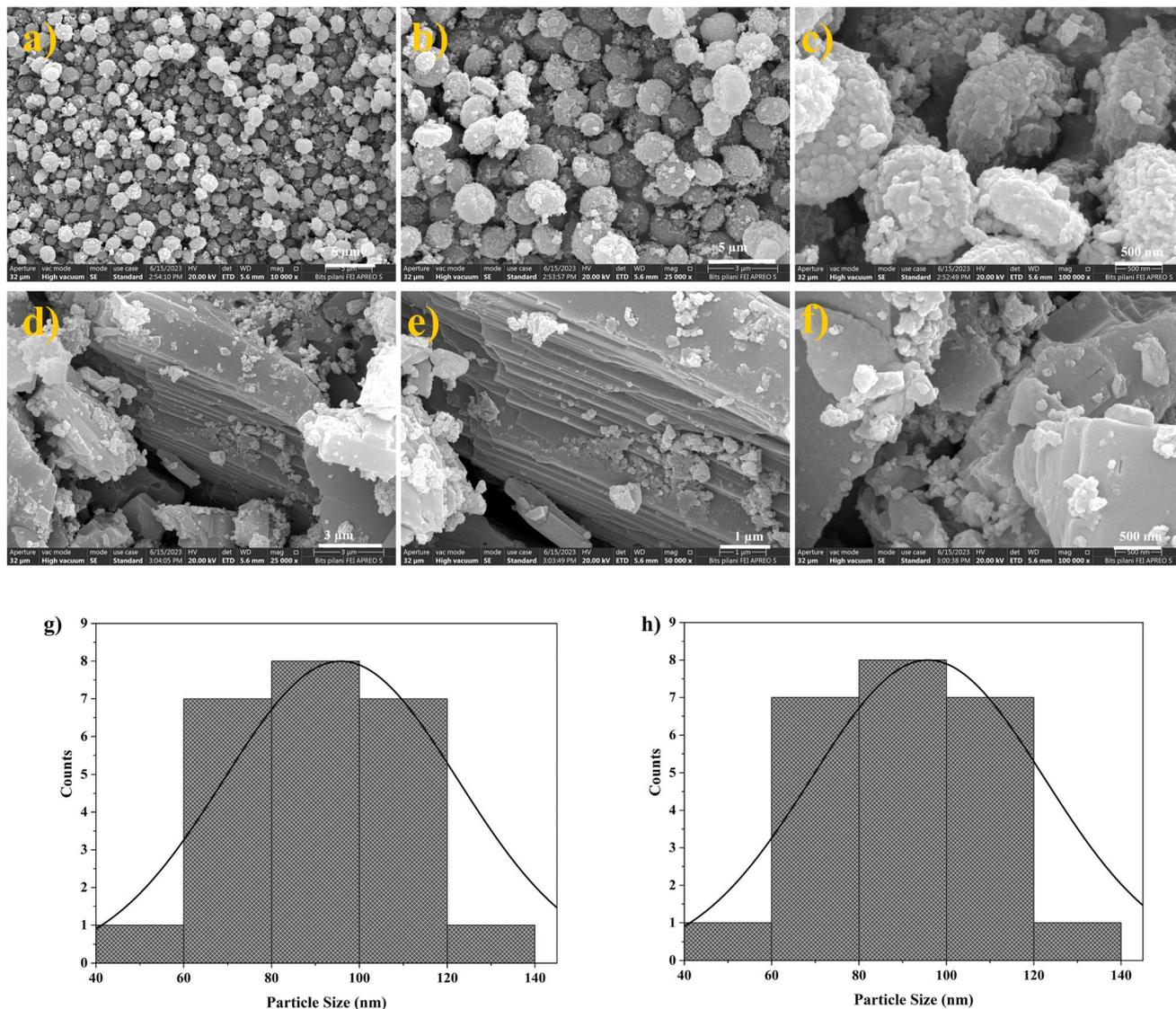
Fig. 4 FESEM images and particle size distribution of (a–c and g) MIL-68(In)-NH<sub>2</sub>, (d–f and h) In(aip)<sub>2</sub>.
