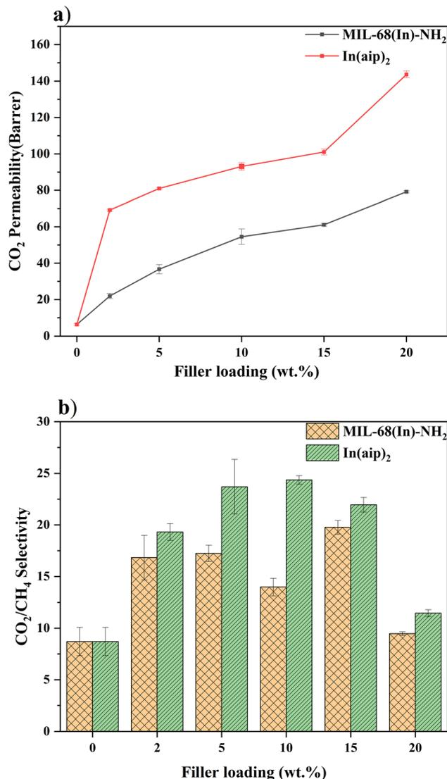
Fig. 6 (a) CO<sub>2</sub> permeabilities and (b) CO<sub>2</sub>/CH<sub>4</sub> selectivities of pure PSF, MIL-68(In)-NH<sub>2</sub>/PSF In(aip)<sub>2</sub>/PSF membranes.
