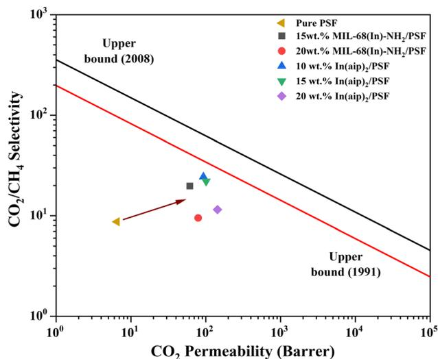
Fig. 8 Status of MIL-68(In)-NH<sub>2</sub>, In(aip)<sub>2</sub> and PSF based MMMs on Robeson plot.
