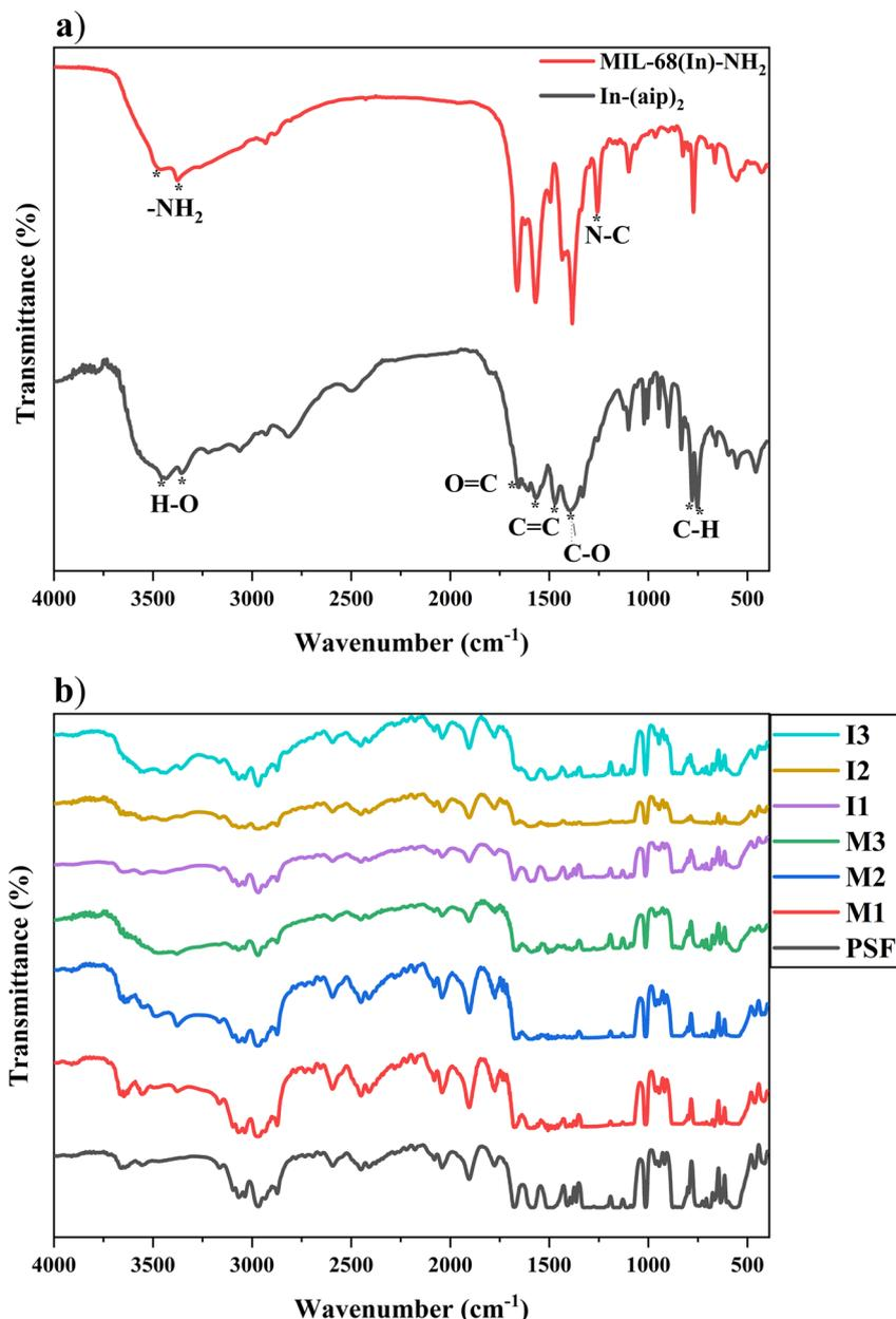
Fig. 3 FTIR of (a) MOFs and (b) membranes.
