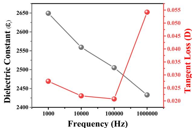
Fig. 8 Dielectric constant ( $\epsilon$ ) and tangent loss ( $D$ ) of sintered barium titanate as a function of frequency. The dielectric constant decreases with increasing frequency, while the tangent loss initially decreases before sharply increasing at higher frequencies.
