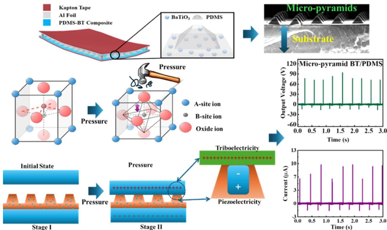
Fig. 13 Schematic illustration of the HBNG nanogenerator with a micro-pyramidal structure, showing the layered composition of Kapton tape, aluminum foil, and PDMS-BaTiO<sub>3</sub> composite. The micro-pyramidal substrate design enhances contact sensitivity, facilitating higher output voltages under mechanical stress.
