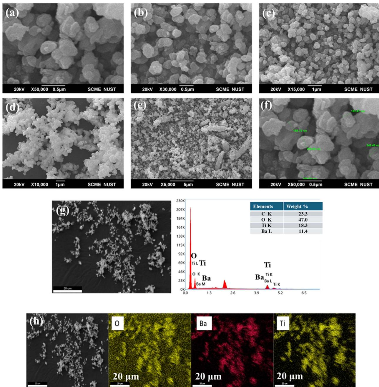
Fig. 5 (a–f) SEM images of barium titanate ( $\text{BaTiO}_3$ ) powder at various magnifications, displaying particle morphology and size distribution. (g) EDS analysis for elemental composition, confirming the presence of Ba, Ti, O, and C in the sample. (h) Elemental mapping images for Ba, Ti, and O, showing uniform distribution of these elements within the  $\text{BaTiO}_3$  powder, indicating consistent material composition.
