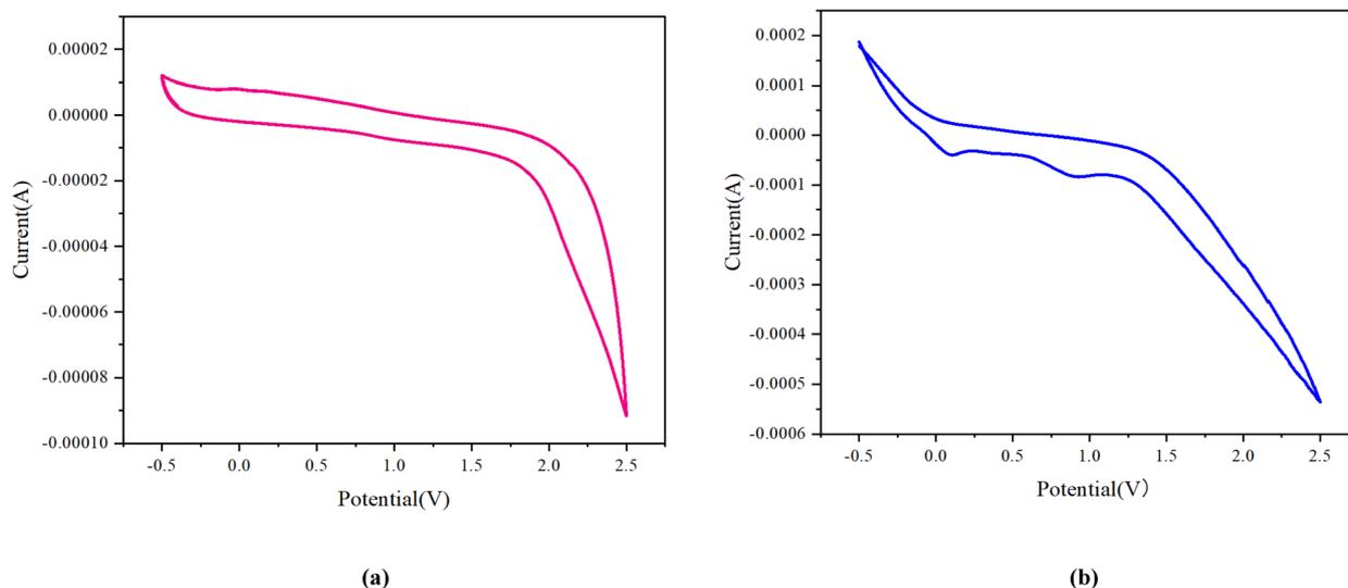
Fig. 5 Electrochemical performance of (a) 1 and (b) 2 in  $\text{CH}_2\text{Cl}_2$  containing 0.1 M  $\text{Bu}_4\text{NPF}_6$  as an electrolyte at 298 K; the scan rate is  $100 \text{ mV s}^{-1}$ .
