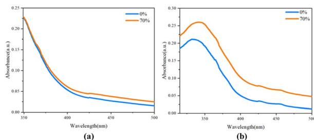
Fig. 2 (a) Ultraviolet (UV) spectroscopy of polymers 1 in different water fractions. (b) Ultraviolet (UV) spectroscopy of polymers 2 in different water fractions (0.05 mg mL<sup>-1</sup> in THF or THF/H<sub>2</sub>O mixture).
