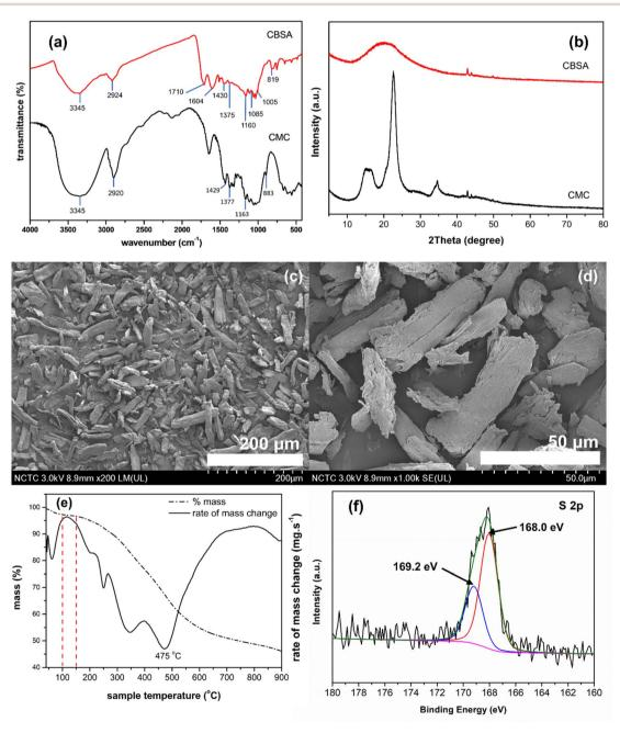
Fig. 1 Catalyst characterization: (a) FTIR spectra of cellulose microcrystals (CMC) and cellulose benzenesulfonic acid (CBSA), (b) PXRD patterns of CMC and CBSA, (c) SEM image of CBSA at  $200 \times \text{magnification}$ , (d) SEM image of CBSA at  $1000 \times \text{magnification}$ , (e) TGA profile of CBSA and, (f) XPS spectrum of CBSA in the S 2p region.
