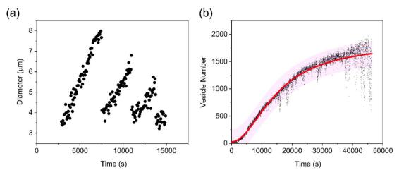
Fig. 2 (a) Diameter of the specific traced vesicle vs. time and (b) vesicle number vs. time curve.
