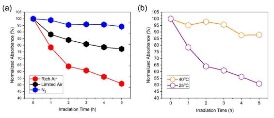
UV-vis studies for the degradation of the 2-sulfur m-RAFT agent (a) at various oxygen levels and (b) at 25 °C and 40 °C
