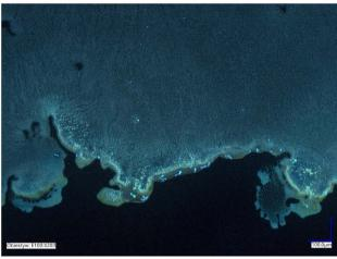
Fig. 2 Picture of the thin layer of compound 1j (top) and 1e (bottom) captured using a digital microscope, illuminated with UV light at a 360–380 nm. The top photograph illustrate crystallization ability of the compound 1j in the thin layer of the solid. The bottom picture was taken at the edge of the layer to better illustrate the continuity of the layer and the limited crystallization ability of the compound 1e in the area where the material accumulates.
