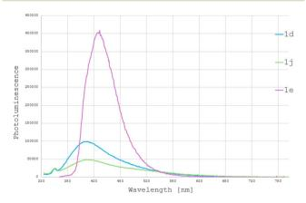
Fig. 1 Emission spectra of selected pyrazoles derivatives.
