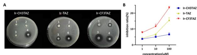
Fig. 2 The inhibitory effect of iridium(III) tetrazolato complexes on bacterial growth in a solid medium. (A) Inhibition ring performance. (1) 1  $\mu\text{M}$ , (2) 10  $\mu\text{M}$ , (3) 100  $\mu\text{M}$ , (4) kanamycin (control) (B) bacteriostatic effect of media with complexes. The inhibition rate was treated with a blank group as control.
