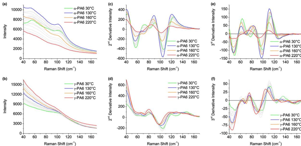
Fig. 3 (a) and (b) Low-frequency Raman spectra of  $\alpha$ - and  $\gamma$ -PA6, respectively, (c) and (d) their second derivative spectra, and (e) and (f) their third derivative spectra as a function of temperature from 30 °C to 220 °C.
