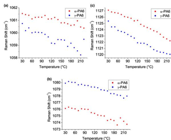
Fig. 6 Plots of the bands at approximately (a)  $1060\text{ cm}^{-1}$ , (b)  $1080\text{ cm}^{-1}$ , and (c)  $1126\text{ cm}^{-1}$  as a function of temperature from  $30\text{ }^\circ\text{C}$  to  $220\text{ }^\circ\text{C}$ .
