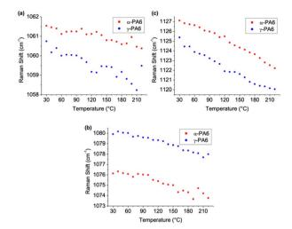
Fig. 6 Plots of the bands at approximately (a)  $1060~\rm cm^{-1}$ , (b)  $1080~\rm cm^{-1}$ , and (c)  $1126~\rm cm^{-1}$  as a function of temperature from 30 °C to 220 °C.
