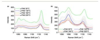
Fig. 5 Raman spectra in C–C stretching regions of (a)  $\alpha$ -PA6 and (b)  $\gamma$ -PA6 as a function of temperature from 30 °C to 230 °C.
