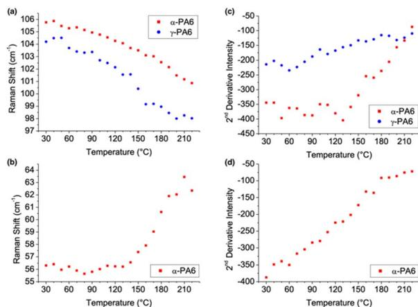
Fig. 4 Raman shift for the bands at approximately (a) 100 cm<sup>-1</sup> and (b) 60 cm<sup>-1</sup>, and the second derivative intensities for the bands at approximately (c) 100 cm<sup>-1</sup> and (d) 60 cm<sup>-1</sup> as a function of temperature from 30 °C to 220 °C.
