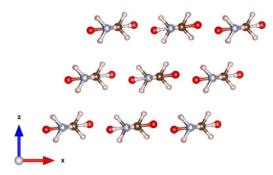
Fig. 1 Unit cell of PA6 in the  $\alpha$ -form used in the calculations.
