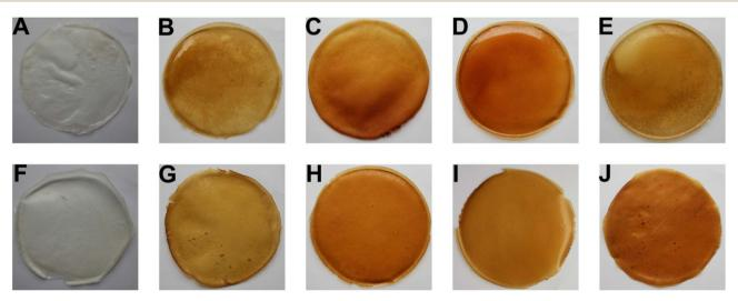
Fig. 2 Photographs of the casein-based films. (A) C, (B) CS50, (C) CS100, (D) CU50, (E) CU100, (F) CT, (G) CS50T, (H) CS100T, (J) CU100T.
