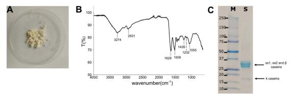
Fig. 1 (A) Photograph of the casein isolated by precipitation after overnight drying at room temperature, (B) FT-IR of casein: relevant signals are highlighted with dotted lines, (C) SDS-PAGE analysis (20%) of isolated proteins from UHT skimmed milk: (M) marker, and (S) isolated sample. Casein bands present in S are pointed with black arrows.
