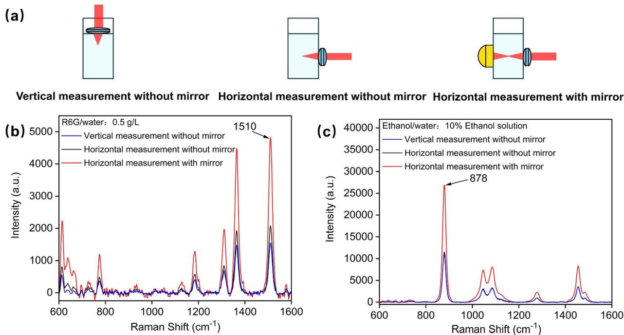
Fig. 3 (a) Comparison of measurement configurations using a 20 mm path length cuvette. (b) Signal enhancement of Rhodamine 6G at  $1510\text{ cm}^{-1}$  under different measurement configurations. (c) Signal enhancement of ethanol at  $878\text{ cm}^{-1}$  under different measurement configurations.
