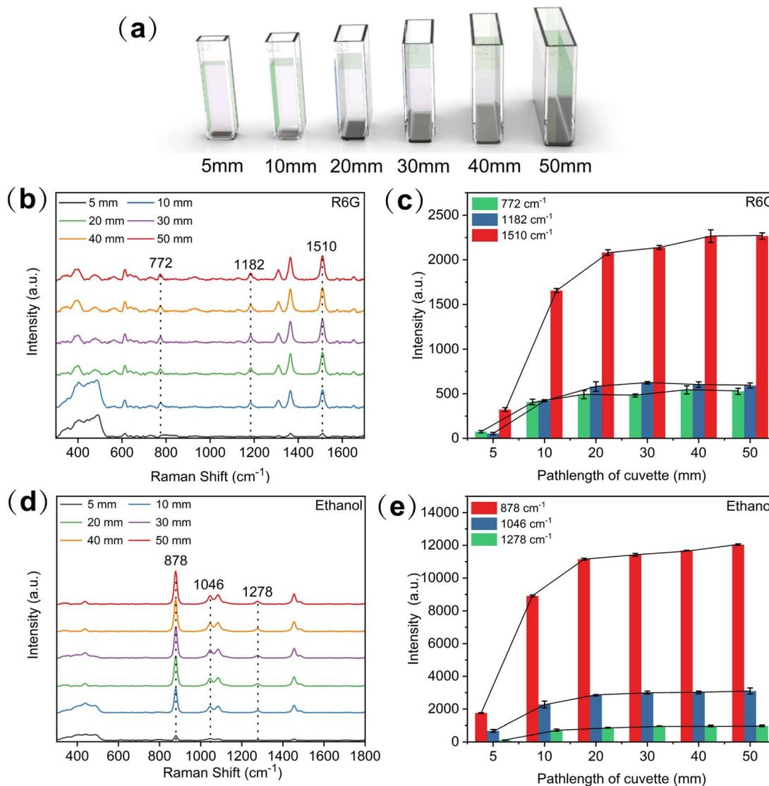
Fig. 2 (a) Schematic diagram of cuvettes with different path lengths. (b) Raman spectrum of Rhodamine 6G in cuvettes with different path lengths. (c) Signal intensity variations of Rhodamine 6G under different cuvette path lengths (d) Raman spectrum of ethanol in cuvettes with different path lengths. (e) Signal intensity variations of ethanol under different cuvette path lengths.
