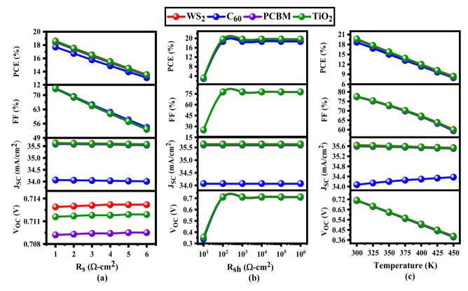
Fig. 13 Impact of photovoltaic (PV) variables (PCE, FF,  $J_{SC}$  and  $V_{OC}$ ) given the modification in (a) series resistance (b) shunt resistance and (c) temperature of Cs<sub>2</sub>CuBiBr<sub>6</sub>.
