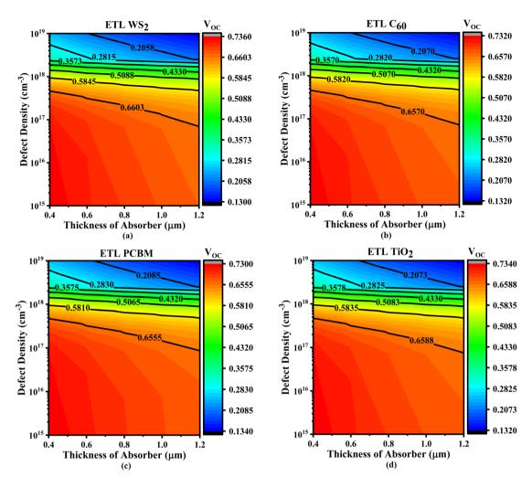
Fig. 8 Contour plots of  $V_{OC}$  resulting from the concurrent variation in defect density and absorber layer thickness with ETLs including (a) WS<sub>2</sub>, (b) C<sub>60</sub>, (c) PCBM, and (d) TiO<sub>2</sub>.
