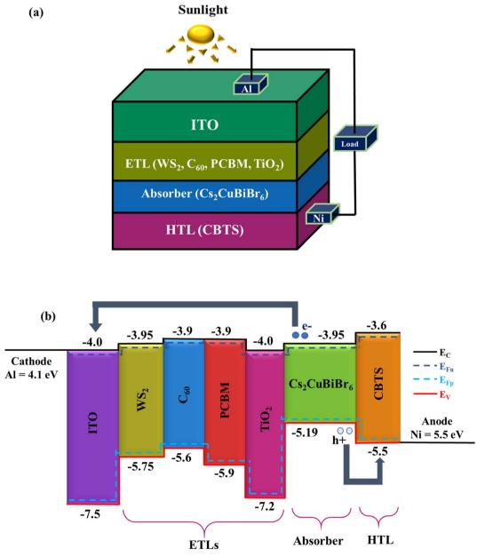
Fig. 2 The  $Cs_2CuBiBr_6$  absorber's (a) crystal arrangement and (b) energy band aligning associated with various ETL materials (WS<sub>2</sub>,  $C_{60}$ , PCBM, and TiO<sub>2</sub>).
