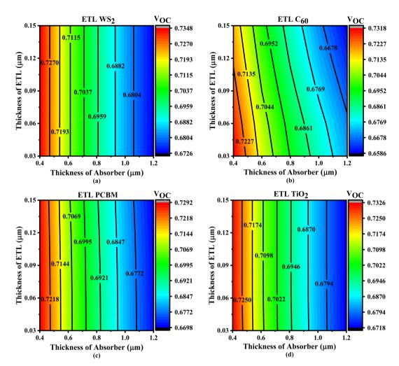
Fig. 4 Contour plots of  $V_{\rm OC}$  resulting from the sequential change in absorber layer thickness and ETL layer thickness with ETLs including (a) WS<sub>2</sub>, (b) C<sub>60</sub>, (c) PCBM, and (d) TiO<sub>2</sub>.
