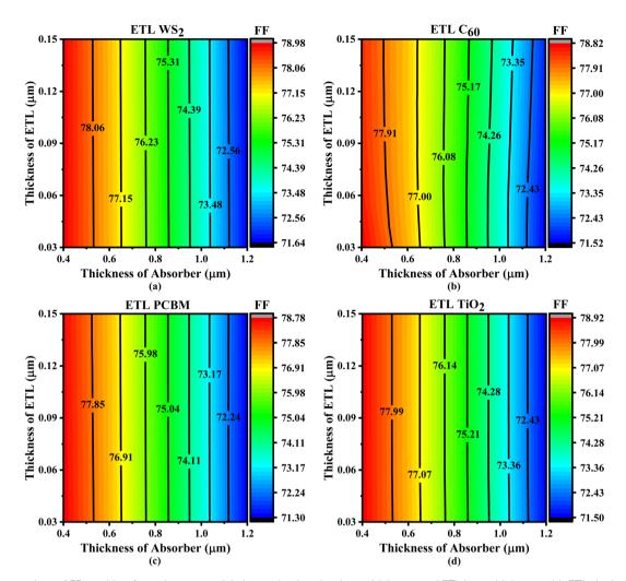
Fig. 6 Contour plots of FF resulting from the sequential change in absorber layer thickness and ETL layer thickness with ETLs including (a) WS<sub>2</sub>, (b)  $C_{60}$ , (c) PCBM, and (d)  $TiO_2$ .
