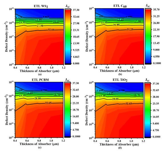
Fig. 9 Contour plots of  $J_{SC}$  resulting from the concurrent variation in defect density and absorber layer thickness with ETLs including (a) WS<sub>2</sub>, (b) C<sub>60</sub>, (c) PCBM, and (d) TiO<sub>2</sub>.
