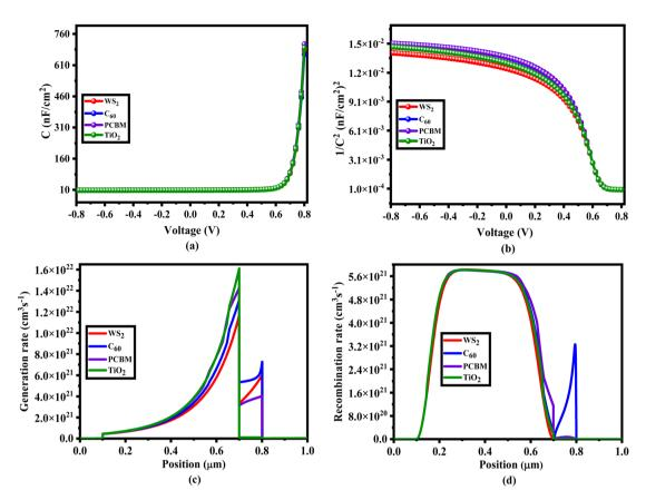
Fig. 14 Distinctions in (a) capacitance (b) Mott-Schottky (c) generation and (d) recombination of Cs<sub>2</sub>CuBiBr<sub>6</sub>.
