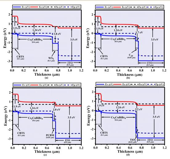
Fig. 3 Band diagram containing (a) WS<sub>2</sub>, (b) C<sub>60</sub>, (c) PCBM, and (d) TiO<sub>2</sub> for Cs<sub>2</sub>CuBiBr<sub>6</sub>.
