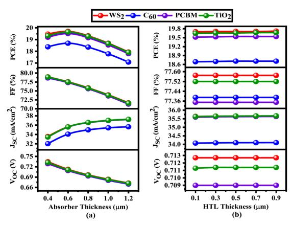
Fig. 12 Impact of photovoltaic (PV) variables (PCE, FF,  $J_{SC}$  and  $V_{OC}$ ) given the modification in (a) absorber thickness and (b) HTL thickness of Cs2CuBiBr6.
