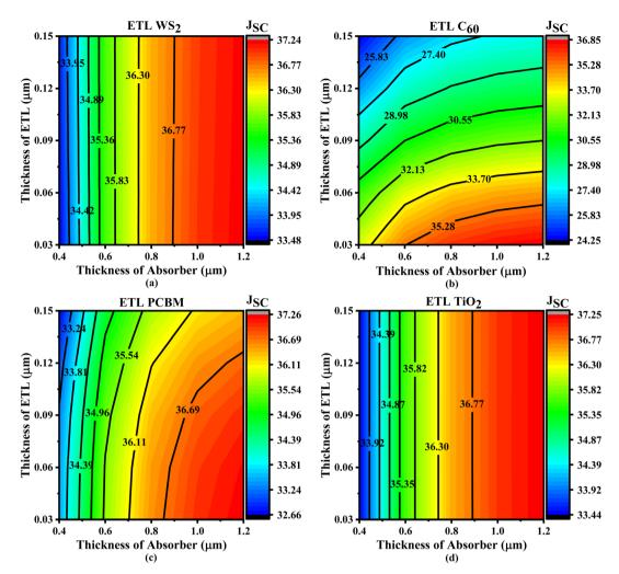
Fig. 5 Contour plots of  $J_{SC}$  resulting from the sequential change in absorber layer thickness and ETL layer thickness with ETLs including (a) WS<sub>2</sub>, (b) C<sub>60</sub>, (c) PCBM, and (d) TiO<sub>2</sub>.
