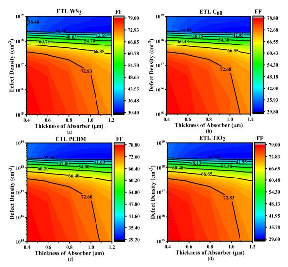
Fig. 10 Contour plots of FF resulting from the concurrent variation in defect density and absorber layer thickness with ETLs including (a)  $WS_2$ , (b)  $C_{60}$ , (c) PCBM, and (d)  $TiO_2$ .
