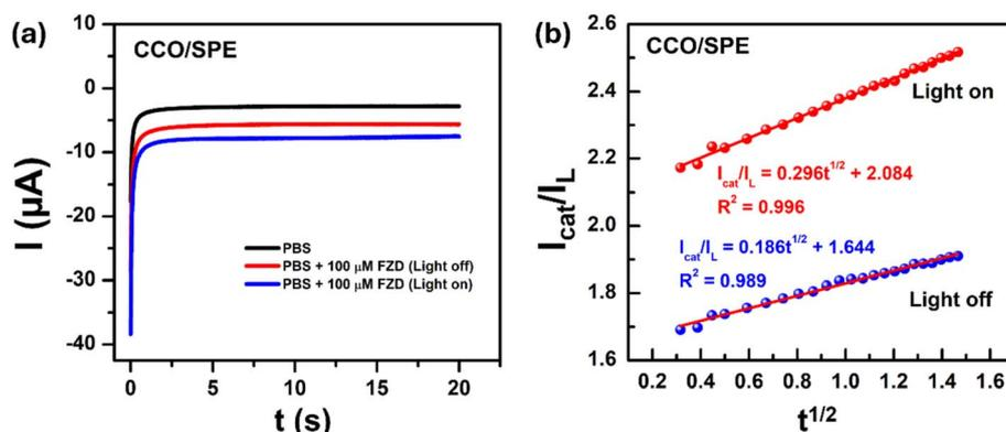
Fig. 7 (a) Chronoamperometric curves of the CCO/SPE in the absence and presence of  $100 \mu\text{M}$  FZD in  $0.1 \text{ M}$  PBS solution under turn on and off light conditions; (b) the plot of  $I_{\text{cat}}/I_{\text{L}}$  vs.  $t^{1/2}$  obtained from the chronoamperograms.
