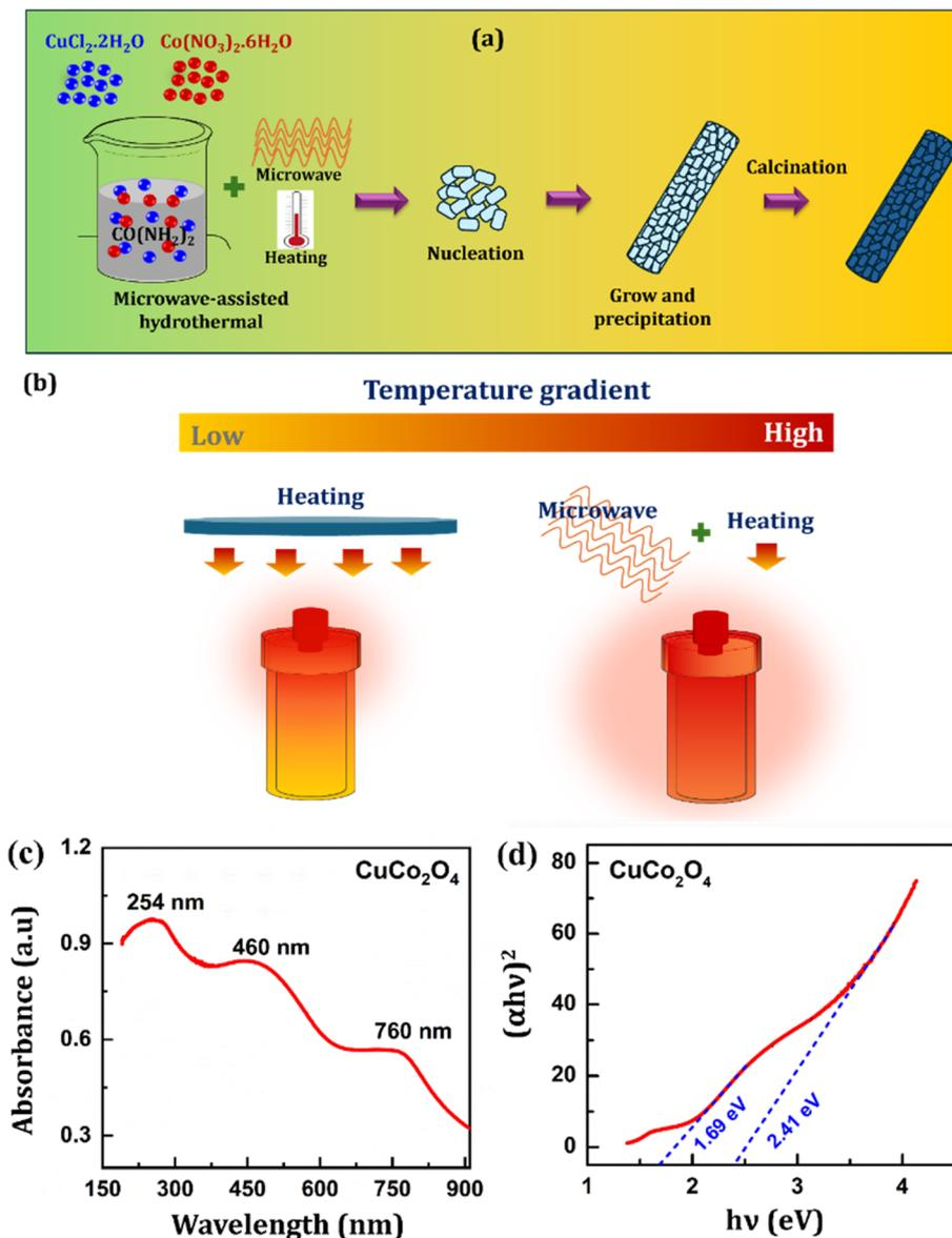
Fig. 2 (a) Schematic representation for the formation mechanism  $\text{CuCo}_2\text{O}_4$  nanorods, and (b) comparison of conductive and microwave heating process, (c) UV-Vis absorption spectra, and (d) the Tauc plot and optical band gap values of  $\text{CuCo}_2\text{O}_4$  nanorods.
