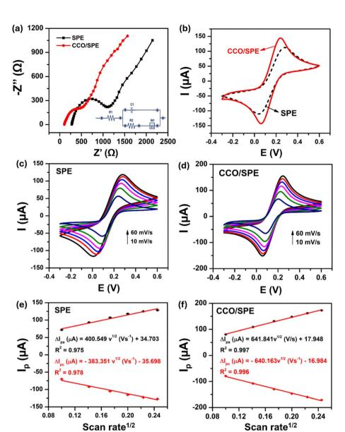
Fig. 3 Nyquist plot (a) and CV profiles (b) of pure SPE, and CCO-modified SPE electrode. (c-f) CV curves recorded on SPE and CCO/SPE in 0.1 M KCl containing 5 mM  $K_3$ [Fe(CN)<sub>6</sub>] and  $K_4$ [Fe(CN)<sub>6</sub>] at different scan rates, corresponding to the linear graphs of peak current response ( $l_{pa}$ ,  $l_{pc}$ ) versus  $\nu^{1/2}$  with error bars.
