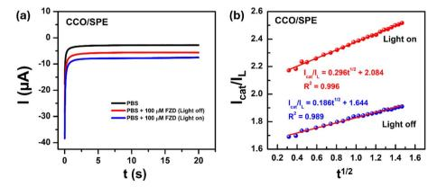
Fig. 7 (a) Chronoamperometric curves of the CCO/SPE in the absence and presence of 100 μM FZD in 0.1 M PBS solution under turn on and off light conditions; (b) the plot of  $I_{cat}/I_L$  vs.  $t^{1/2}$  obtained from the chronoamperograms.
