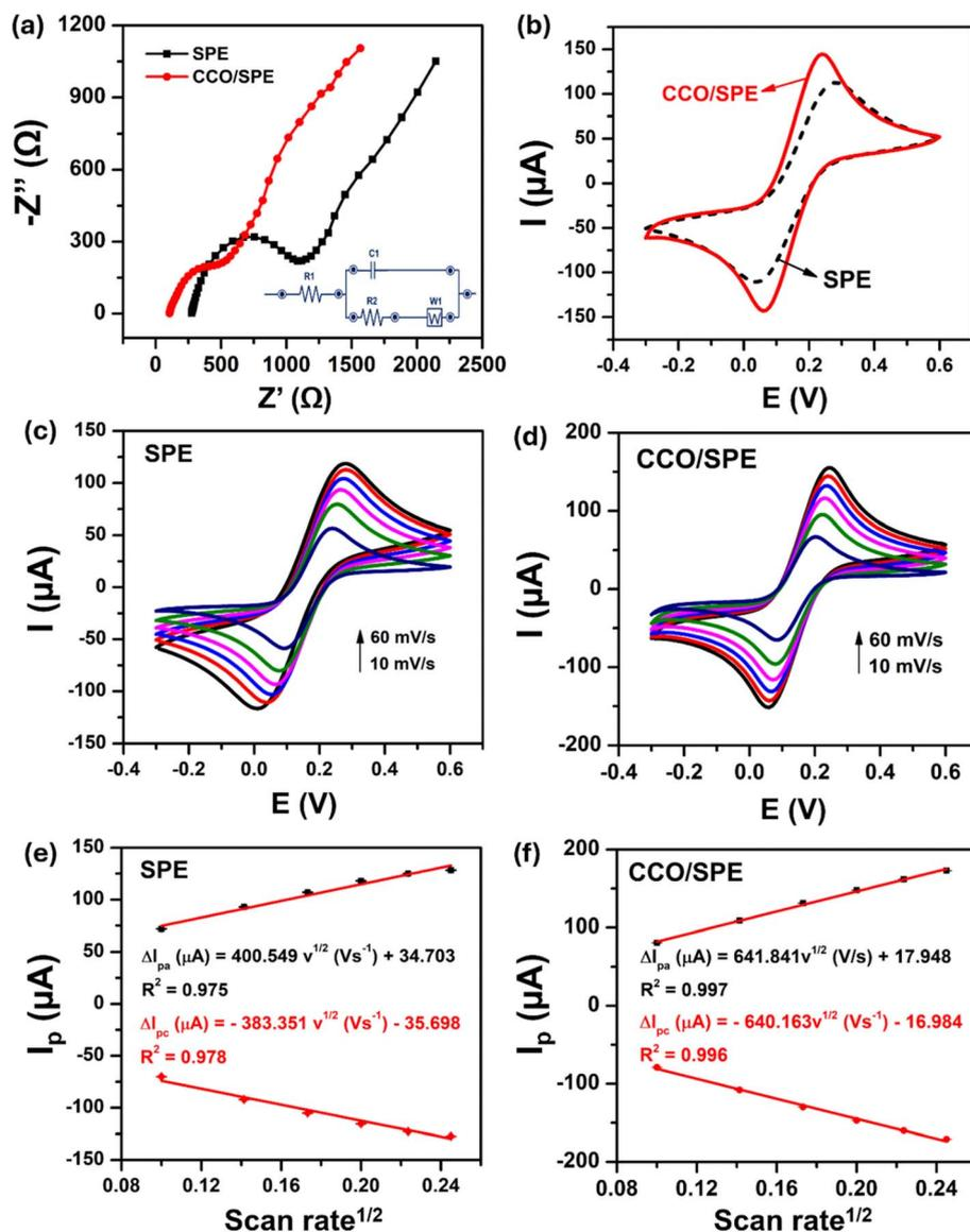
Fig. 3 Nyquist plot (a) and CV profiles (b) of pure SPE, and CCO-modified SPE electrode. (c–f) CV curves recorded on SPE and CCO/SPE in 0.1 M KCl containing 5 mM  $\text{K}_3[\text{Fe}(\text{CN})_6]$  and  $\text{K}_4[\text{Fe}(\text{CN})_6]$  at different scan rates, corresponding to the linear graphs of peak current response ( $I_{pa}$ ,  $I_{pc}$ ) versus  $v^{1/2}$  with error bars.
