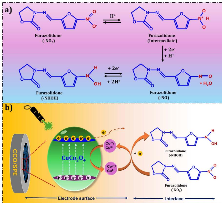
Fig. 9 (a) The electrochemical reduction mechanism of FZD, and (b) the enhancement mechanism of CuCo<sub>2</sub>O<sub>4</sub>-based photoelectrochemical sensor for detection of FZD under green light irradiation.
