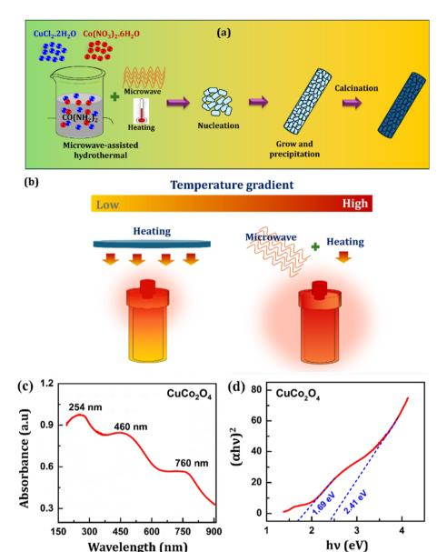
Fig. 2 (a) Schematic representation for the formation mechanism  $CuCo_2O_4$  nanorods, and (b) comparison of conductive and microwave heating process, (c) UV-Vis absorption spectra, and (d) the Tauc plot and optical band gap values of  $CuCo_2O_4$  nanorods.
