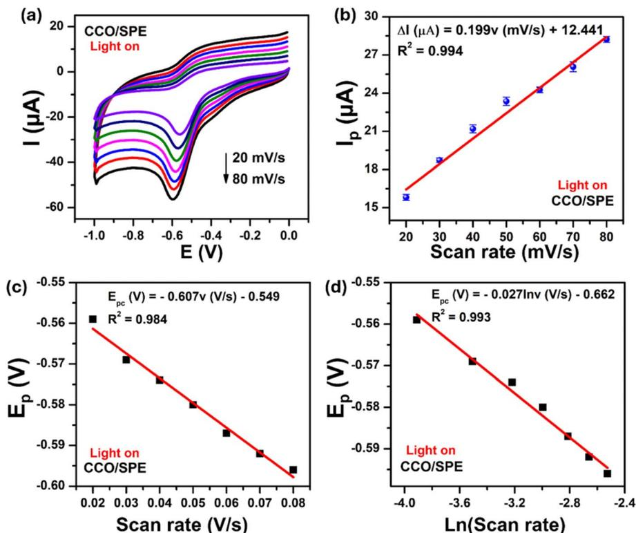
Fig. 6 (a) CV voltammograms of CCO/SPE in 0.1 M PBS (pH 7.3) containing 200  $\mu\text{M}$  FZD at various scan rates from 20 to 80  $\text{mV s}^{-1}$ , (b) a linear relationship between electro-reduction peak current and scan rate, (c) linear graph for scan rate versus  $E_{\text{pc}}$ , and (d) the plot of  $E_{\text{pc}}$  with the natural logarithm of scan rate  $[\ln(\nu)]$  in the presence of light-assisted.
