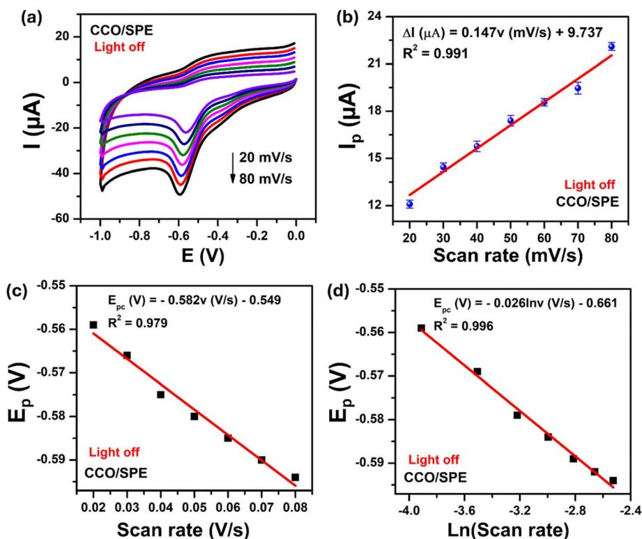
Fig. 5 (a) CV curves of CCO/SPE were recorded in 0.1 M PBS (pH 7.3) containing 200  $\mu\text{M}$  FZD, (b) linear plot for scan rate vs. FZD electro-reduction peak current, (c) linear graph for scan rate versus FZD electro-reduction peak potential ( $E_{pc}$ ), and (d) the plot of  $E_{pc}$  with the natural logarithm of scan rate [ $\ln(\nu)$ ].
