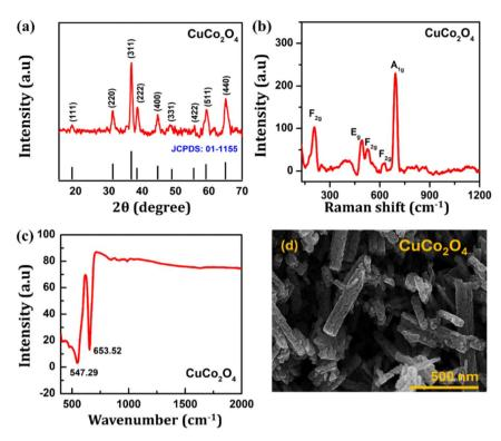
Fig. 1 (a) XRD pattern, (b) Raman spectrum, (c) FTIR spectra, and (d) SEM micrographs of CuCo<sub>2</sub>O<sub>4</sub> nanorods.
