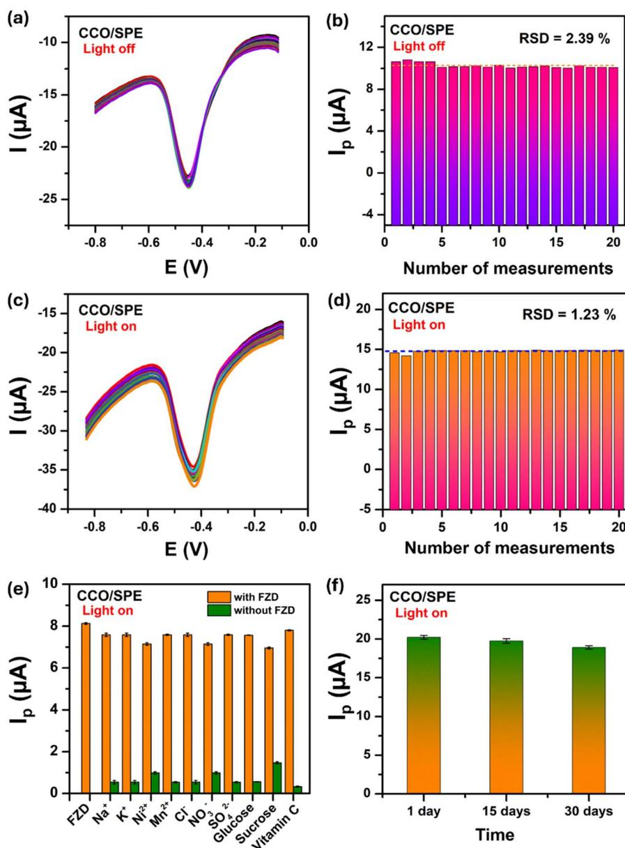
**Fig. 10** The repeatability of CCO/SPE in 0.1 M PBS (pH 7.0) containing 100  $\mu\text{M}$  FZD without (a and b) and with (c and d) of green light; (e) the anti-interfering capability in 0.1 M PBS containing 50  $\mu\text{M}$  FZD and 1000  $\mu\text{M}$  interfering substances in the assistance of green light; (f) the stability in 30 days with green light irradiation condition. The error bars denote the standard deviations from three independent experiments.
