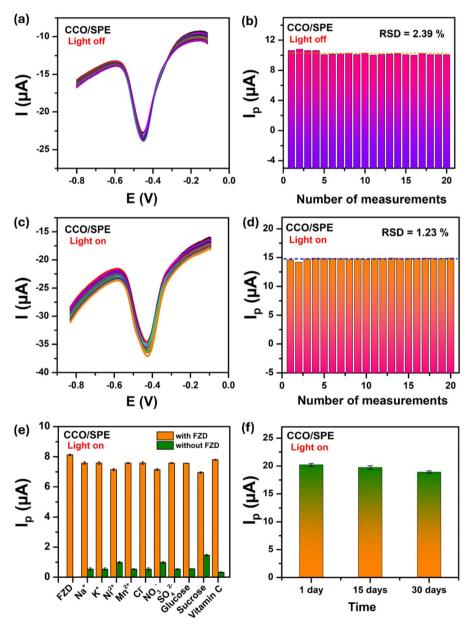
Fig. 10 The repeatability of CCO/SPE in 0.1 M PBS (pH 7.0) containing  $100 \mu M$  FZD without (a and b) and with (c and d) of green light; (e) the anti-interfering capability in 0.1 M PBS containing  $50 \mu M$  FZD and  $1000 \mu M$  interfering substances in the assistance of green light; (f) the stability in 30 days with green light irradiation condition. The error bars denote the standard deviations from three independent experiments.
