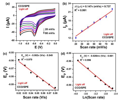
Fig. 5 (a) CV curves of CCO/SPE were recorded in 0.1 M PBS (pH 7.3) containing 200  $\mu$ M FZD, (b) linear plot for scan rate vs. FZD electro-reduction peak current, (c) linear graph for scan rate versus FZD electro-reduction peak potential ( $E_{pc}$ ), and (d) the plot of  $E_{pc}$  with the natural logarithm of scan rate [ $\ln(v)$ ].
