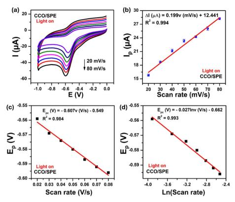
Fig. 6 (a) CV voltammograms of CCO/SPE in 0.1 M PBS (pH 7.3) containing 200  $\mu$ M FZD at various scan rates from 20 to 80 mV s<sup>-1</sup>, (b) a linear relationship between electro-reduction peak current and scan rate, (c) linear graph for scan rate *versus*  $E_{pc}$ , and (d) the plot of  $E_{pc}$  with the natural logarithm of scan rate  $|In(\nu)|$  in the presence of light-assisted.
