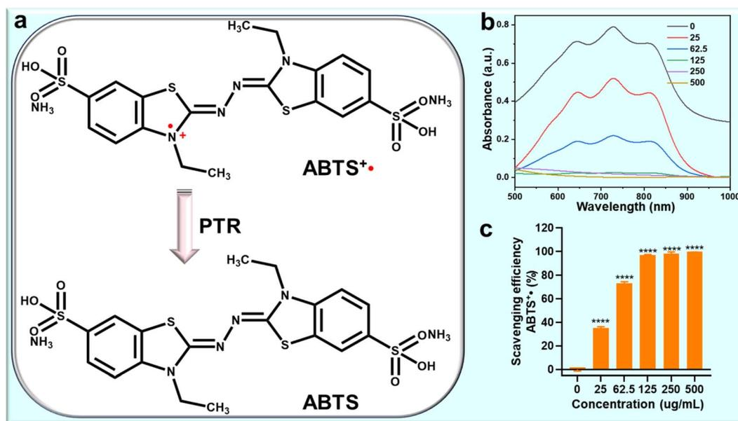
Fig. 3 Free radical scavenging  $\text{ABTS}^{+\cdot}$  assays of PTR NPs: (a) a schematic illustration depicting the  $\text{ABTS}^{+\cdot}$  radical scavenging process. (b) UV-vis spectra of  $\text{ABTS}^{+\cdot}$  radicals after incubation with varying concentration gradients of PTR NPs. (c) Quantitative analysis of  $\text{ABTS}^{+\cdot}$  radical scavenging effects of PTR NPs at different concentrations.
