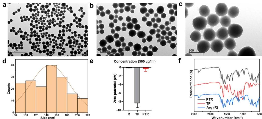
Fig. 2 Nanoparticle size and surface characteristics: TEM images of PTR nanoparticles at low, medium, and high magnifications, (a) scale bar: 1  $\mu\text{m}$ , (b) scale bar: 500 nm, (c) scale bar: 200 nm. (d) Particle size distribution chart of PTR NPs,  $d = 146.8 \pm 37.67$  nm. (e) Zeta potential of PTR NPs. (f) FTIR spectrum of PTR NP, TP, Arg (R).
