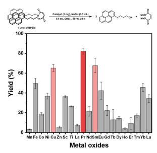
Fig. 3 Comparative fluorescence yields from transesterification using transition or lanthanide metal oxide catalysts with this HTS method.
