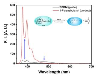
Fig. 1 Comparison of fluorescence spectra between BPBM (pyrene excimer probe) and 1-pyrenebutanol (transesterification product).
