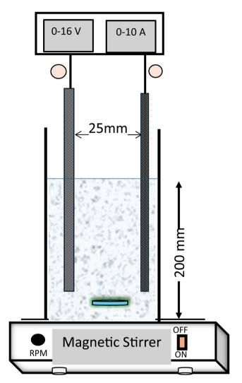
Fig. 1 Experimental setup for electrocoagulation treatment.
