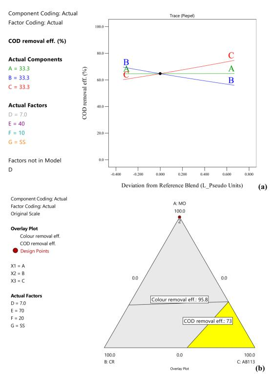
Fig. 3 Effect of dye concentrations on COD removal efficiency of dye mixtures with stainless steel electrodes at pH = 7, 70 A m $^{-2}$  and 20 min treatment time using (a) trace plots and (b) overlay plots (A, B, C = dye concentration, D = pH, E = current density, F = treatment time, G = electrode pair).
