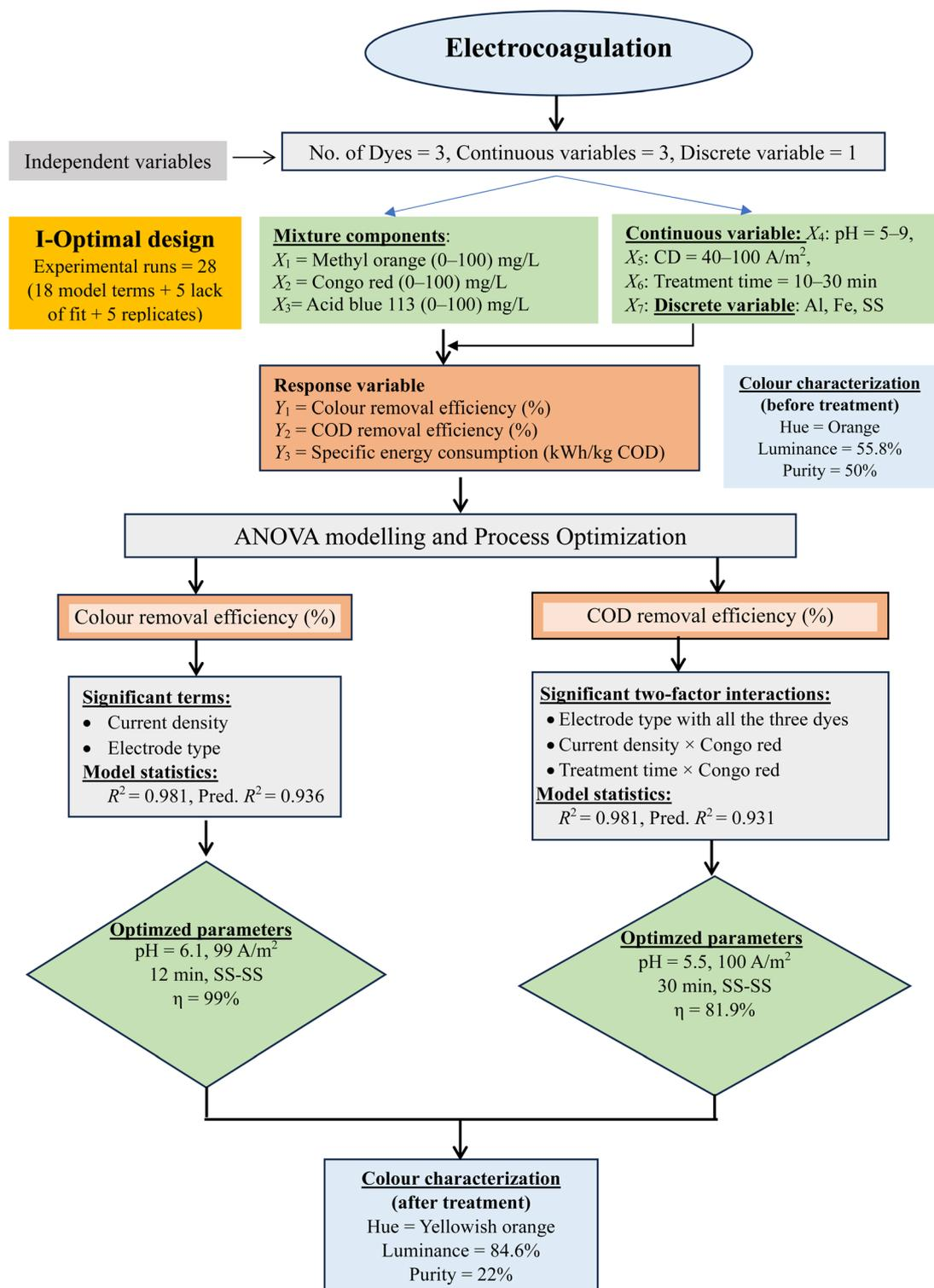
**Fig. 4** Flow chart for electrocoagulation treatment of ternary dye mixture.
