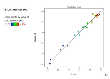
Fig. 2 Normal percentage probability plot and (b) actual vs. predicted plot for COD removal efficiency of dye mixtures after log transformation.
