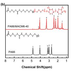
Fig. 2 FTIR spectra (a) and <sup>1</sup>H-NMR spectra (b) of PA66 and PA66/MACM6 copolymers.
