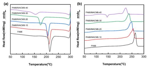
Fig. 4 DSC curves of PA66 and PA66/MACM6 copolymers during the first cooling (a) and the second heating (b) process at a rate of 10 °C min<sup>-1</sup>.
