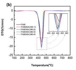
Fig. 3 TGA curves (a) and DTG curves (b) of PA66 and PA66/MACM6 copolymers.
