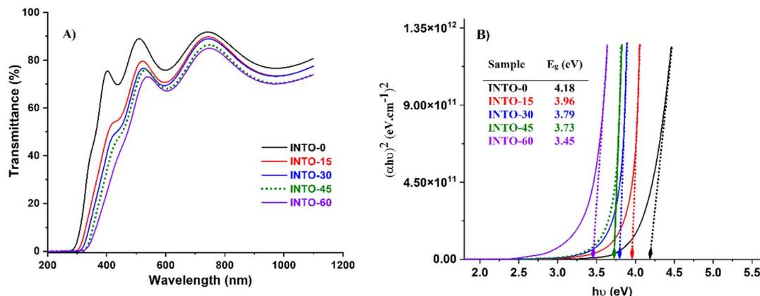
Fig. 7 Transmittance spectra (A) and bandgap energy (B) of INTO- $x$  films deposited on quartz substrates at 300 °C and  $10^{-3}$  torr, with different percentages of  $N_2$  in a mixed sputtering gas.
