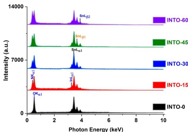
Fig. 1 EDX spectra of INTO-*x* films deposited on silicon substrates at 300 °C and 10<sup>−3</sup> torr, with different percentages of N<sub>2</sub> in a mixed sputtering gas.
