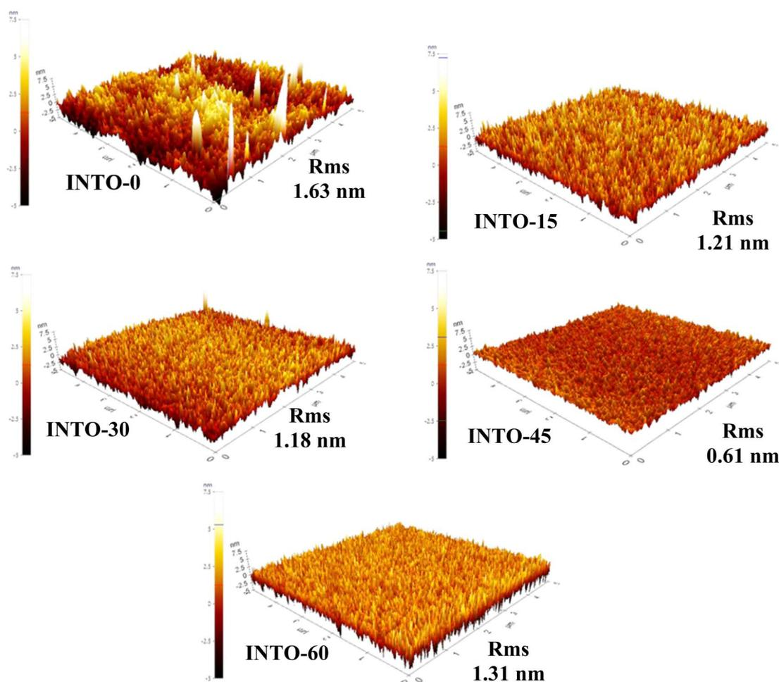
**Fig. 6** AFM images of INTO-*x* films deposited on quartz substrates at 300 °C and 10<sup>-3</sup> torr, with different percentages of N<sub>2</sub> in a mixed sputtering gas.
