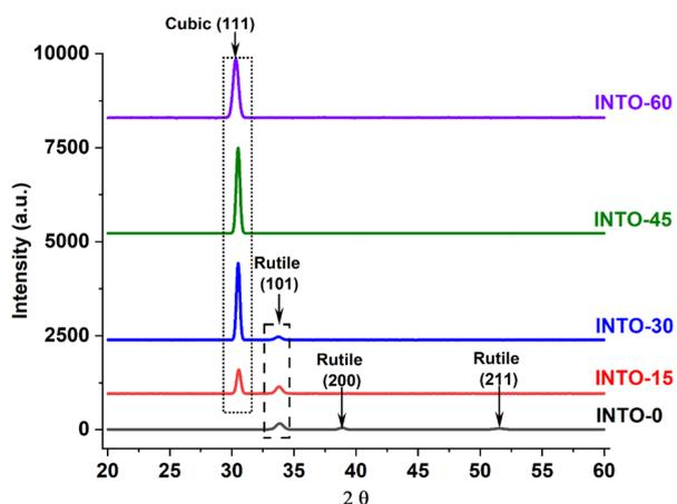
**Fig. 4** XRD patterns of INTO-*x* films deposited on quartz substrates at 300 °C and 10<sup>-3</sup> torr, with different percentages of N<sub>2</sub> in a mixed sputtering gas.
