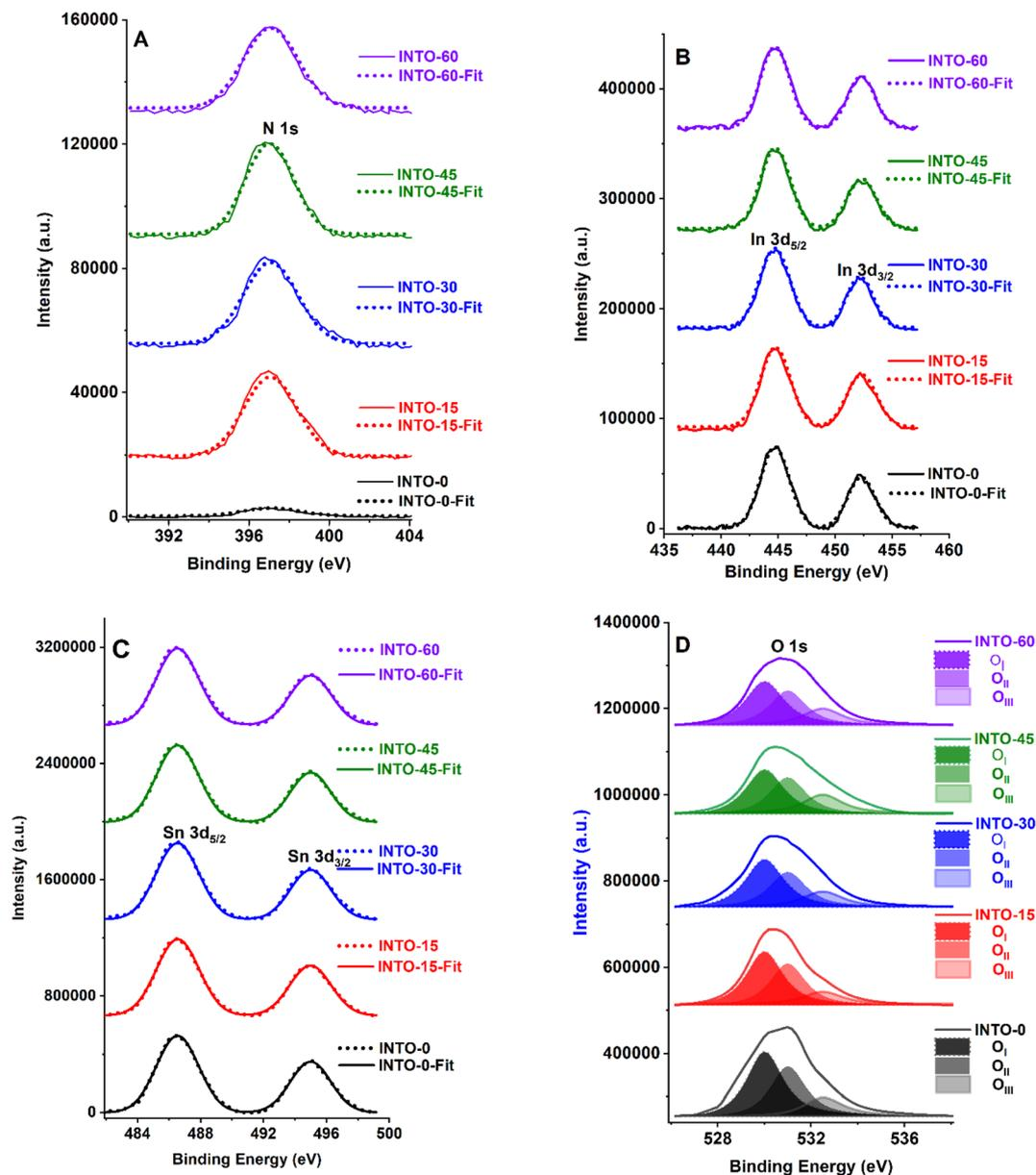
Fig. 3 XPS spectra of INTO-*x* films deposited on quartz substrates at 300 °C and 10<sup>-3</sup> torr, with different percentages of N<sub>2</sub> in a mixed sputtering gas.
