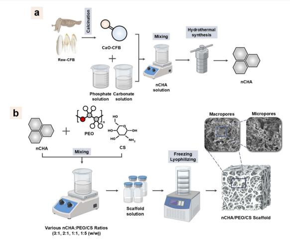
Fig. 1 Schematic methods for (a) the nCHA synthesis and (b) nCHA/PEO/CS scaffold fabrication.
