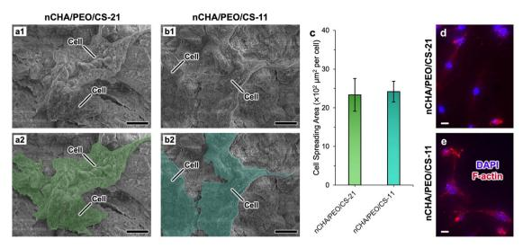
Fig. 10 Morphology of adherent MC3T3-E1 cells on the surfaces of (a1) nCHA/PEO/CS-21 and (b1) nCHA/PEO/CS-11 scaffolds. (a2 and b2) Cells highlighted in the panels a1 and b1. (c) Cell spreading area on the surfaces of nCHA/PEO/CS-21 and nCHA/PEO/CS-11 scaffolds. Cytoskeleton of adherent cells on (d) nCHA/PEO/CS-21 and (e) nCHA/PEO/CS-11 scaffold surfaces. Scale bars: 20 μm (a1-b2,d,e).
