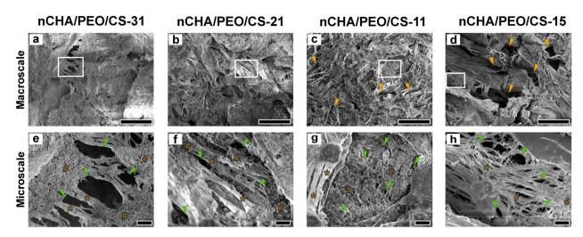
Fig. 5 Morphologies of the nCHA/PEO/CS scaffolds in (a–d) macro- and (e–h) microscale. The characters "#," "\*," orange and green arrowheads indicate nCHA, PEO/CS fibrous network, macropores, and micropores, respectively. Scale bars: 100 µm (a–d) and 10 µm (e–h).
