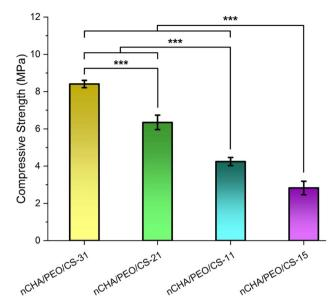
Fig. 6 Compressive strengths of the nCHA/PEO/CS scaffolds. \*\*\*p < 0.001.
