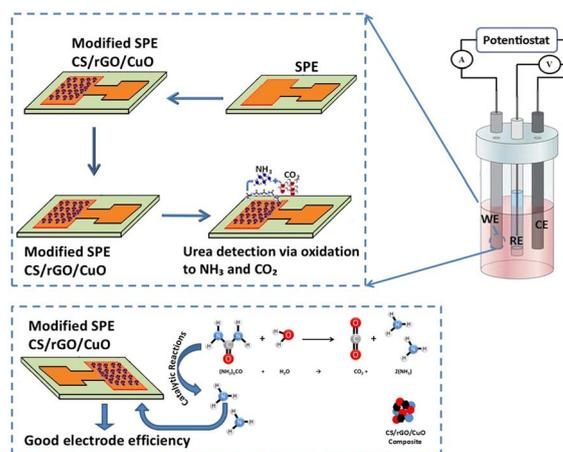
Fig. 11 Schematic of the reaction mechanism of urea fertilizer detection using CS/rGO/CuO-modified SPE.<sup>36</sup>
