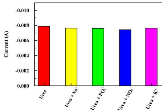
Fig. 12 Interference bar graph of the CS/rGO/CuO-modified SPE electrode.
