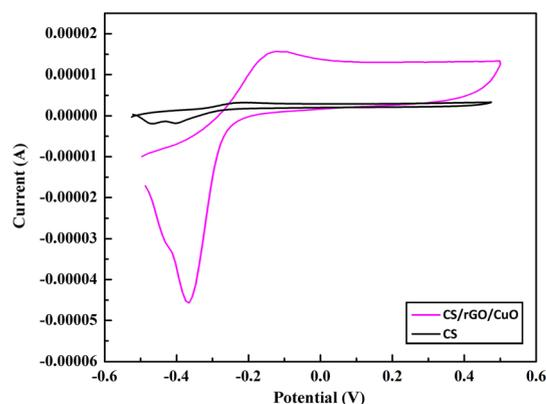
Fig. 5 CV voltammograms of electrodes modified with CS/rGO/CuO and CS and then dipped in a PBS solution with a pH of 7 at a scan rate of  $100$  mV s<sup>-1</sup>.
