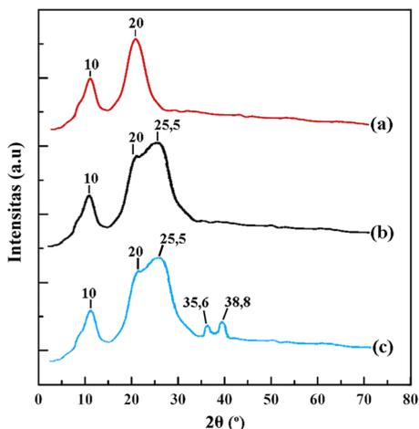
Fig. 3 XRD diffractograms of CS (a), CS/rGO (b) and CS/rGO/CuO.
