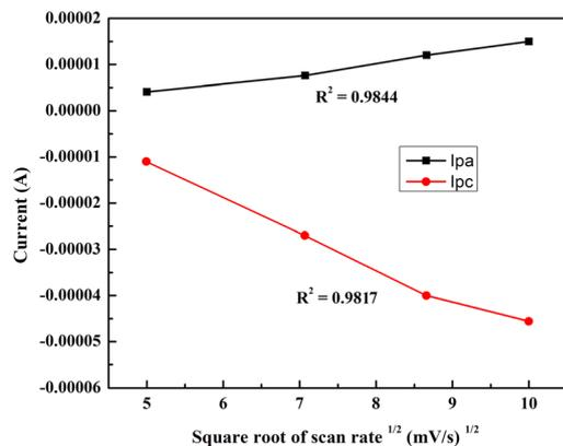
Fig. 7 The effect of scan rate on the anodic (and cathodic) peak current is presented, with the inset showing a linear fit of peak current versus the square root of the scan rate, indicating a diffusion-controlled process.
