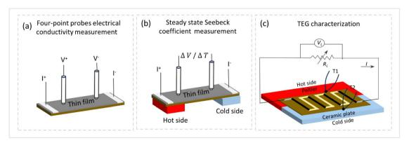
Fig. 2 Schematic illustration of (a) electrical resistance measurement. (b) Seebeck coefficient measurement, and (c) TEG characterization setup.
