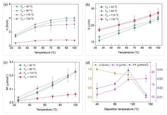
Fig. 4 Temperature dependency of (a) electrical conductivity, (b) Seebeck coefficient, and (c) power factor of the thin films printed at different substrate temperatures ( $T_D$ ). (d) The variation of electrical conductivity, Seebeck coefficient, and power factor with deposition temperature. The error bars were calculated by two times repetition of measurements on each sample.
