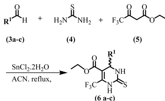
Scheme 1 DHPM-thiones (6a–c) synthesis through Biginelli reaction.
