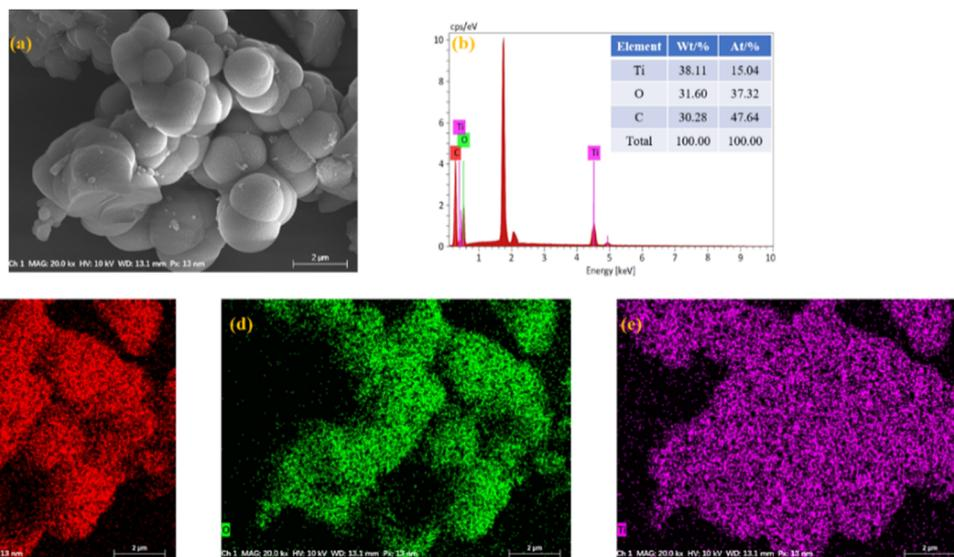
Fig. 6 (a) An FESEM photograph and (b–e) EDS analysis of titanium adipate.
