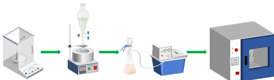
Fig. 2 A diagram of the devices used to prepare the titanium adipate catalyst.
