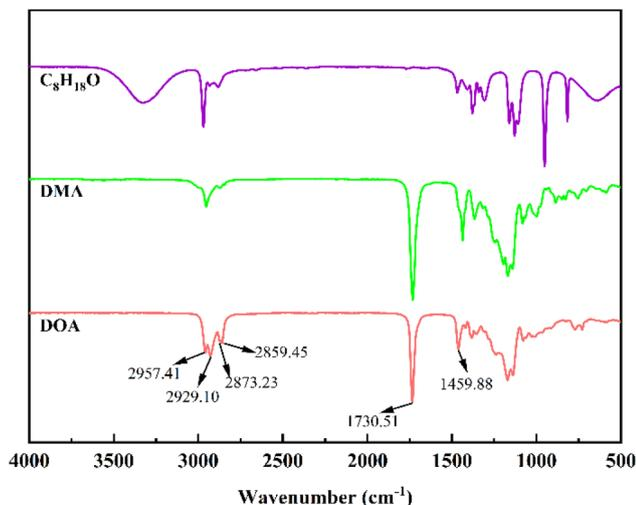
Fig. 8 The FT-IR spectrum of DOA, with DMA and isoctanol shown for reference.
