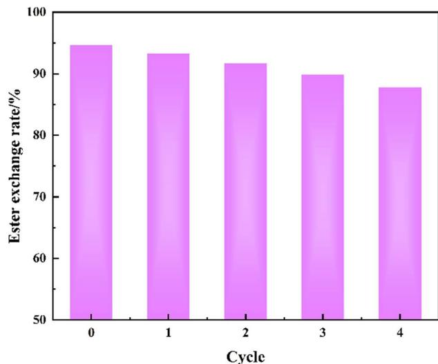
Fig. 14 Effects of the reuse of the catalyst.
