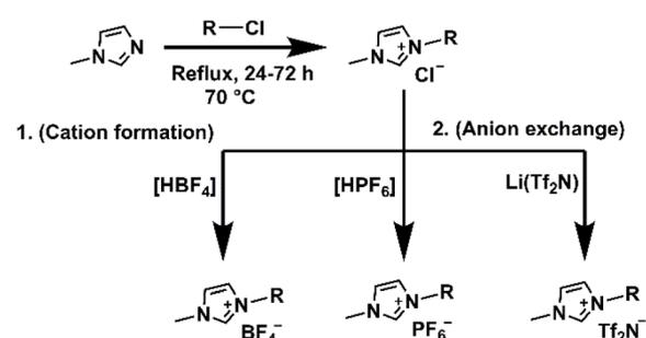
Fig. 6 Synthesis of ionic liquids using methylimidazole.
