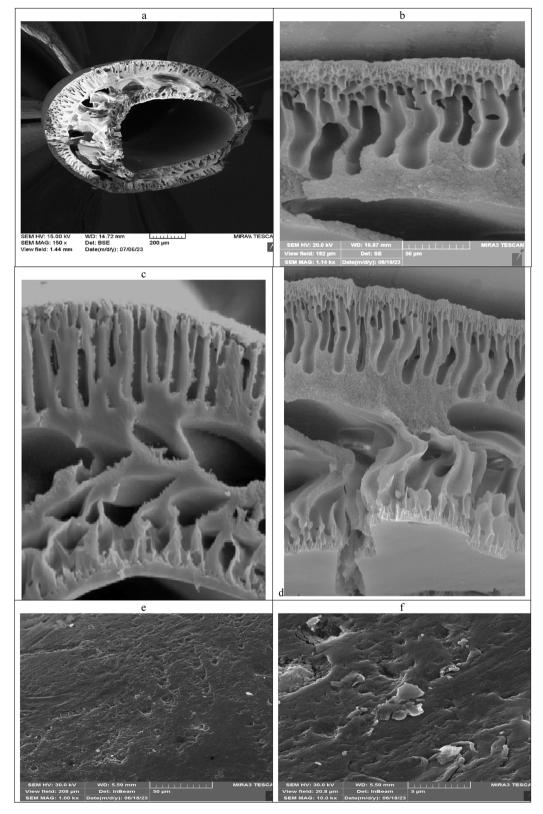
Fig. 3 FESEM image of PAN/GO-Tyr (a), cross-sectional images (b) and (d), cross section of PAN/GO hollow fiber (c) and surface images of PAN/ GO-Tyr HF (e) and (f).
