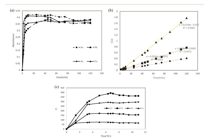
Fig. 7 (a) Adsorption kinetics of metal ions during 140 min at optimum conditions, (b) pseudo-second order fitting of kinetic data and (c) intraparticle diffusion models employing kinetic adsorption of metal ions using PAN/GO-Tyr HF.
