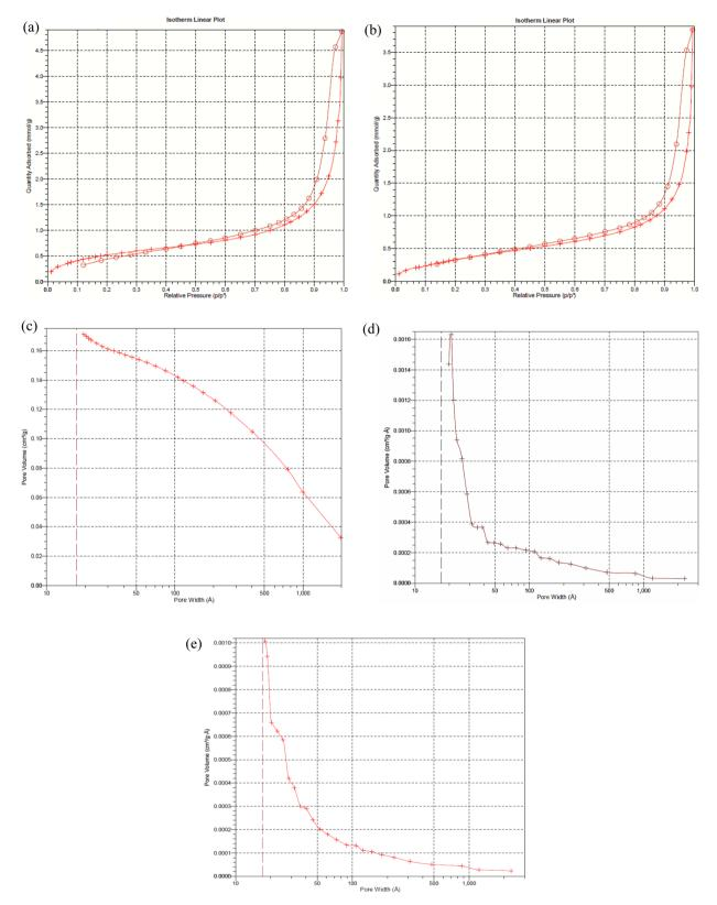
Fig. 4 BET  $N_2$  adsorption–desorption isotherms of PAN/GO-Tyr (a) and PAN/GO HF (b), BJH adsorption cumulative pore volume of PAN/GO-Tyr (c), BJH adsorption dV/dw pore volume of PAN/GO-Tyr (d) and BJH adsorption dV/dw pore volume of PAN/GO HF (e).
