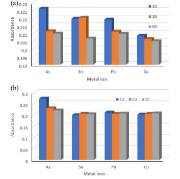
Fig. 6 Effect of phosphate ion (a) and carbonate ion (b) on the extraction of metal ions using PAN/GO-Tyr HF.
