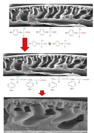
**Scheme 1** Proposed mechanism for the modification of PAN/GO HF using tyrosine.
