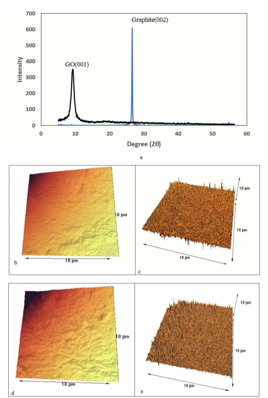
Fig. 2 (a) XRD spectra of pure graphite (black line) and GO (blue line), (b) AFFM 2D image and (c) 3D image of PAN/GO HF and (d) 2D AFM image and (e) 3D image of PAN/GO-Tyr HF.
