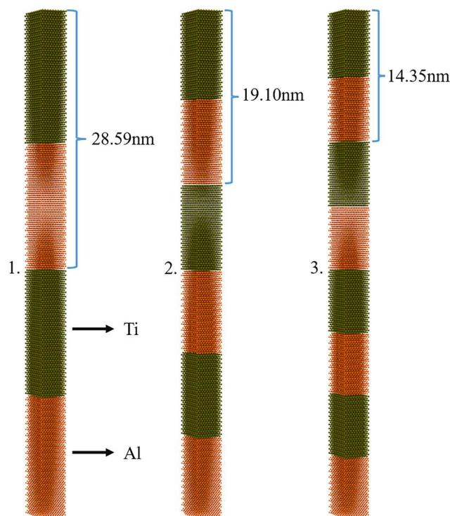
Fig. 1 Schematic diagram of modelling of Al/Ti layered nanosystems: (1) (Al/Ti)<sub>II</sub> layered nanosystem, (2) (Al/Ti)<sub>III</sub> layered nanosystem, (3) (Al/Ti)<sub>IV</sub> layered nanosystem; the orange particles are Al atoms and the green particles are Ti atoms.
