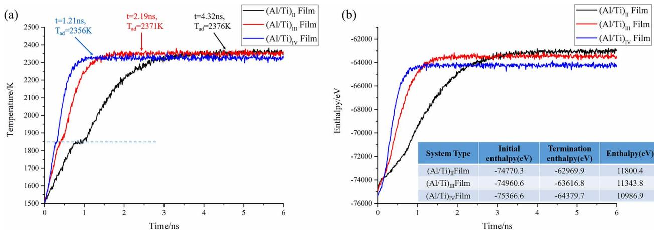
Fig. 4 (a) Variation of reaction temperature with simulation time for three modulation cycle (Al/Ti)<sub>II</sub>, (Al/Ti)<sub>III</sub> and (Al/Ti)<sub>IV</sub> thin film systems at an initial temperature of 1500 K. (b) Variation of reaction enthalpy with simulation time for (Al/Ti)<sub>II</sub>, (Al/Ti)<sub>III</sub> and (Al/Ti)<sub>IV</sub> thin film systems.
