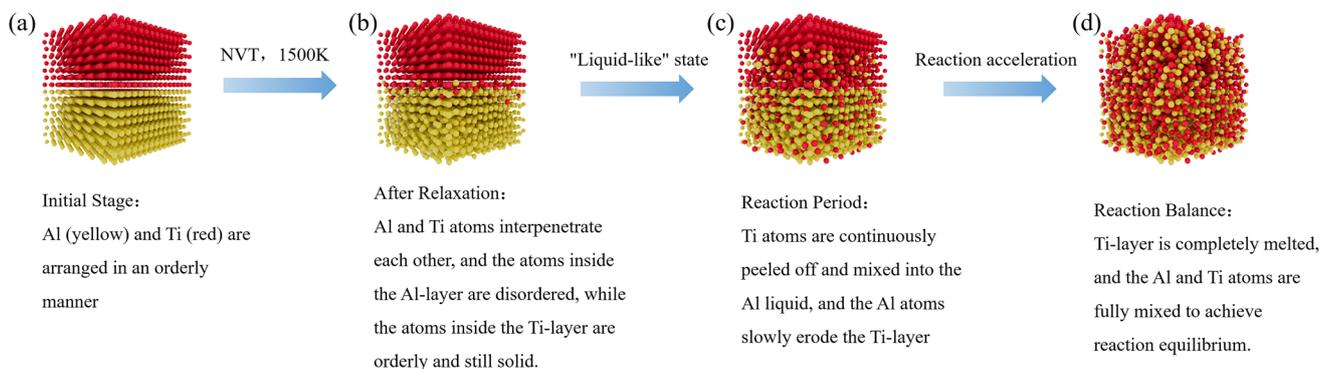
Fig. 8 Mechanism of simulated processes in the Al/Ti layer system (Al atoms: yellow, Ti atoms: red): (a) initial stage; (b) after relaxation; (c) reaction period; (d) reaction balance.
