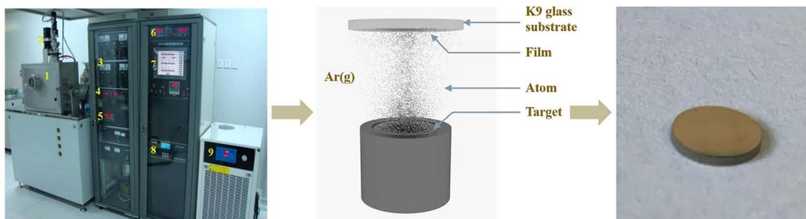
Fig. 2 Magnetron sputtering flow and sample diagram.
