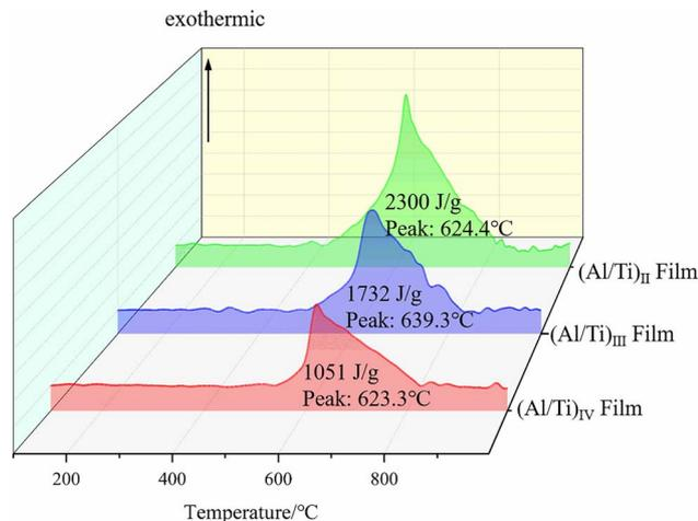
Fig. 9 DSC curves of Al/Ti nanoenergy-containing films with three different modulation cycles ((Al/Ti)<sub>II</sub>, (Al/Ti)<sub>III</sub>, (Al/Ti)<sub>IV</sub>).
