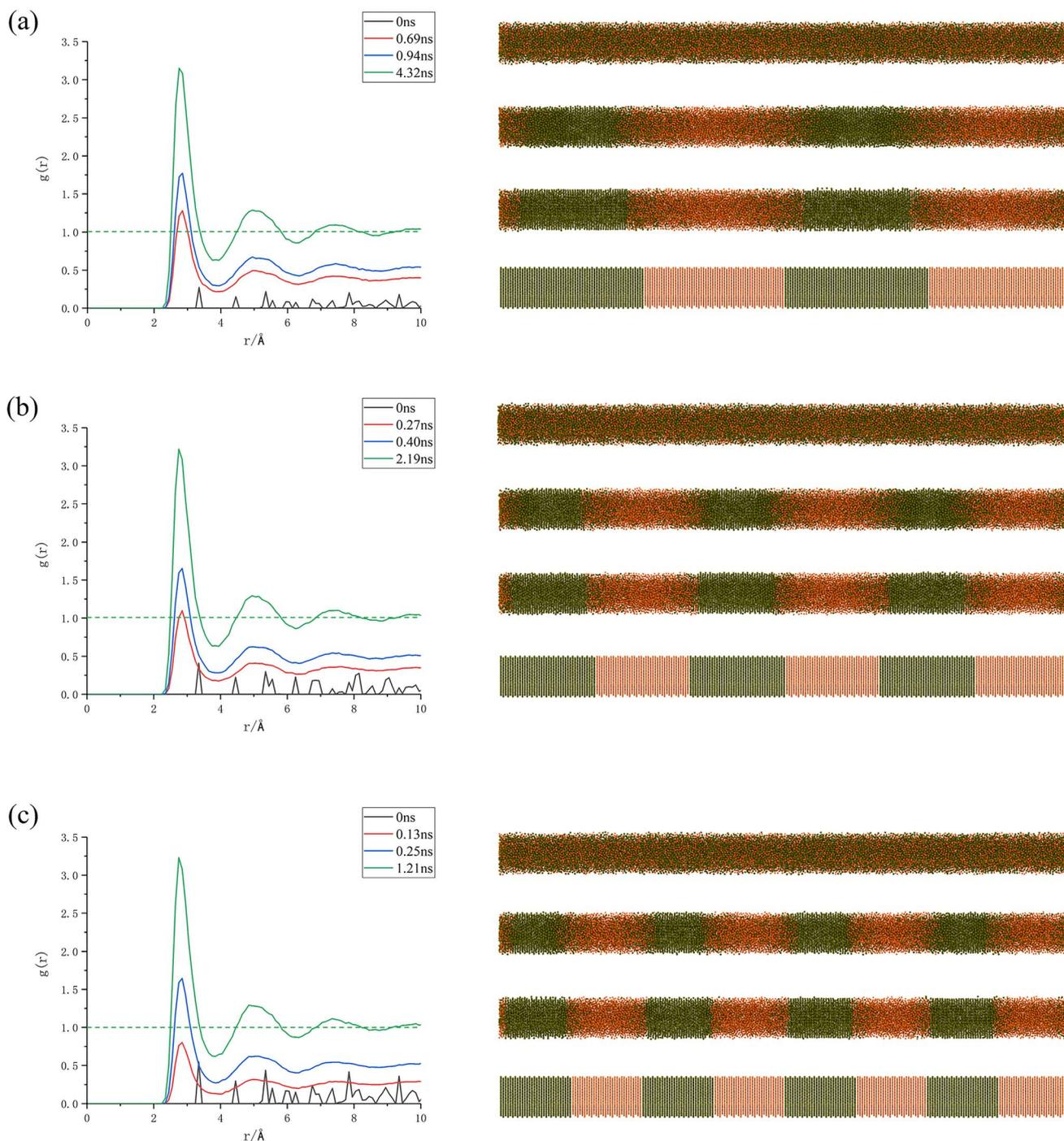
Fig. 5 (a)–(c) represent the correspondence between  $g_{\text{Al-Ti}}(r)$  and atomic migration snapshots for different modulation cycles of Al/Ti, respectively.
