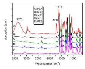
Fig. 3 FTIR spectra of different PEA/PES blends.
