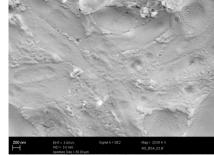
Fig. 9 SEM micrographs for the M2 (left) and PES18 (right) membranes with the surface covered with BSA (X = 20 K).
