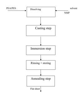
Scheme 1 Process flow sheet for membrane preparation.
