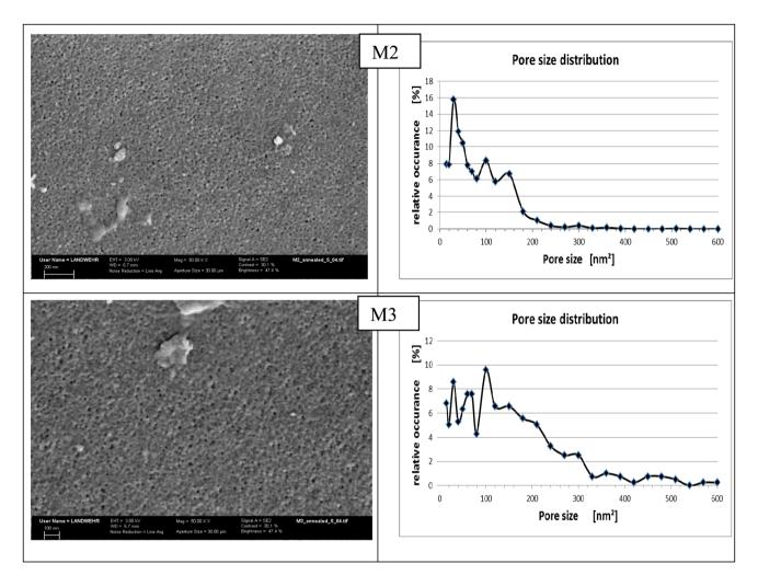
Fig. 5 SEM images and pore size distribution for M2 and M3 membranes annealed at 100 °C ( $X = 50\,000$ ).
