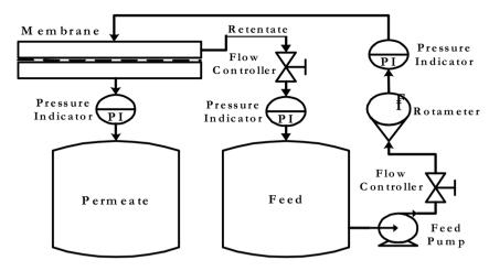
Fig. 2 Instrument set-up for membrane testing.
