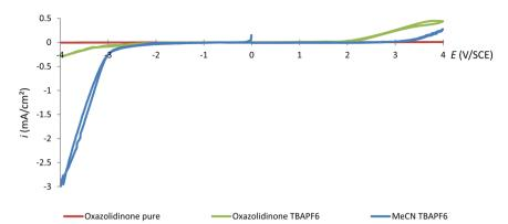
Fig. 1 CVs of the oxazolidinone vs. acetonitrile, pure or containing 0.1 M TBAPF<sub>6</sub> (under Ar, WE: Pt:  $\emptyset = 1$  mm,  $\nu = 10$  mV s<sup>-1</sup>).
