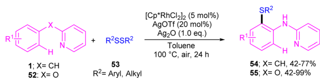
Scheme 32 Rh(III)-catalyzed annulation of N -aryl-2-pyridinamines with disulfides.
