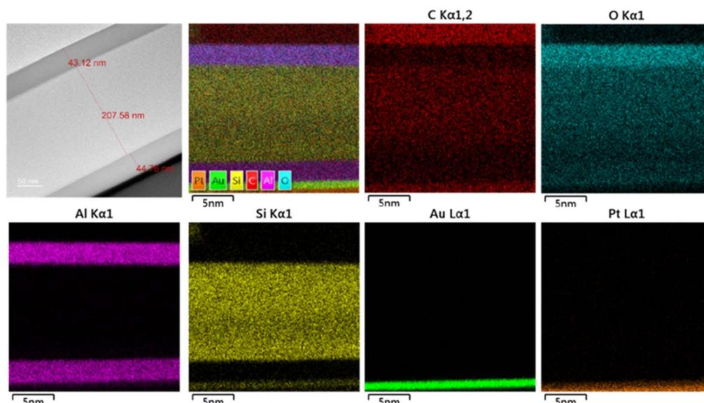
Fig. 7 HRTEM cross-sectional image and EDS mapping of the Al<sub>2</sub>O<sub>3</sub>/OPSZ/Al<sub>2</sub>O<sub>3</sub> three-layer barrier film.
