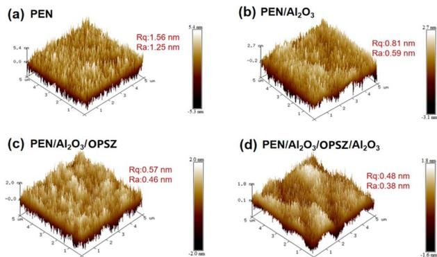
Fig. 8 AFM images and surface roughness values of (a) PEN, (b) PEN/ $\text{Al}_2\text{O}_3$ , (c) PEN/ $\text{Al}_2\text{O}_3$ /OPSZ, and (d) PEN/ $\text{Al}_2\text{O}_3$ /OPSZ/ $\text{Al}_2\text{O}_3$ .
