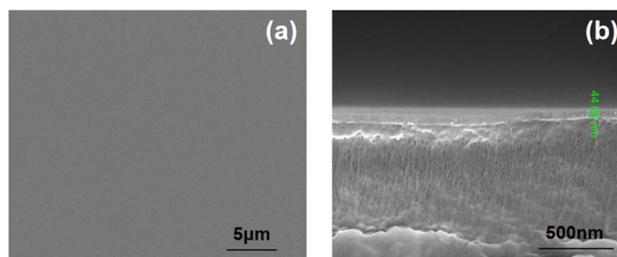
Fig. 2 Surface (a) and cross-sectional (b) SEM images of the  $\text{Al}_2\text{O}_3$  film.
