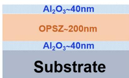
Fig. 1 Schematic of the multilayer barrier film.
