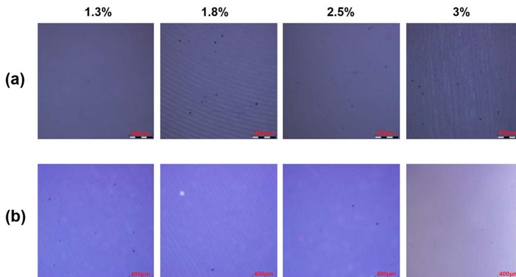
Fig. 12 Microscopic images for  $\text{Al}_2\text{O}_3$  single-layer (a) and  $\text{Al}_2\text{O}_3/\text{OPSZ}/\text{Al}_2\text{O}_3$  multilayer (b) films after 1.3%, 1.8%, 2.5%, and 3% bending strain.
