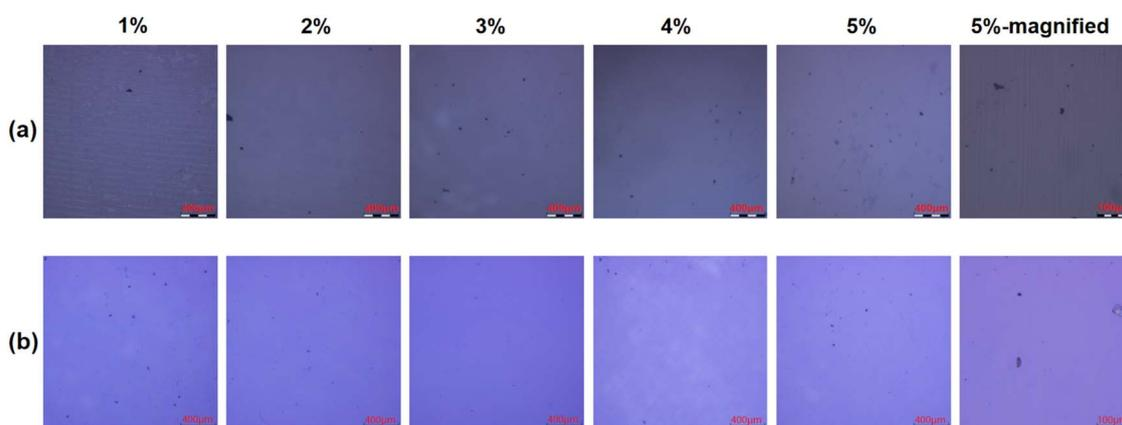
Fig. 11 Microscopic images for  $\text{Al}_2\text{O}_3$  single-layer (a) and  $\text{Al}_2\text{O}_3/\text{OPSZ}/\text{Al}_2\text{O}_3$  multilayer (b) films after 1%, 2%, 3%, 4%, and 5% tensile strain.
