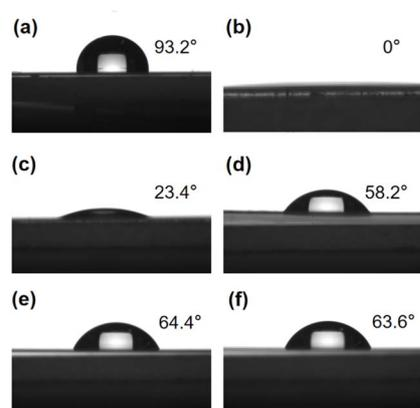
Fig. 4 Images of contact angle before (a) and after (b)–(f) plasma treatment: 0 day (b), 1 day (c), 3 days (d), 5 days (e), and 7 days (f) storage time after treatment.
