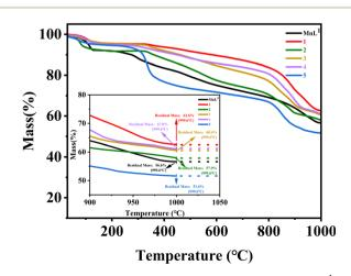
Fig. 2 Thermogravimetric analysis (TGA) curves of  $\mathrm{MnL}^1$  and compounds 1–5.
