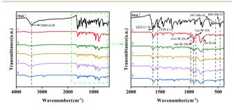
Fig. 1 Fourier transform infrared spectra of  $\mathsf{MnL}^1$  and compounds 1–5.
