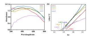
Fig. 4 (a) Solid-state UV/Vis absorption spectra of compounds 1-5; (b) calculated band gap compounds 1-5.
